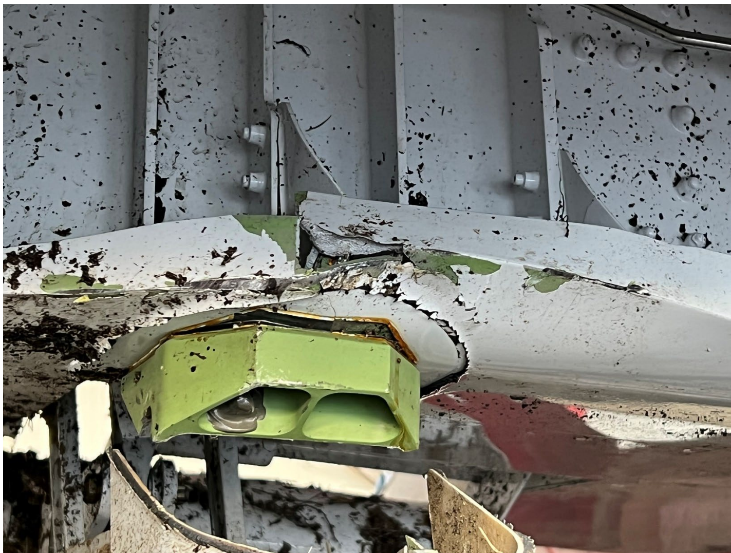
Photograph 8 - View of damage above left main landing gear. (Courtesy of HondaJet)
