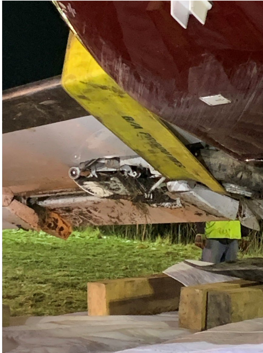
Photograph 4 - View of lower fuselage and wing damage. (Courtesy of FAA)
