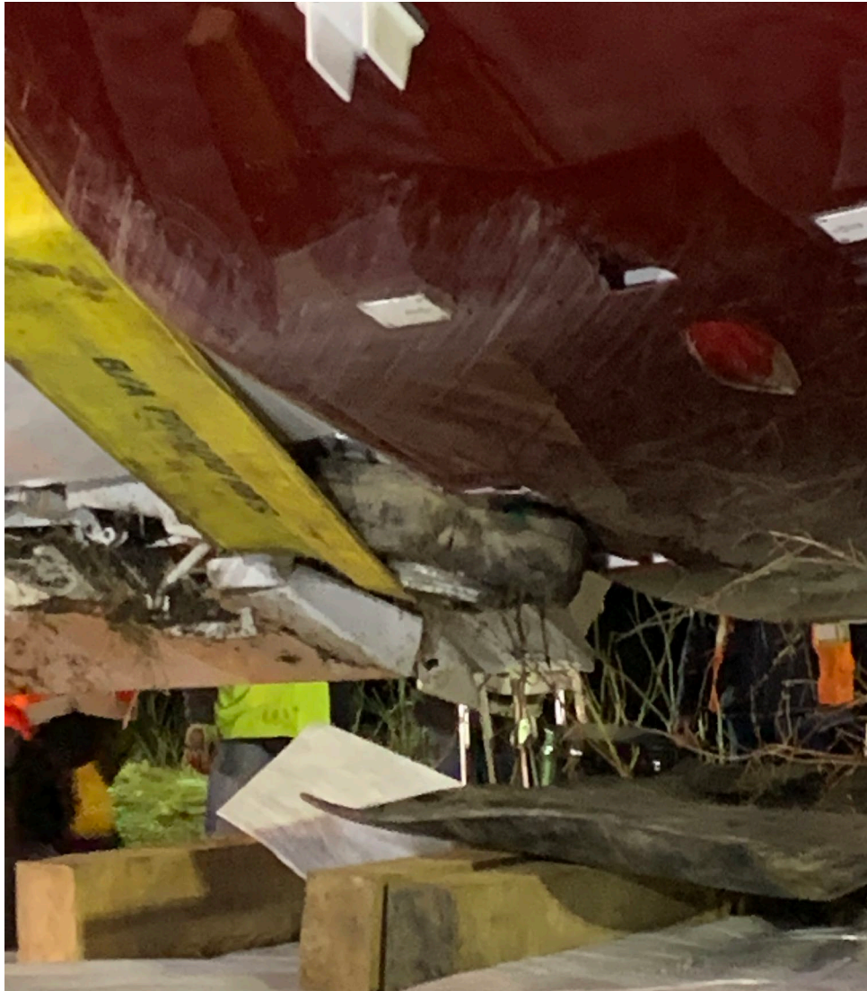
Photograph 6 - View of impact damage as viewed at recovery. (Courtesy of FAA)
