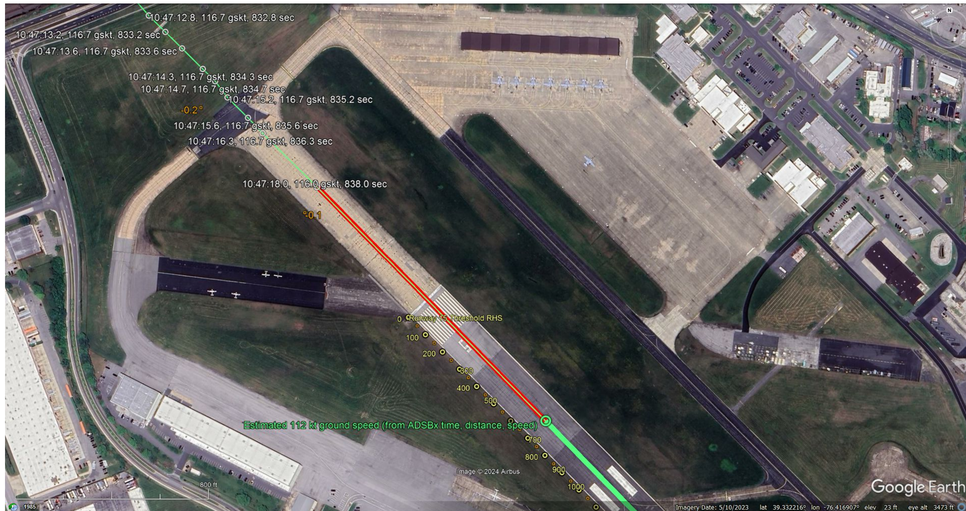
Figure A11.1: N22AU accident flight path reconstruction showing short final approach to 1,000 feet along MTN runway 15. N22AU direction of travel is upper left to lower right. Ground track reconstruction is based on Automatic Dependent Surveillance - Broadcast (ADS-B) data (white text), paraphrased CVR events (green text), Cessna Aircraft Recording System (ARes) parametric data (yellow events), airport surveillance camera video content, and runway witness mark evidence. Due north is toward the top of the page.
