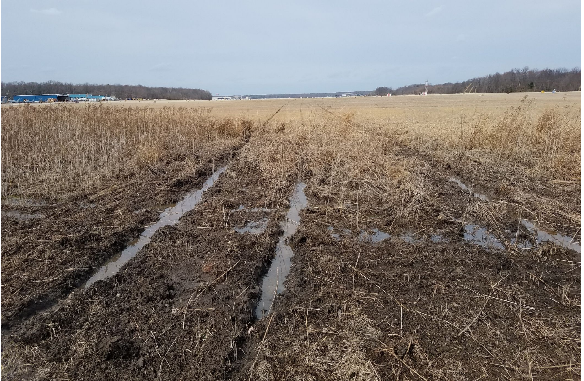
Figure A6.2: N22AU ground track evidence (view looking back toward the departure end of runway 15). Photograph provided to NTSB investigation by Maryland Department of Transportation, Maryland Aviation Administration.
