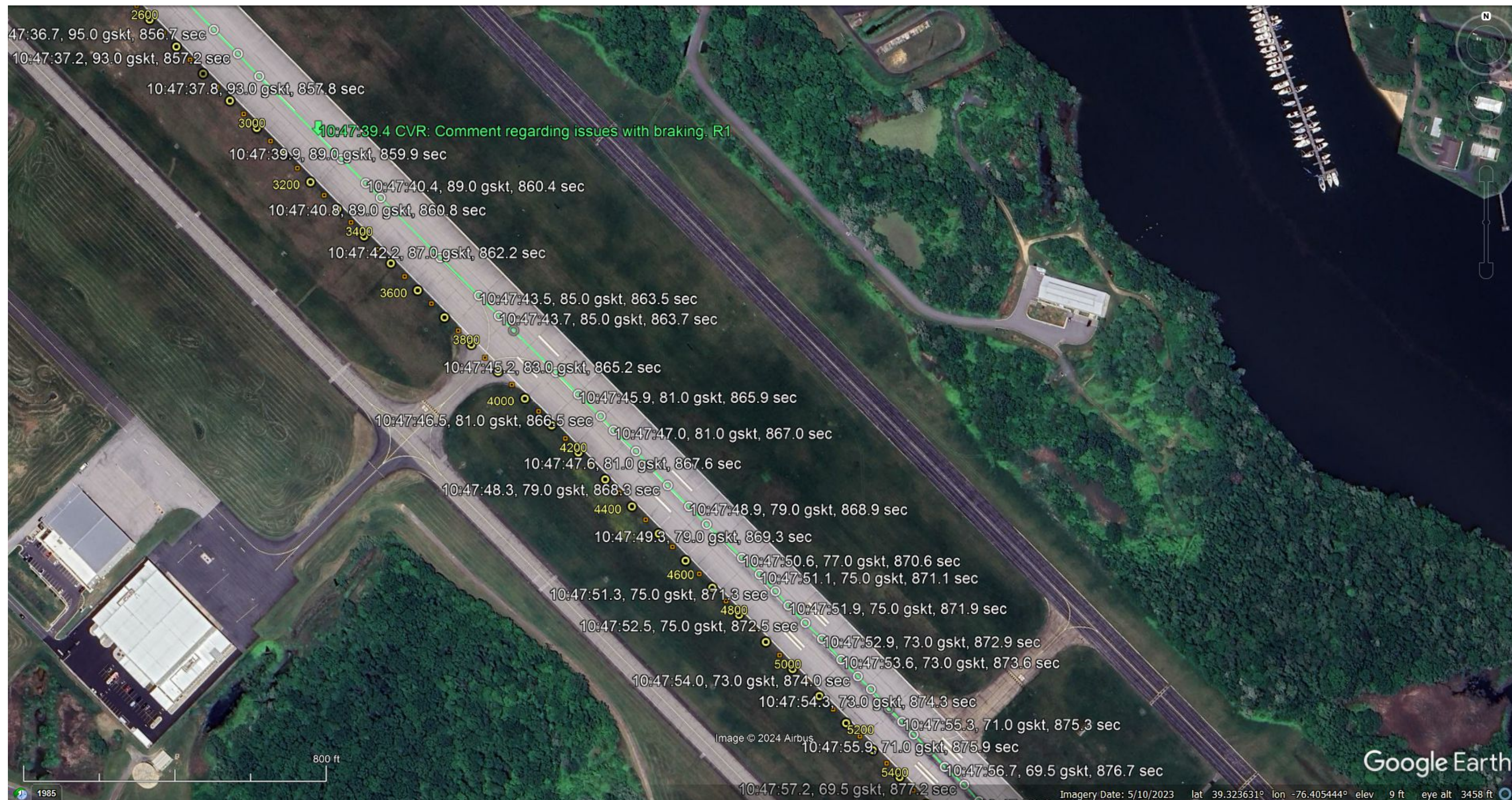
Figure A11.3: N22AU accident flight path reconstruction showing 3,000 to 5,000 feet along MTN runway 15. N22AU direction of travel is upper left to lower right. Ground track reconstruction is based on Automatic Dependent Surveillance - Broadcast (ADS-B) data (white text), paraphrased CVR events (green text), Cessna Aircraft Recording System (ARes) parametric data (yellow events), airport surveillance camera video content, and runway witness mark evidence. Due north is toward the top of the page.
