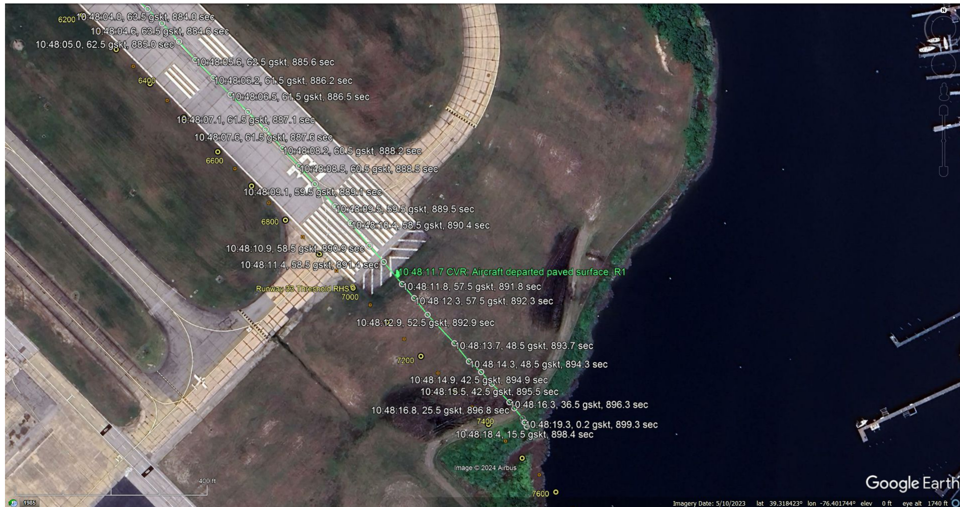
Figure A11.6: N22AU accident flight path reconstruction showing 6,500 to 7,500 feet along MTN runway 15. N22AU direction of travel is upper left to lower right. Ground track reconstruction is based on Automatic Dependent Surveillance - Broadcast (ADS-B) data (white text), paraphrased CVR events (green text), Cessna Aircraft Recording System (ARes) parametric data (yellow events), airport surveillance camera video content, and runway witness mark evidence. Due north is toward the top of the page.
