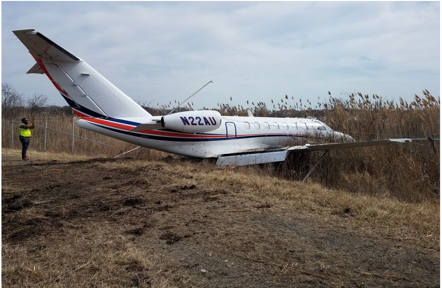
Figure A6.4: N22AU in position of final rest (view looking toward the aircraft and the airport perimeter fence beyond the departure end of runway 15). Photograph provided to NTSB investigation by Maryland Department of Transportation, Maryland Aviation Administration.
