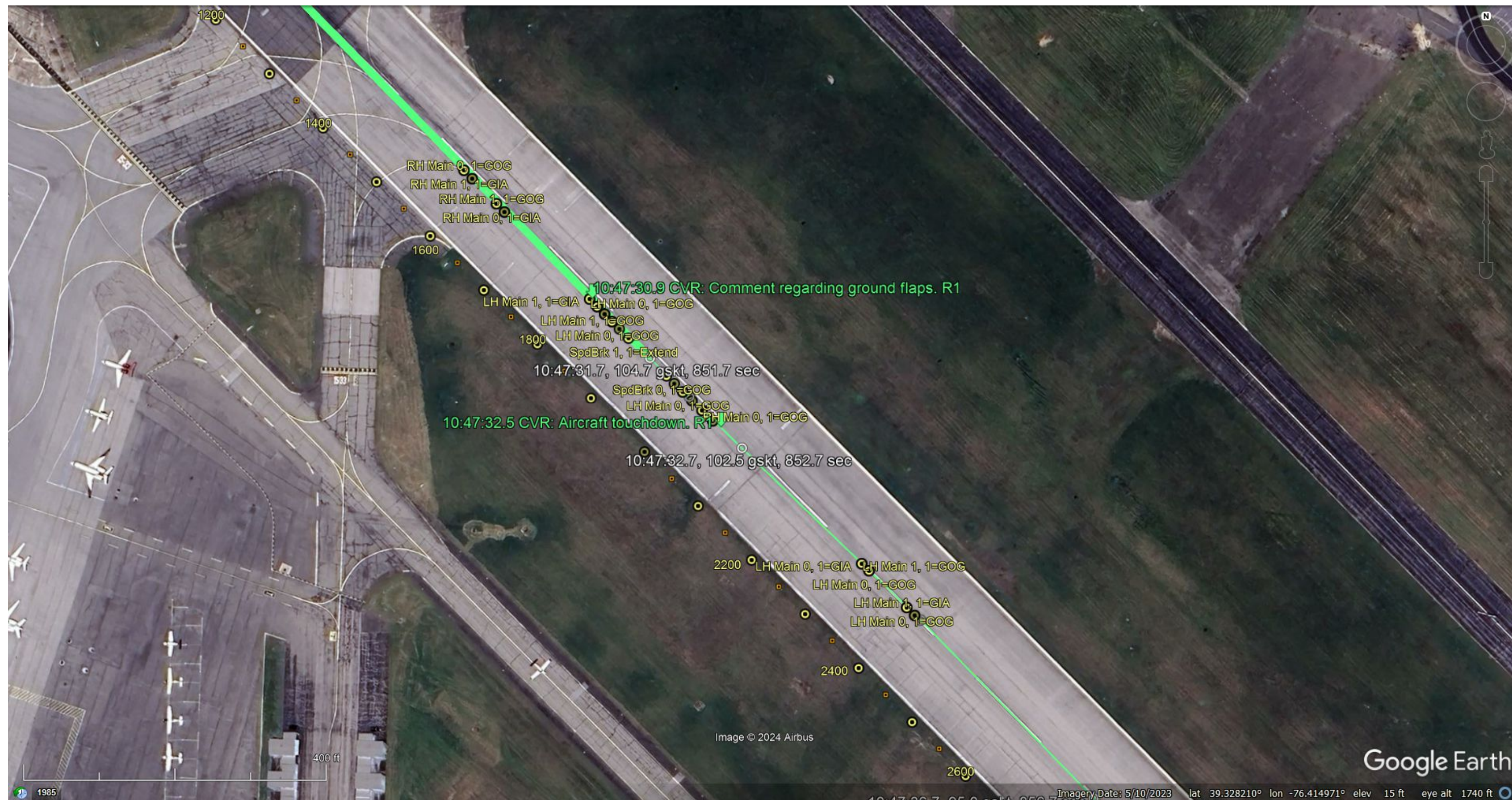
Figure A11.5: N22AU accident flight path reconstruction showing 1,500 to 2,500 feet along MTN runway 15. N22AU direction of travel is upper left to lower right. Ground track reconstruction is based on Automatic Dependent Surveillance - Broadcast (ADS-B) data (white text), paraphrased CVR events (green text), Cessna Aircraft Recording System (ARes) parametric data (yellow events), airport surveillance camera video content, and runway witness mark evidence. Main landing gear touchdown and speed brake nomenclature: LH=left hand, RH=right hand, GOG=gear on ground, GIA=gear in air, SpdBrk=upper and lower wing speed brakes. Due north is toward the top of the page.
