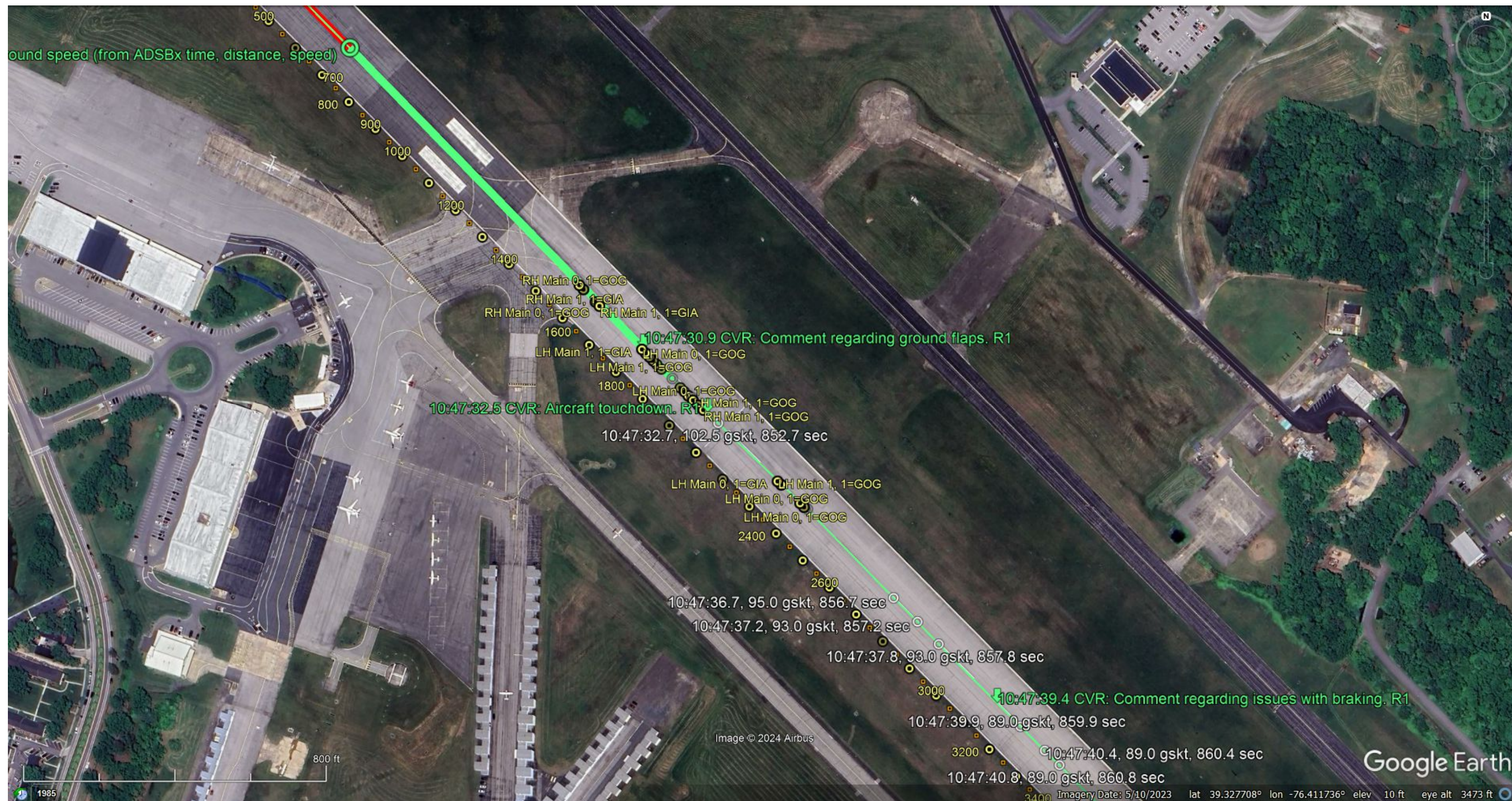
Figure A11.2: N22AU accident flight path reconstruction showing 1,000 to 3,000 feet along MTN runway 15. N22AU direction of travel is upper left to lower right. Ground track reconstruction is based on Automatic Dependent Surveillance - Broadcast (ADS-B) data (white text), paraphrased CVR events (green text), Cessna Aircraft Recording System (ARes) parametric data (yellow events), airport surveillance camera video content, and runway witness mark evidence. Main landing gear touchdown and speed brake nomenclature: LH=left hand, RH=right hand, GOG=gear on ground, GIA=gear in air, SpdBrk=upper and lower wing speed brakes. Due north is toward the top of the page.
