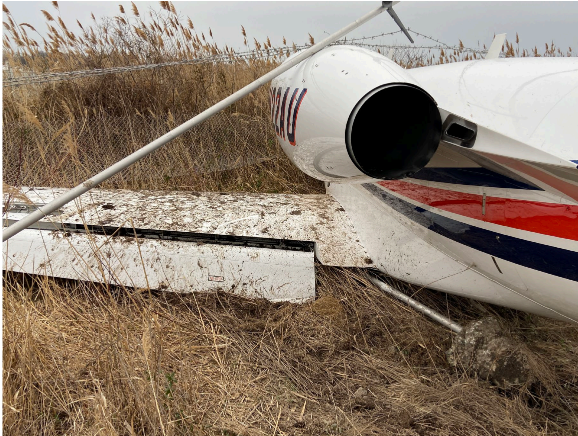
Photograph 4 - View of left wing flap damage. (Courtesy of MTN Airport)
