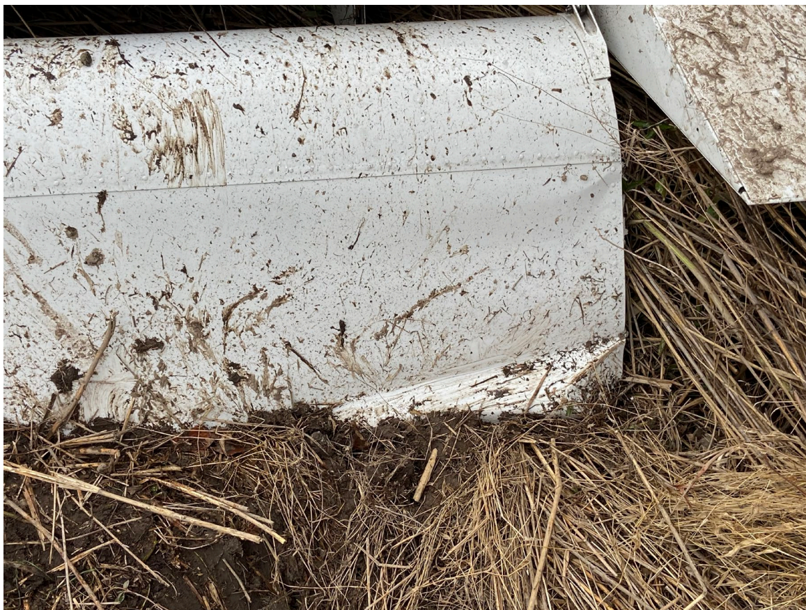
Photograph 5 - Closeup view of left flap damage. (Courtesy of MTN Airport)
