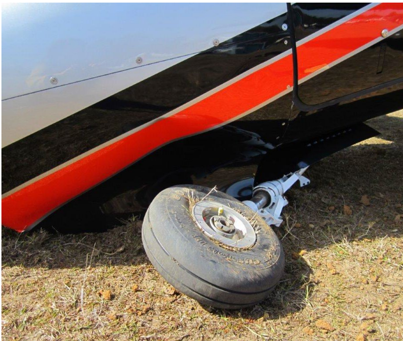
Photograph 2 - View of Nose Landing Gear Wheel (Right Side Facing UP, Courtesy FAA)
