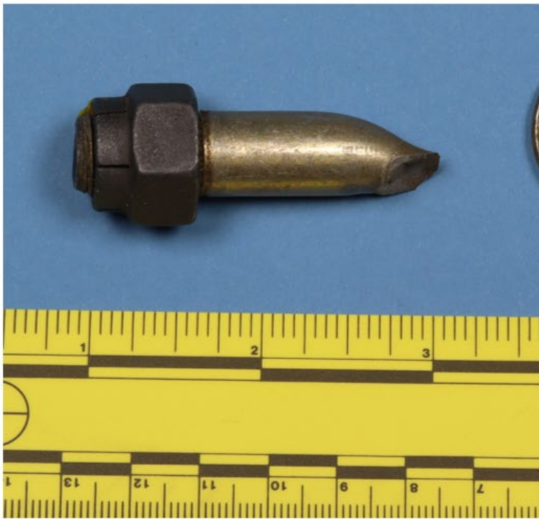
Photograph 6 - Fractured Trunnion Bolt (left) and Fitting (Right)
