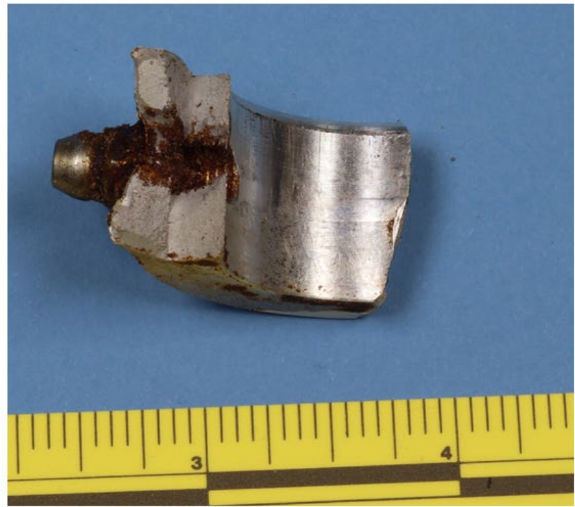
Photograph 6 - Fractured Trunnion Bolt (left) and Fitting (Right)
