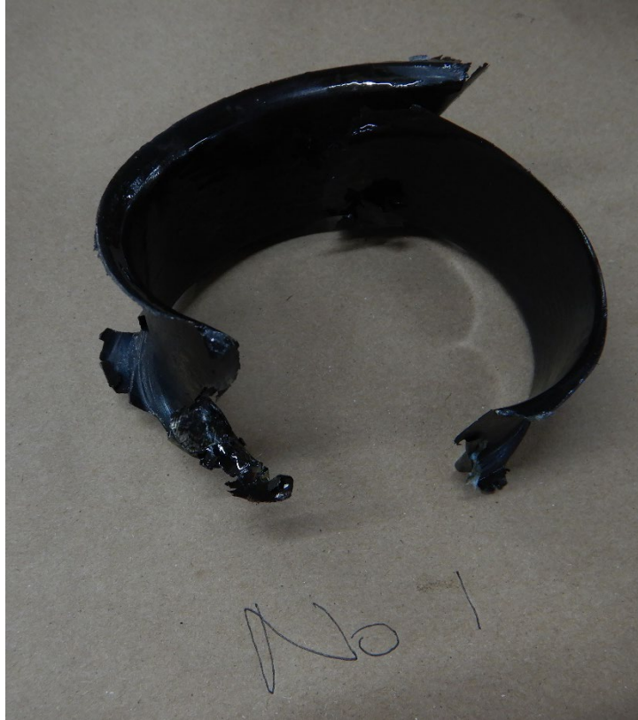
Photo 13 - View of removed fused bearing from cylinder No. 1.
