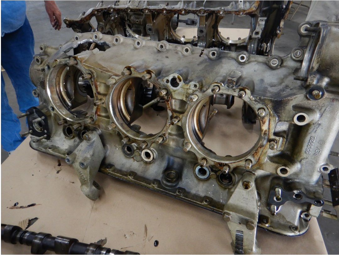
Photo 7 - View of left side of split crank case showing hole above cylinder No. 6.
