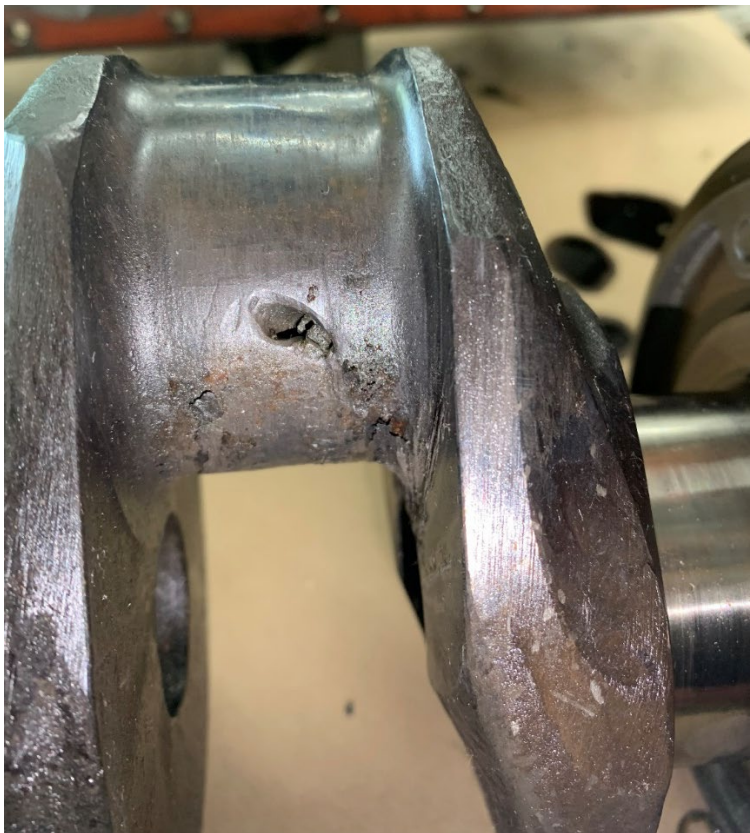
Photo 18 - View of portions of the No. 6 connecting rod bearing fused to the crankshaft journal.
