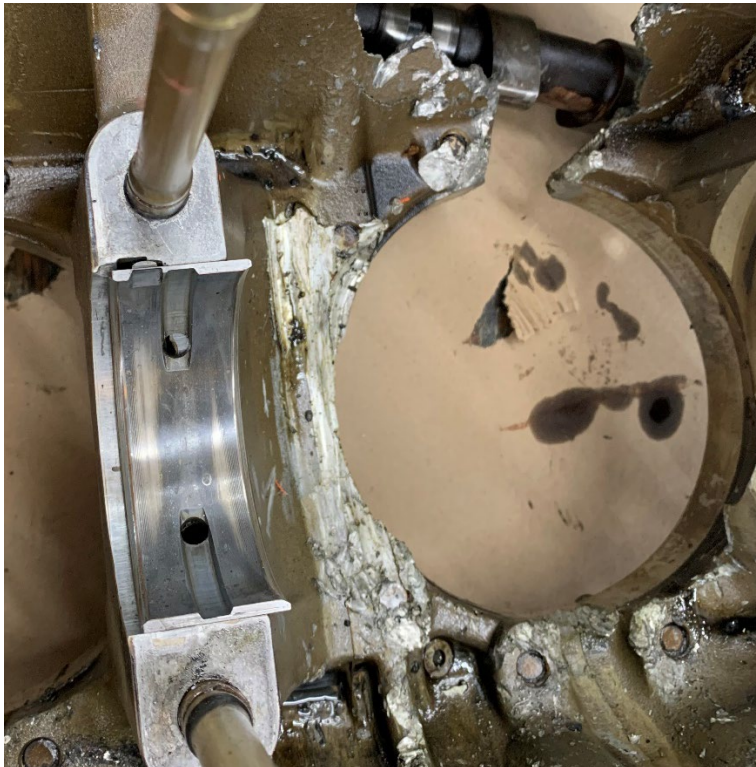
Photo 16 - View of damaged bearing and No. 3 main journal with damage on left crankcase.
