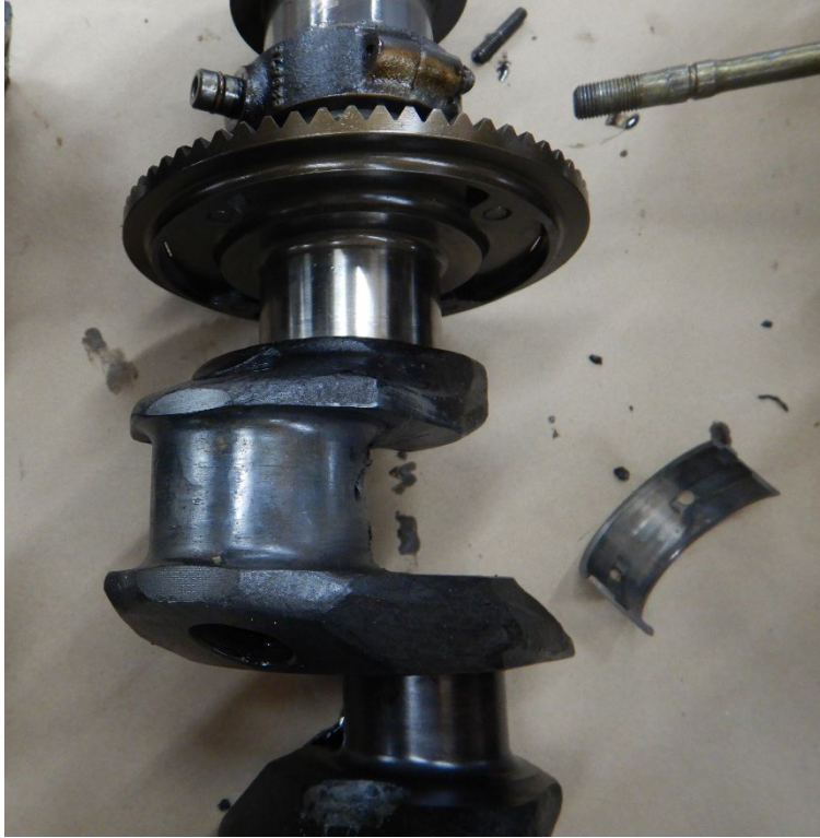
Photo 11 - Close-up view of burnt connecting rod journal.
