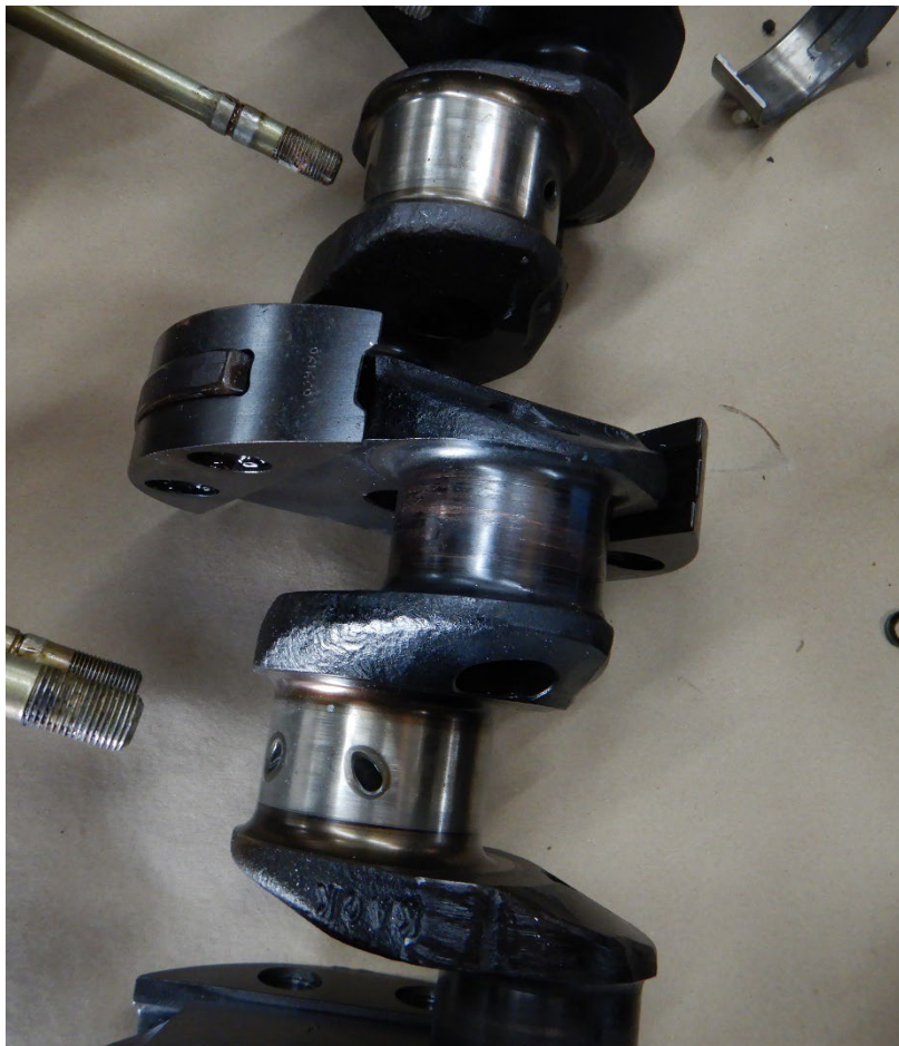
Photo 10 - Close-up view of burnt connecting rod journal.
