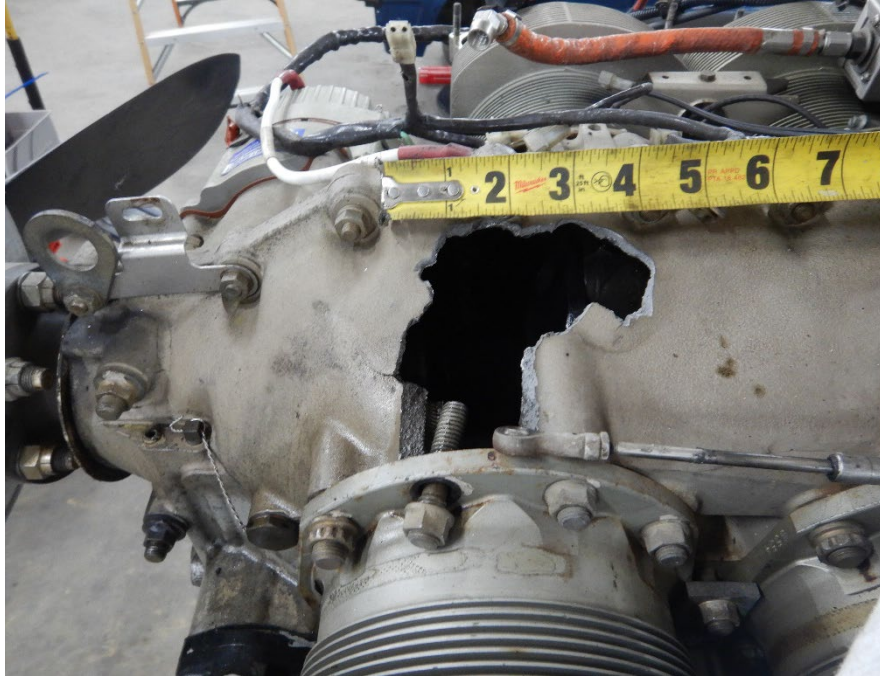
Photo 2 - Close-up view of crankcase hole.
