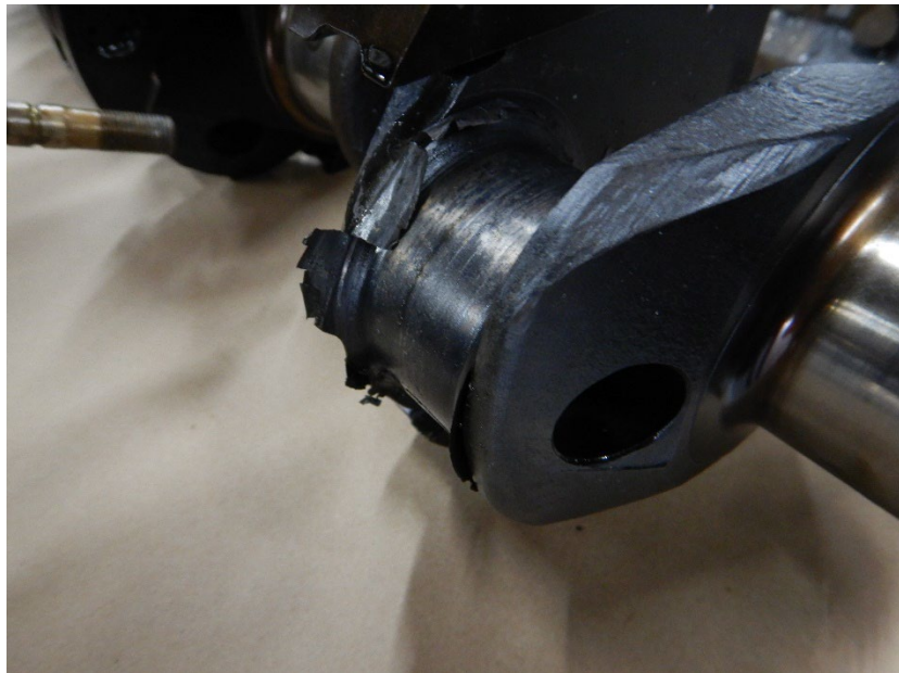
Photo 12 - View of spalling of fused bearing on cylinder No. 1.
