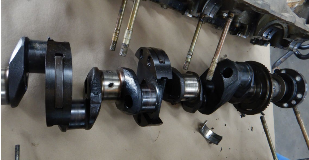
Photo 9 - View of crankshaft with burnt connecting rod journals.
