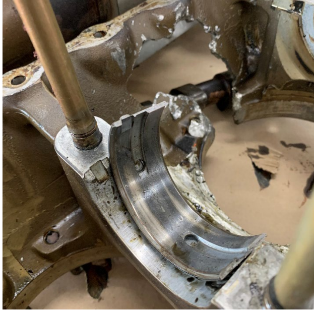
Photo 17 - Close-up view of bearing and No. 3 main journal damage on left crankcase
