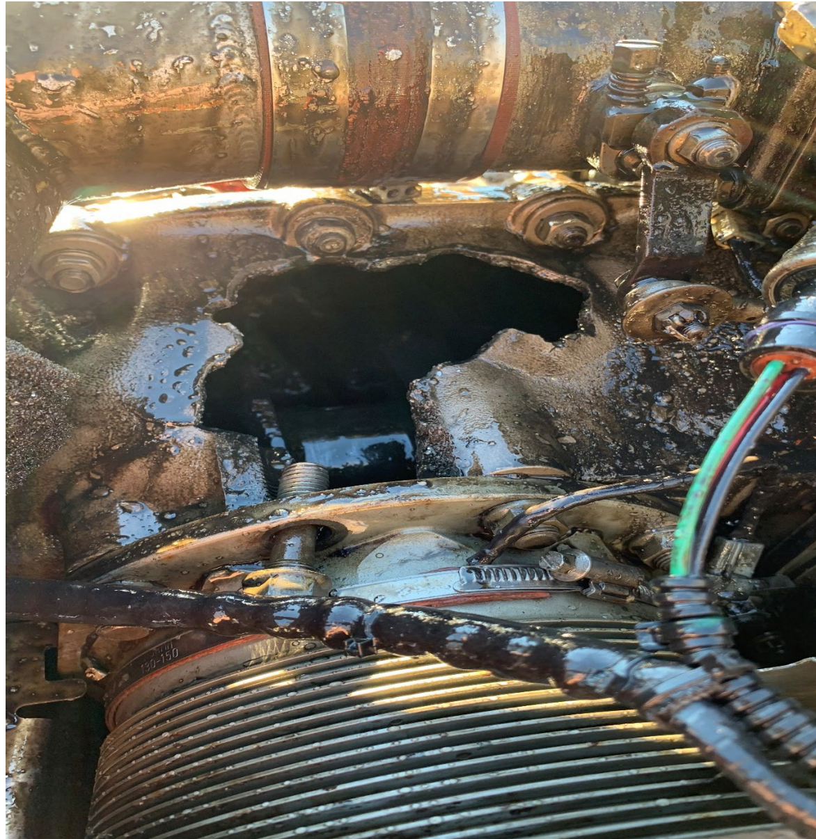
Photo 2 – View of damage to crankcase at cylinder No. 6 (Photo Courtesy of FAA)
