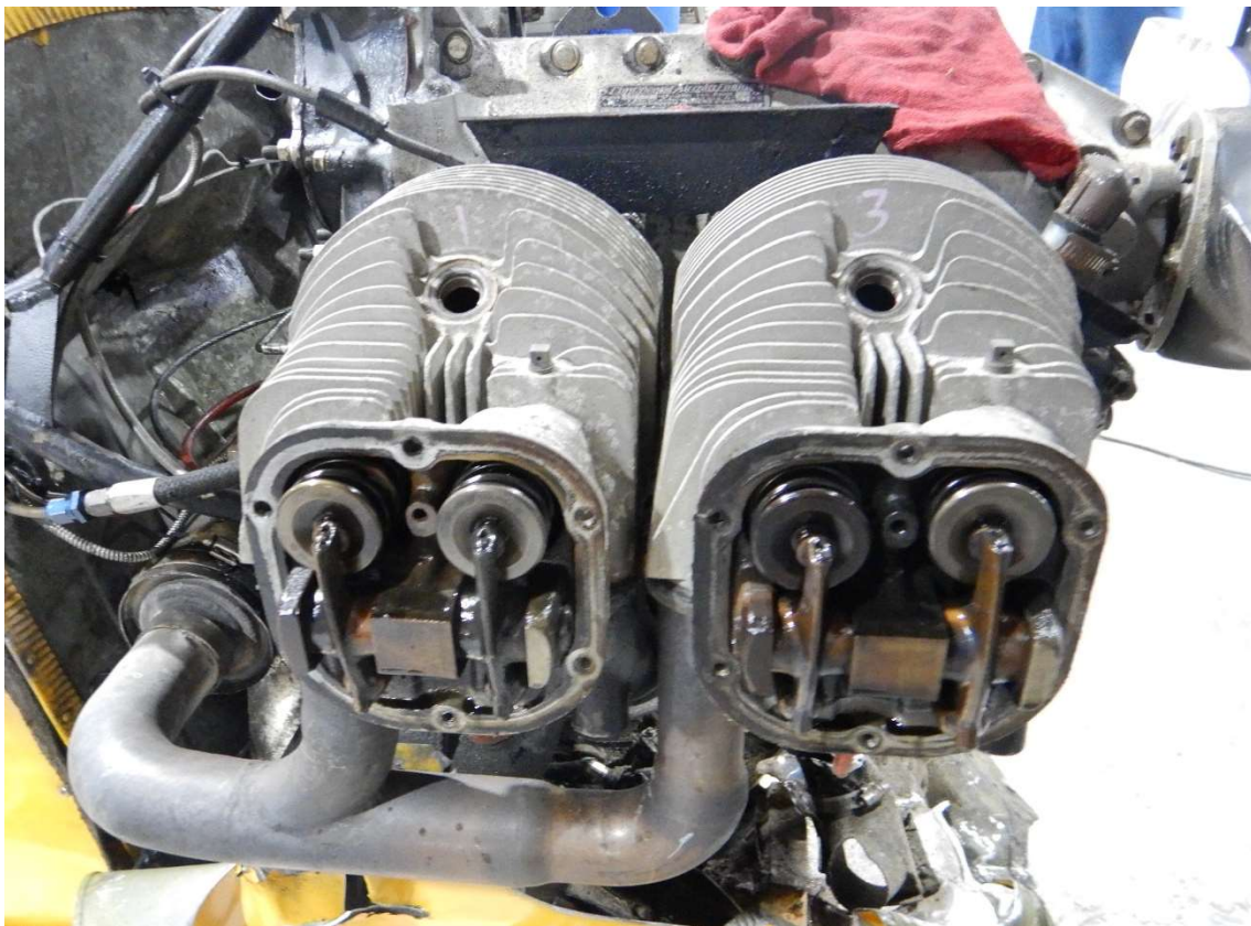
Photo 7 - Cylinder Nos. 1 and 3 with spark plugs and rocker covers removed
