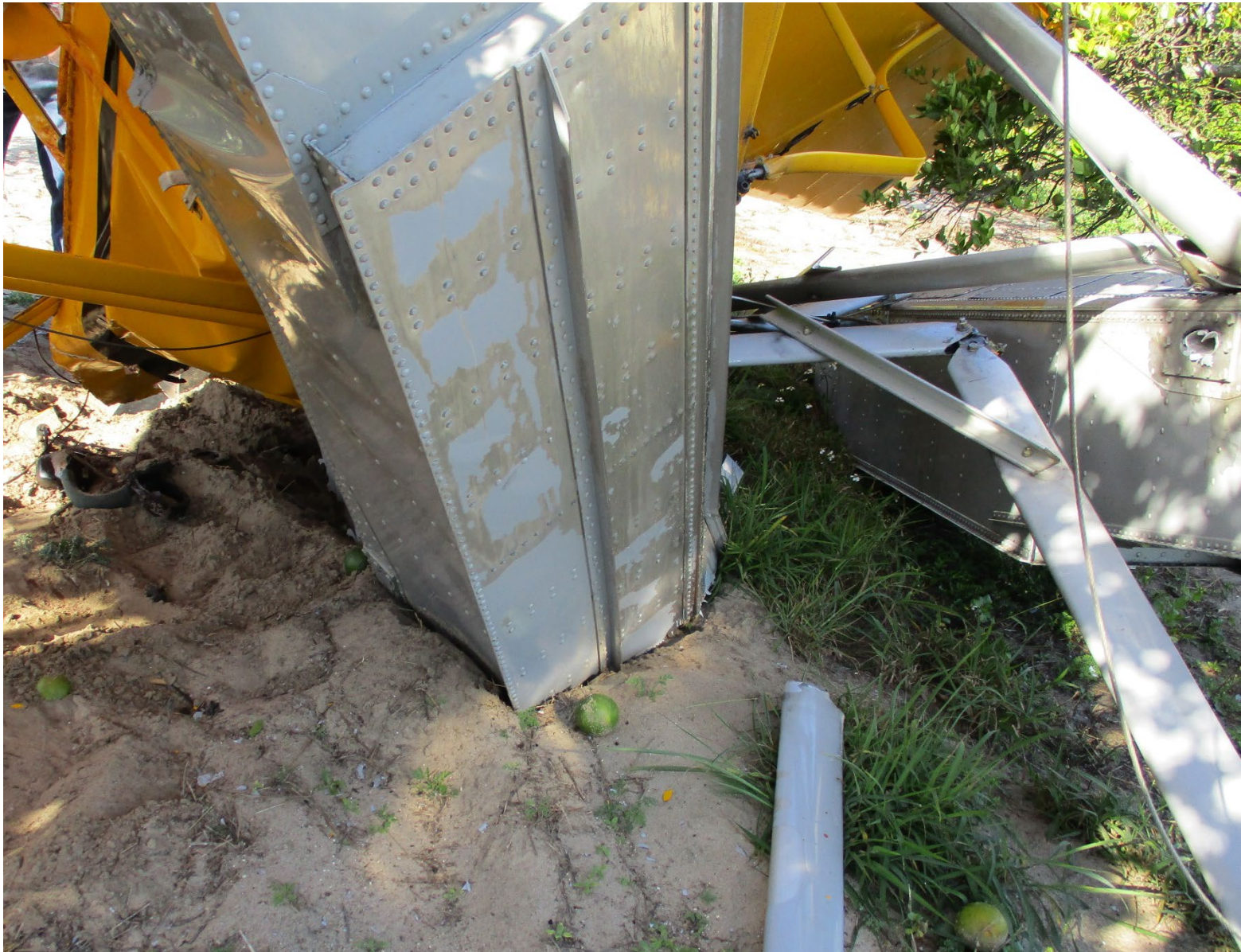
Photo 5 – Close-up View of Left Float Imbedded in Sand (Photo Courtesy of FAA)
