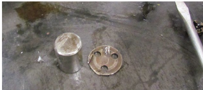
Figure 5 Counterweight missing roller, washer, and circlip. On the right, a free roller and washer found in the crankcase.
