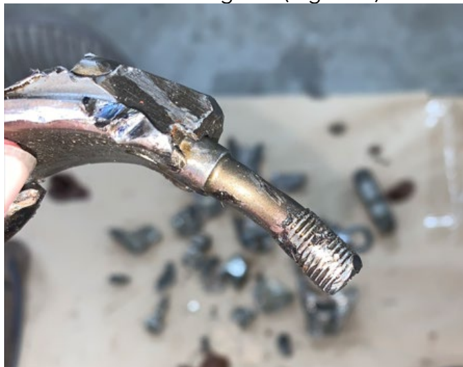
Figure 3 Connecting rod with damaged threads and missing nut.
