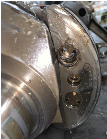
Figure 5 Counterweight missing roller, washer, and circlip. On the right, a free roller and washer found in the crankcase.
