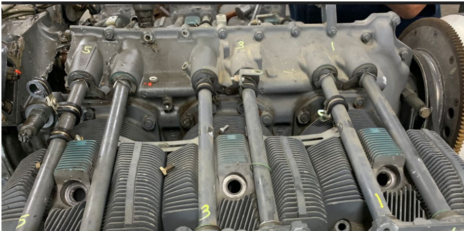
Figure 2 Overall view of top of engine showing hole over No. 5
