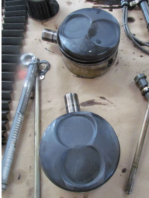
Figure 4 Piston crowns with features consistent with detonation.
