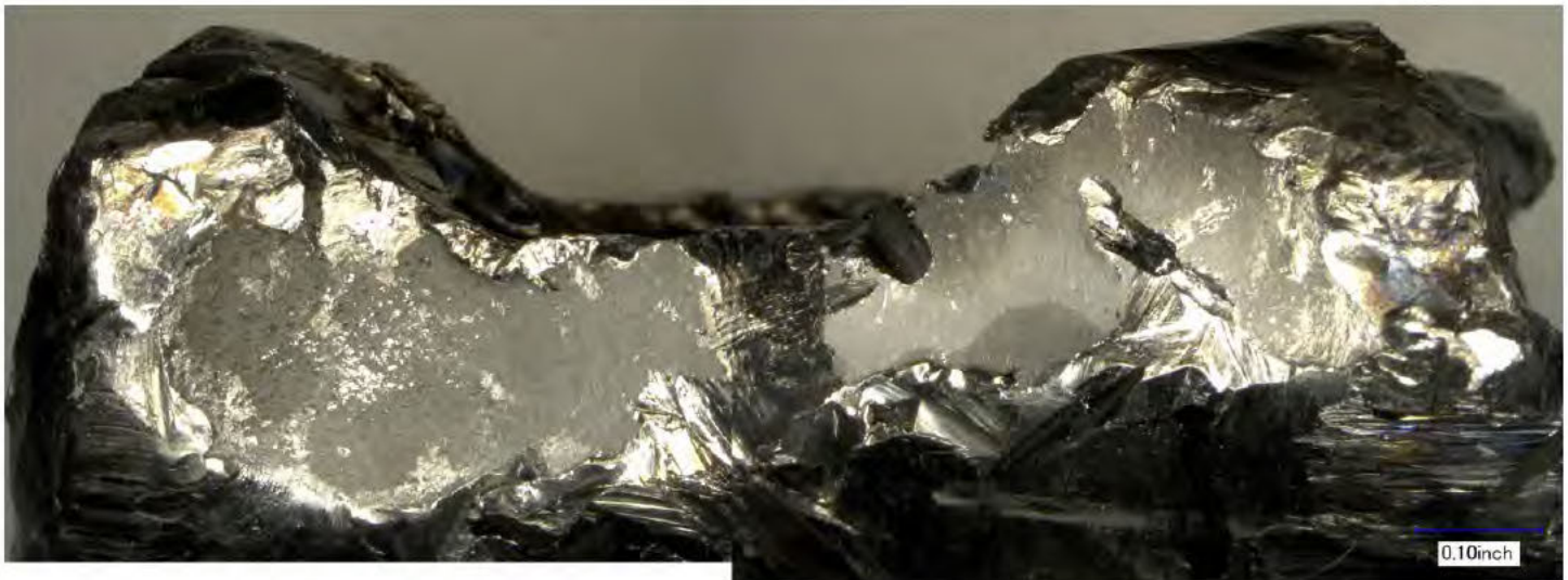
Figure 22. Image of fracture surface of Piece P. Provides no useful failure information.
