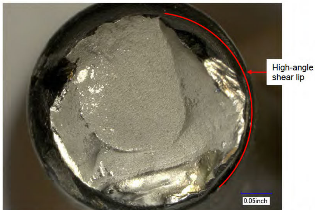
Figure 11. Image of the unthreaded end of Piece H showing cup-and-cone fracture surface and very high-angle shear lip.
