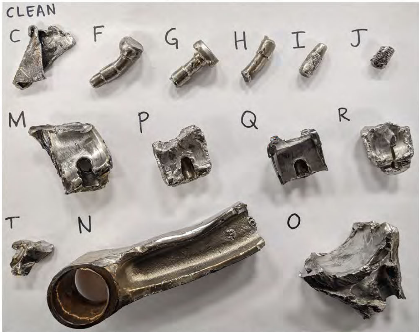
Figure 8. Image of all 13 remnant pieces judged to have fracture surfaces with potentially salvageable (at least partially undamaged) fracture surfaces, labeled and cleaned.
