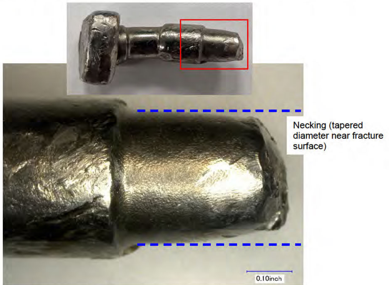
Figure 9. Image of Piece F showing necking.
