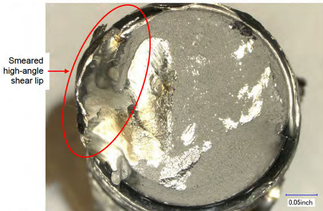
Figure 14. Image of fracture surface of Piece J showing a smeared shear lip and cup-and-cone fracture.
