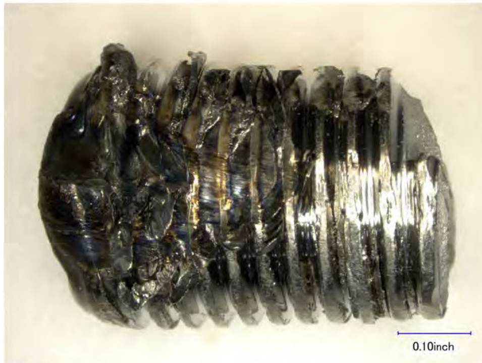
Figure 15. Image showing smashed threads of Piece J.
