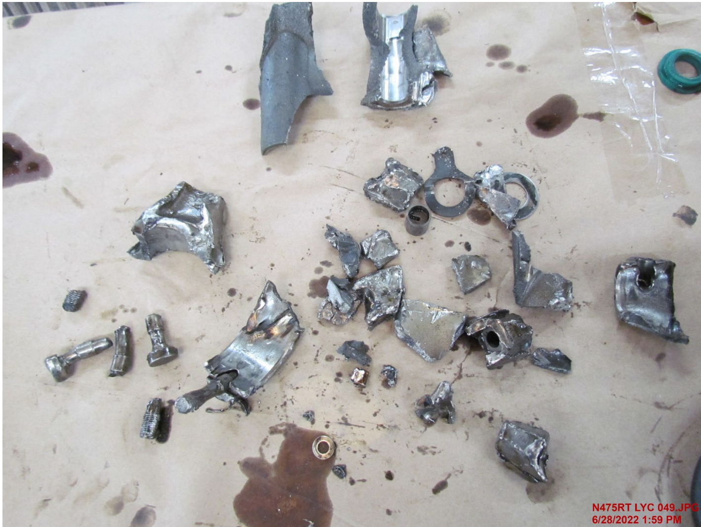
Photograph 6 - Fractured bearings, rods and rod bolts. (Courtesy of Lycoming)
