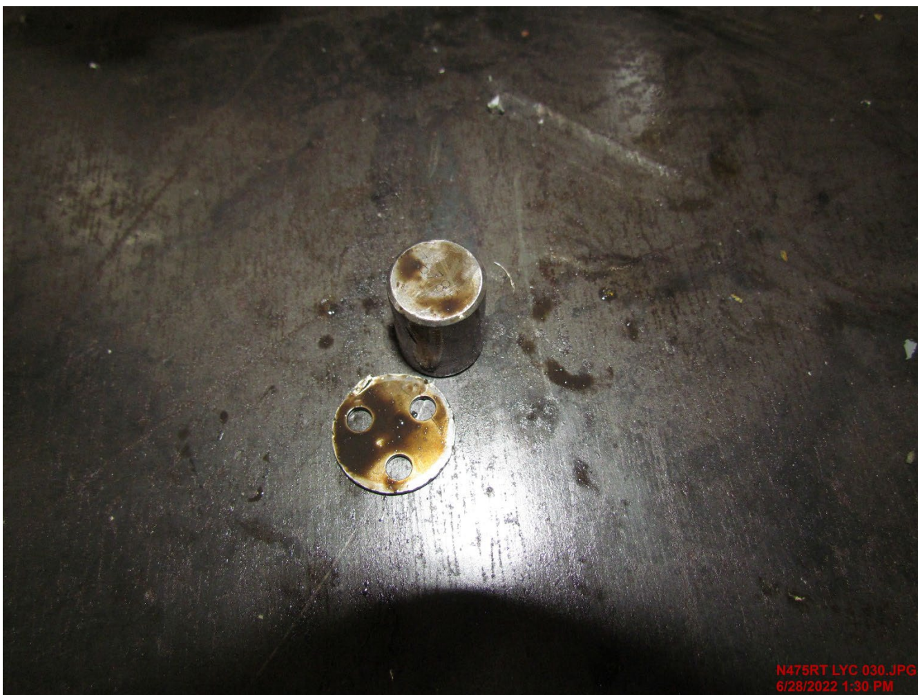
Photograph 4 - Counterweight roller and washer ejected. (Courtesy of Lycoming)
