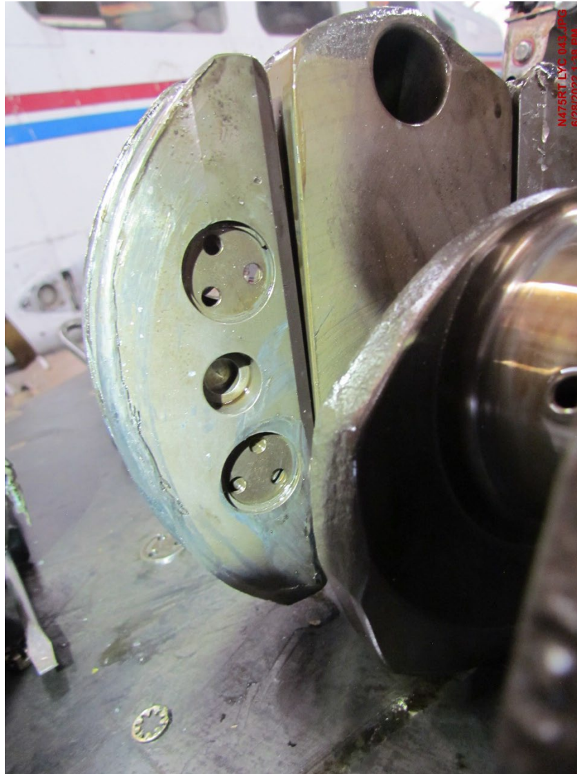
Photograph 5 - Counterweight, washer, and circlip. Note circlip with broken eyelets. (Courtesy of NTSB)
