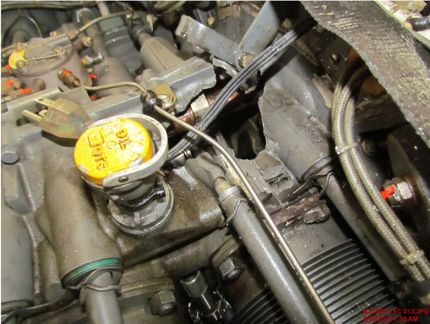
Photograph 2 - Closeup view of hole in engine case. (Courtesy of Lycoming)
