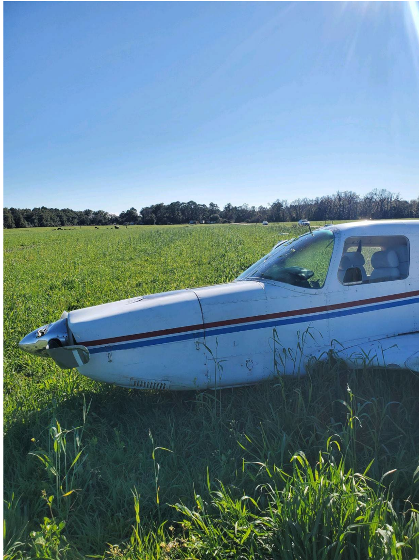
Photograph 3 - View of left front side of airplane showing damage. (Courtesy of FAA)
