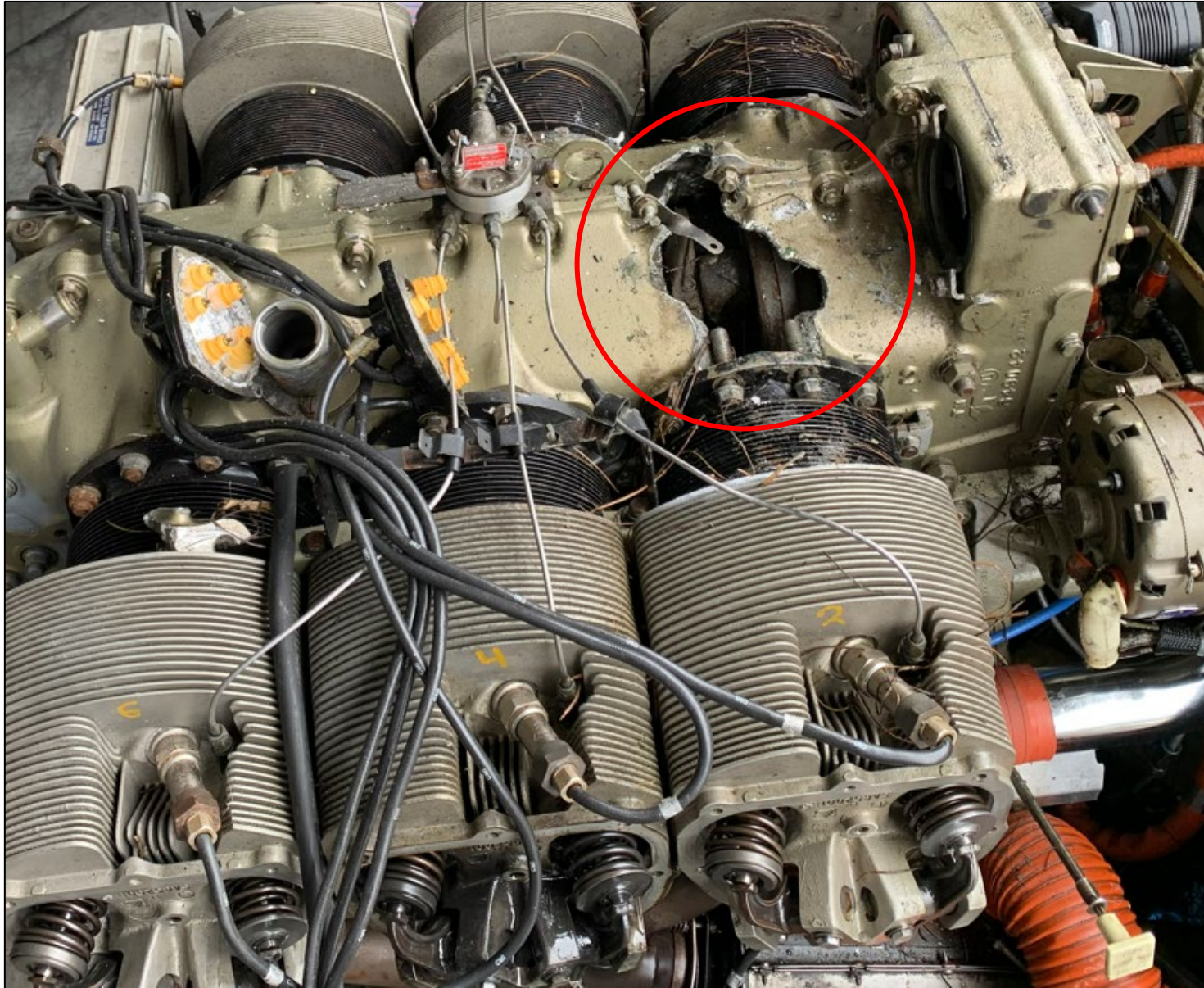
Figure 1: View of the engine damage originating at the No. 2 cylinder area (NTSB Photo)
