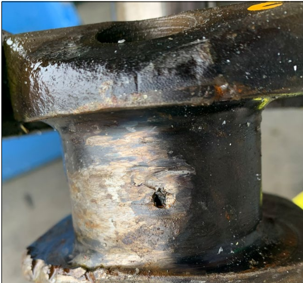
Crankshaft oil transfer hole at the No. 2 connecting rod attachment area.
