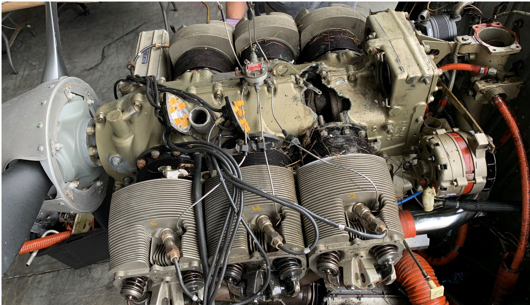
Photo 6: Overview of engine and damage near its aft end, concentrated near the No. 2 Cylinder (NTSB Photos)
