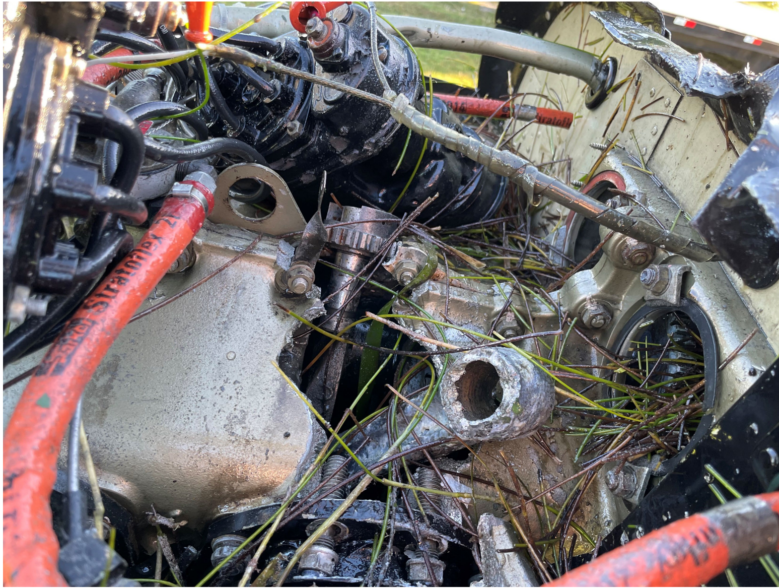
Photo 5: Overview of the engine damage near the No. 2 Cylinder (Photo Courtesy of FAA)
