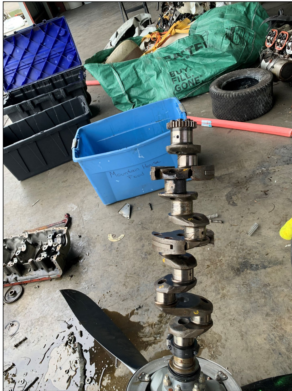
Photo 12: Overview of the crankshaft post disassembly (NTSB Photo)
