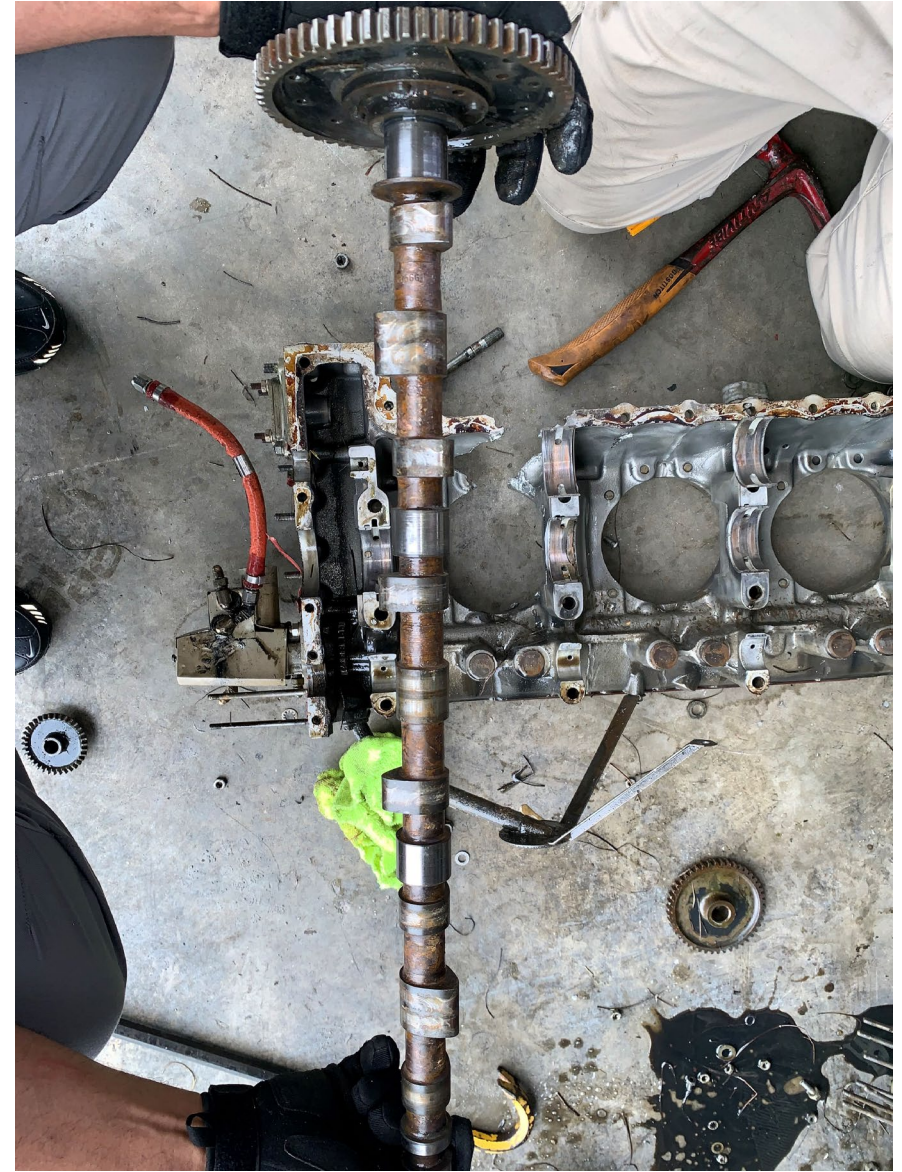
Photos 10, 11: Overview of the oil filter and the camshaft disassembled (NTSB Photo)
