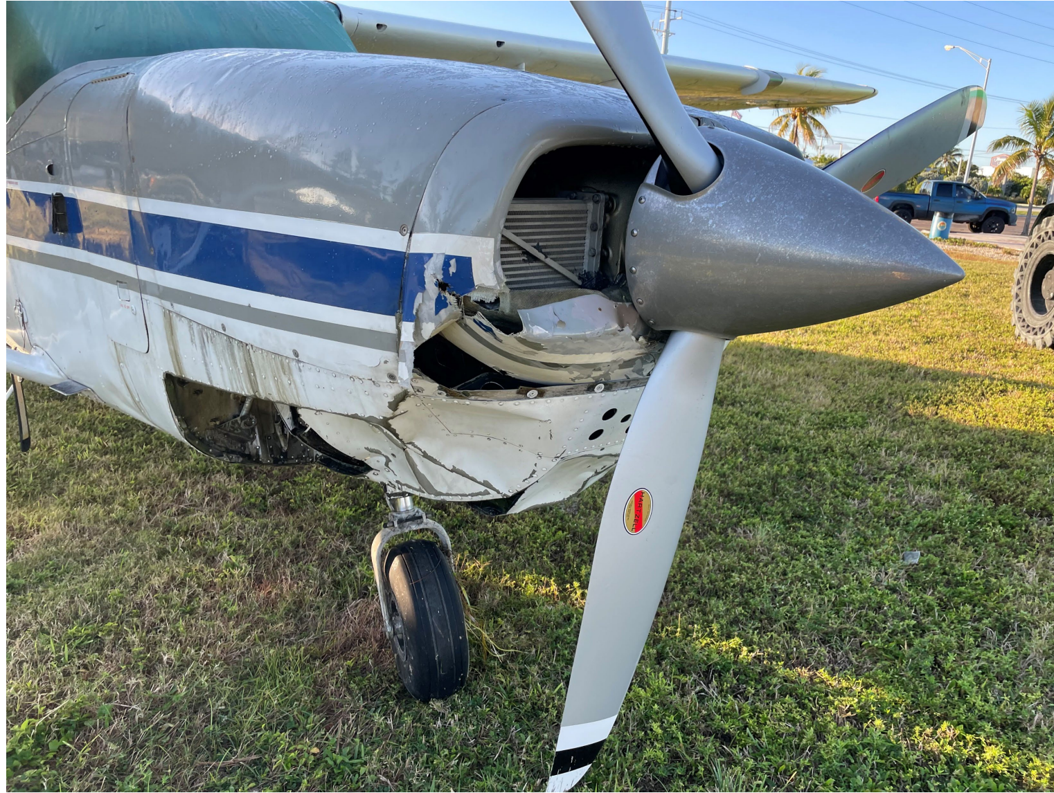
Photo 3: Overview of the cowling and engine area after the airplane had been recovered to shore (Photo Courtesy of FAA)
