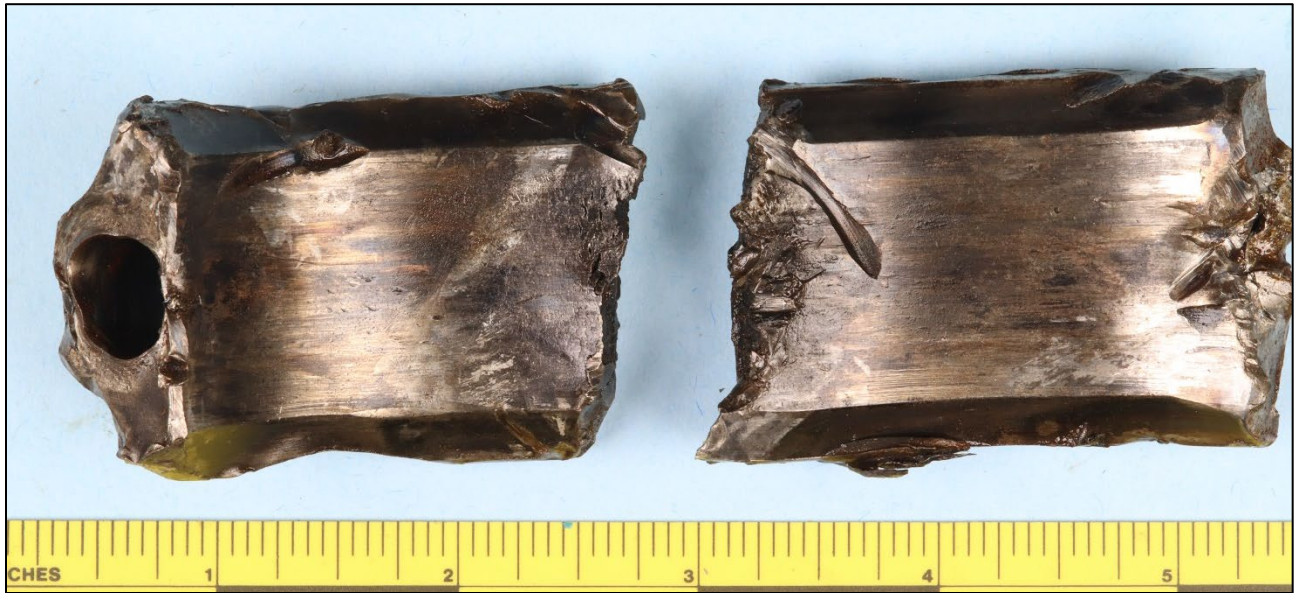
Figure 3. Interior surface of the fractured number 2 connecting rod cap.
