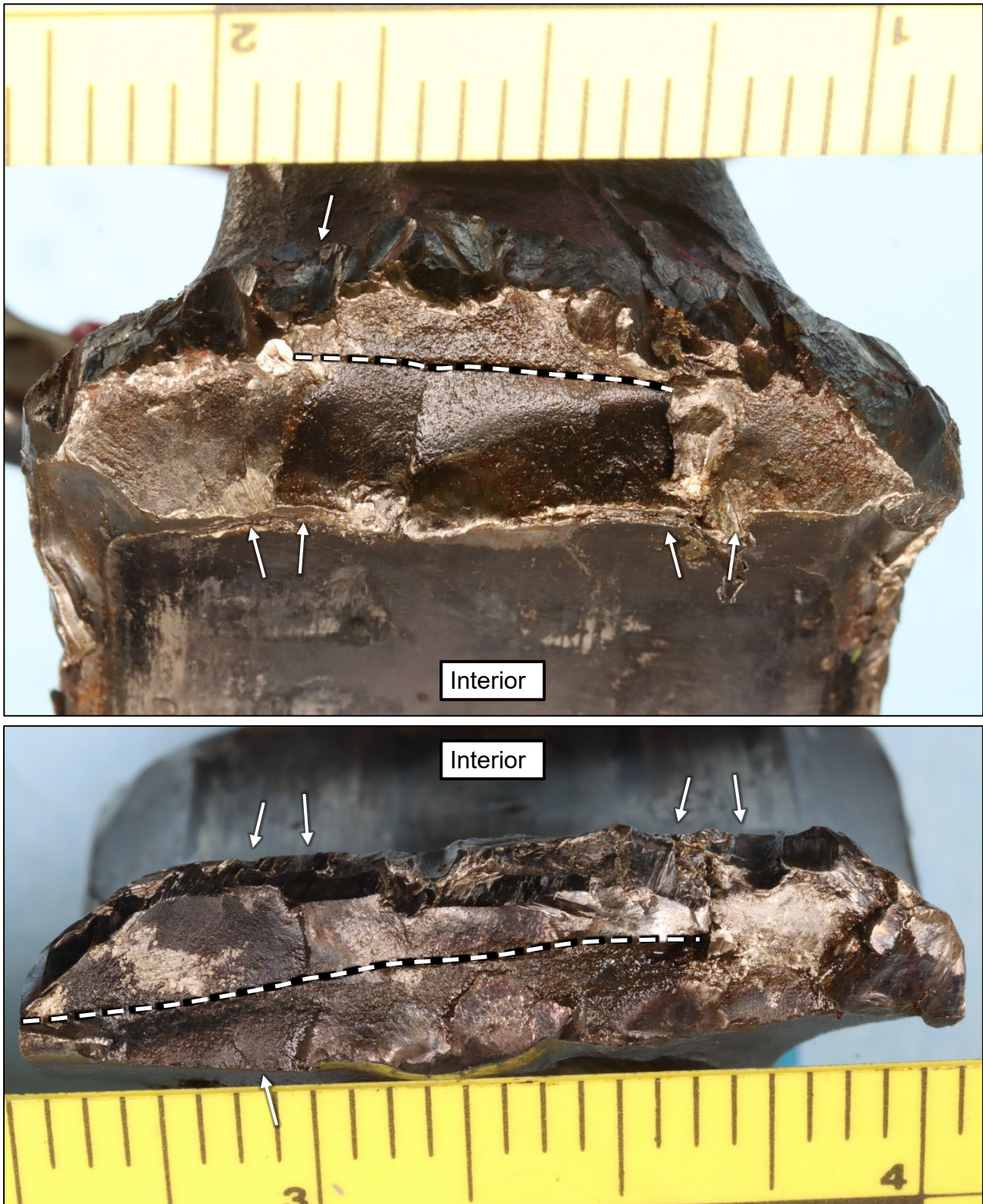
Figure 5. Mating fracture faces on strap A of the number 2 connecting rod. Dashed lines indicate partial fatigue boundaries, and arrows indicate approximate origin areas.
