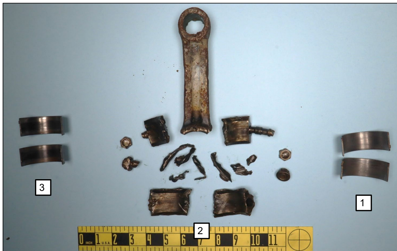
Figure 1. Overall view of the submitted number 2 connecting rod and bearing pieces and bearings from the numbers 1 and 3 connecting rods.
