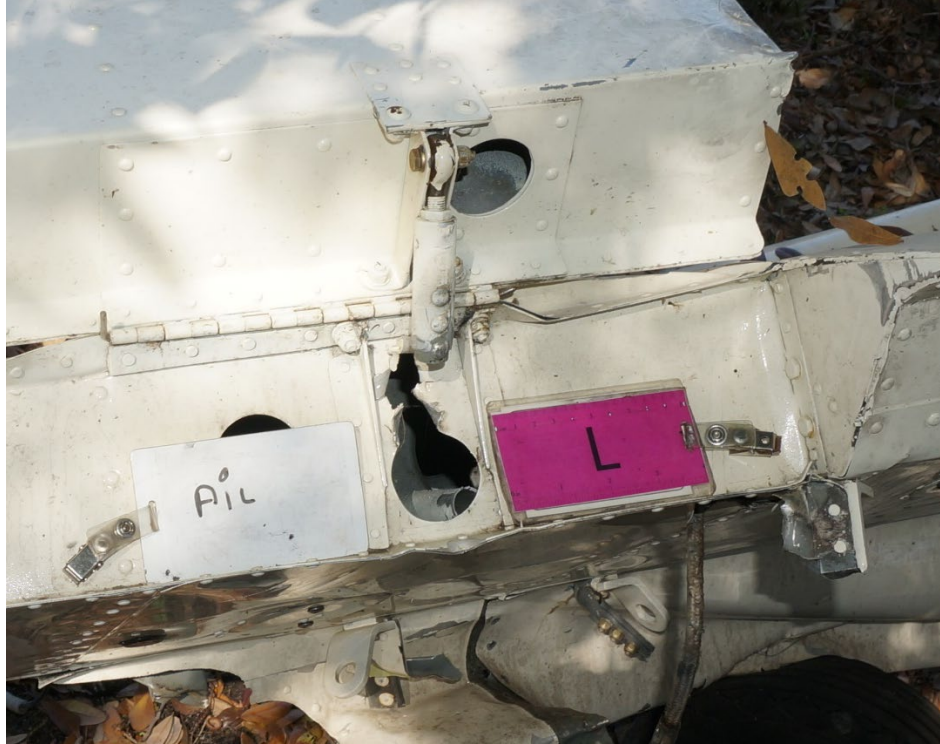
Figure 7 - Left Aileron Fractured Push-Pull Tube at Control Horn
