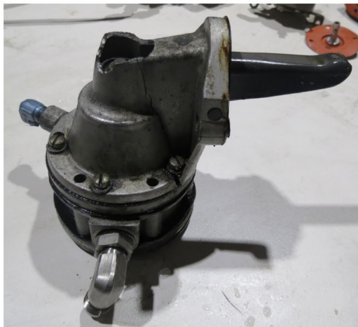
Figure 24 - Engine Driven Fuel Pump - Intact but Damaged (Left) Partially Disassembled (Right)
