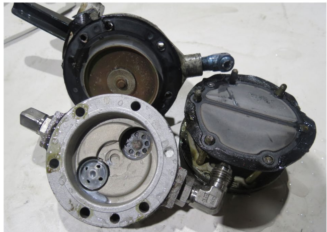
Figure 24 - Engine Driven Fuel Pump - Intact but Damaged (Left) Partially Disassembled (Right)
