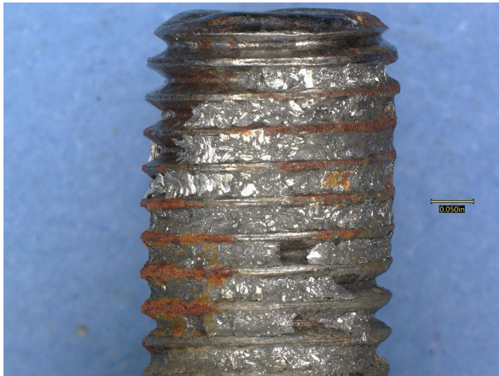
Figure 3: Threaded end of rod end after ultrasonic cleaning.
