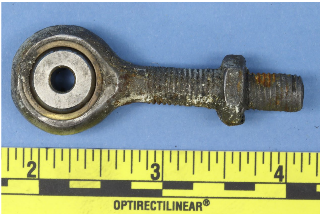
Figure 2: Rod end prior to cleaning.
