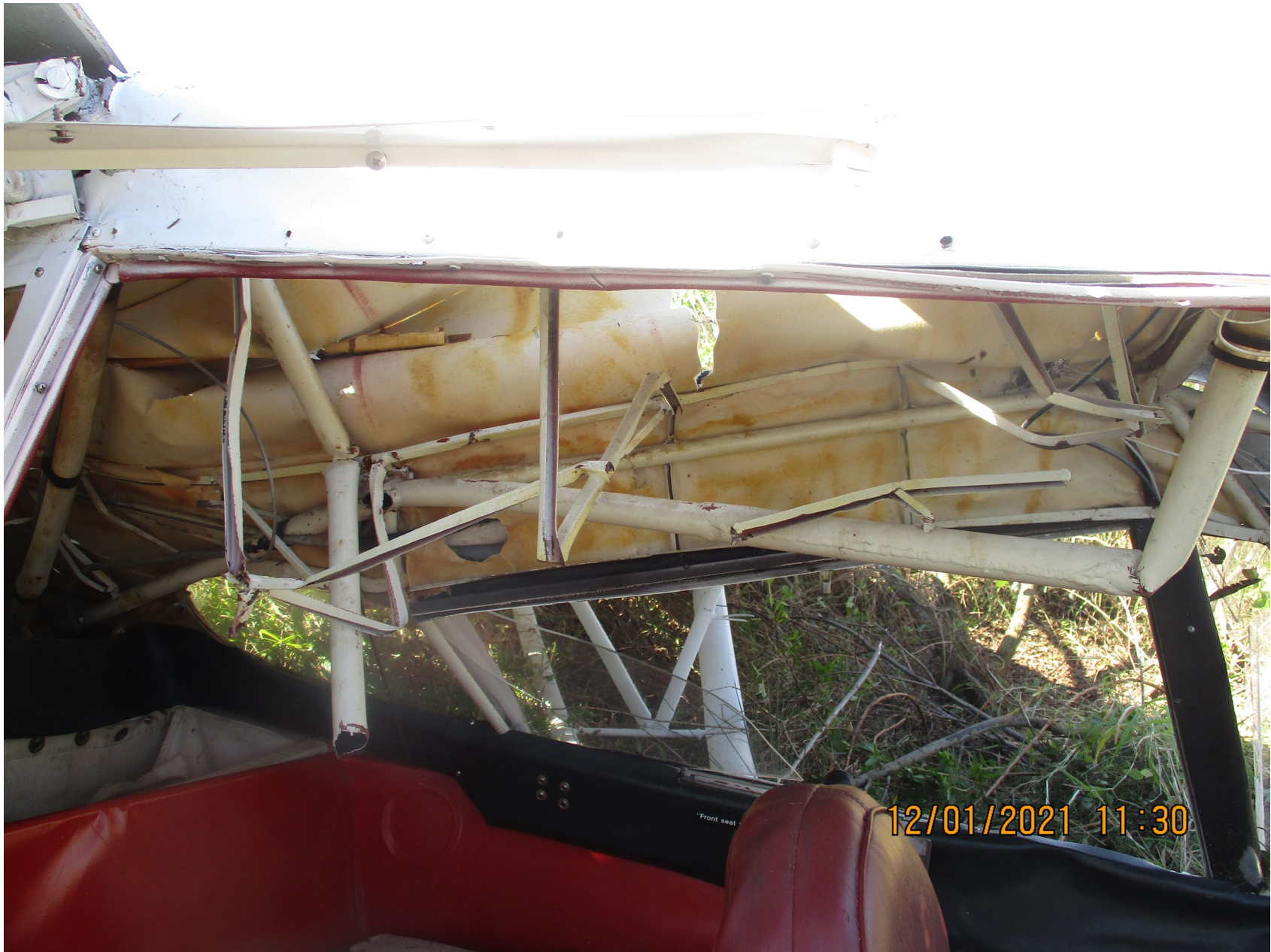
Photo 7 – Internal Fuselage Damage – Courtesy of FAA
