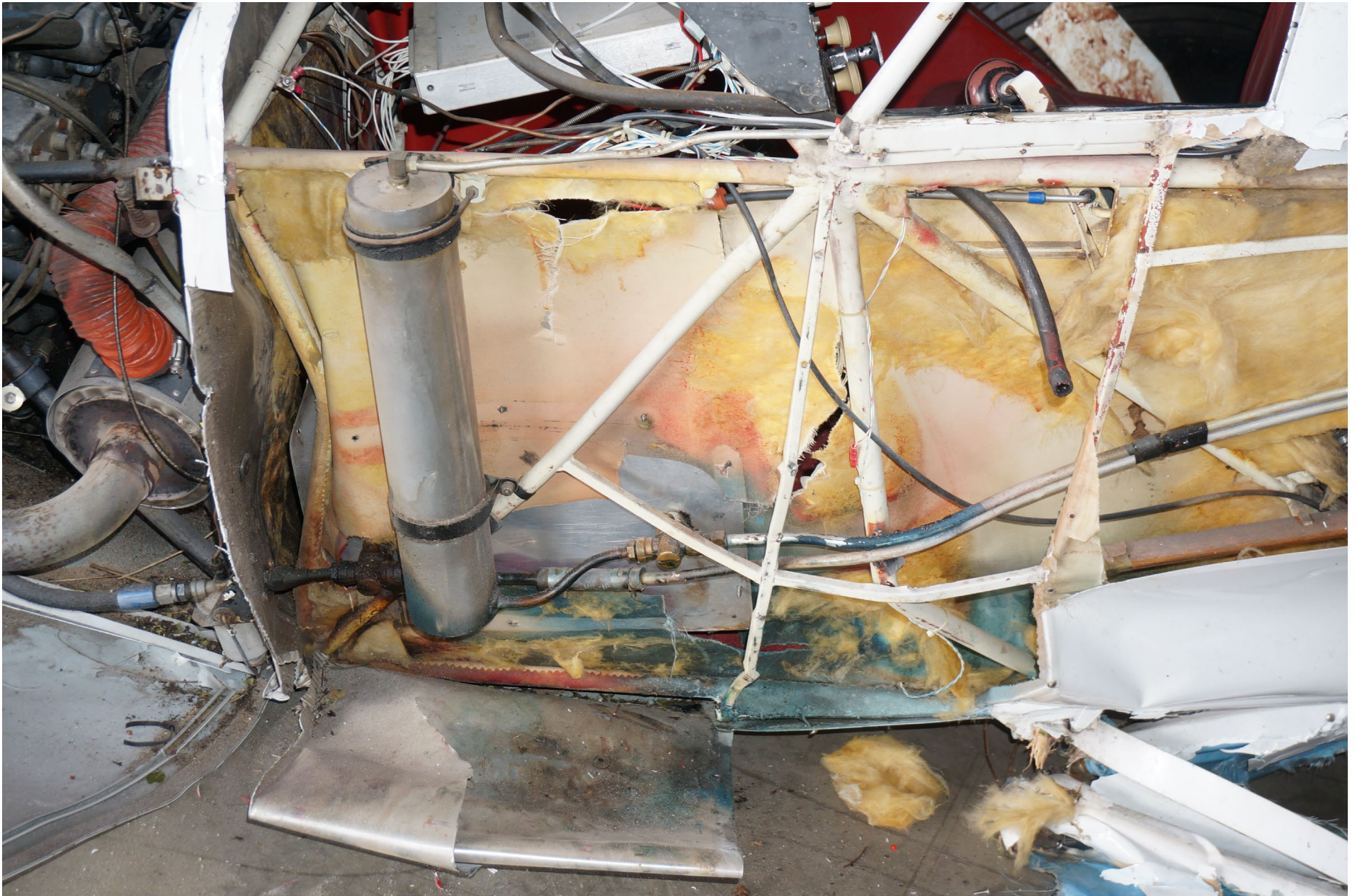
Photo 14 – Accident Airplane’s Modified Fuel System
