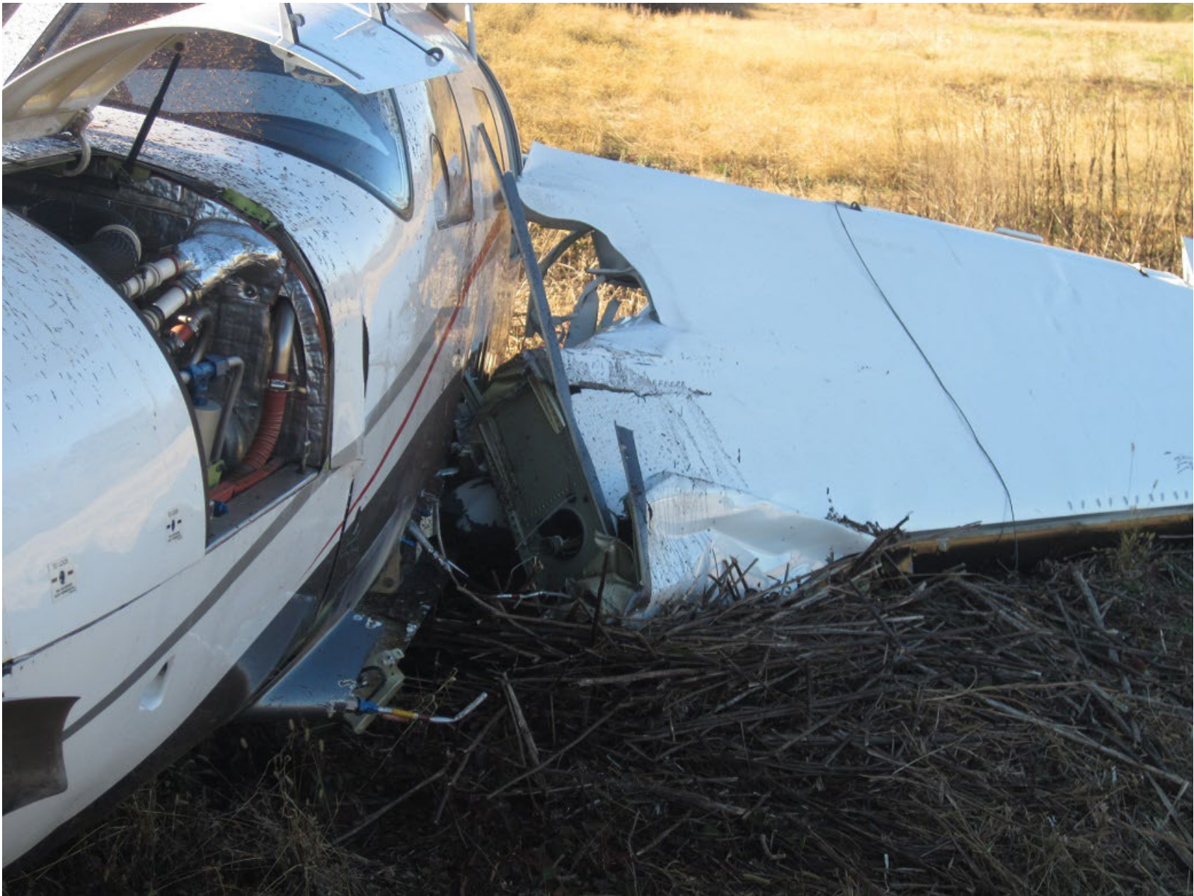
Photo 2 – Separated Left Wing (Photo Courtesy of FAA)
