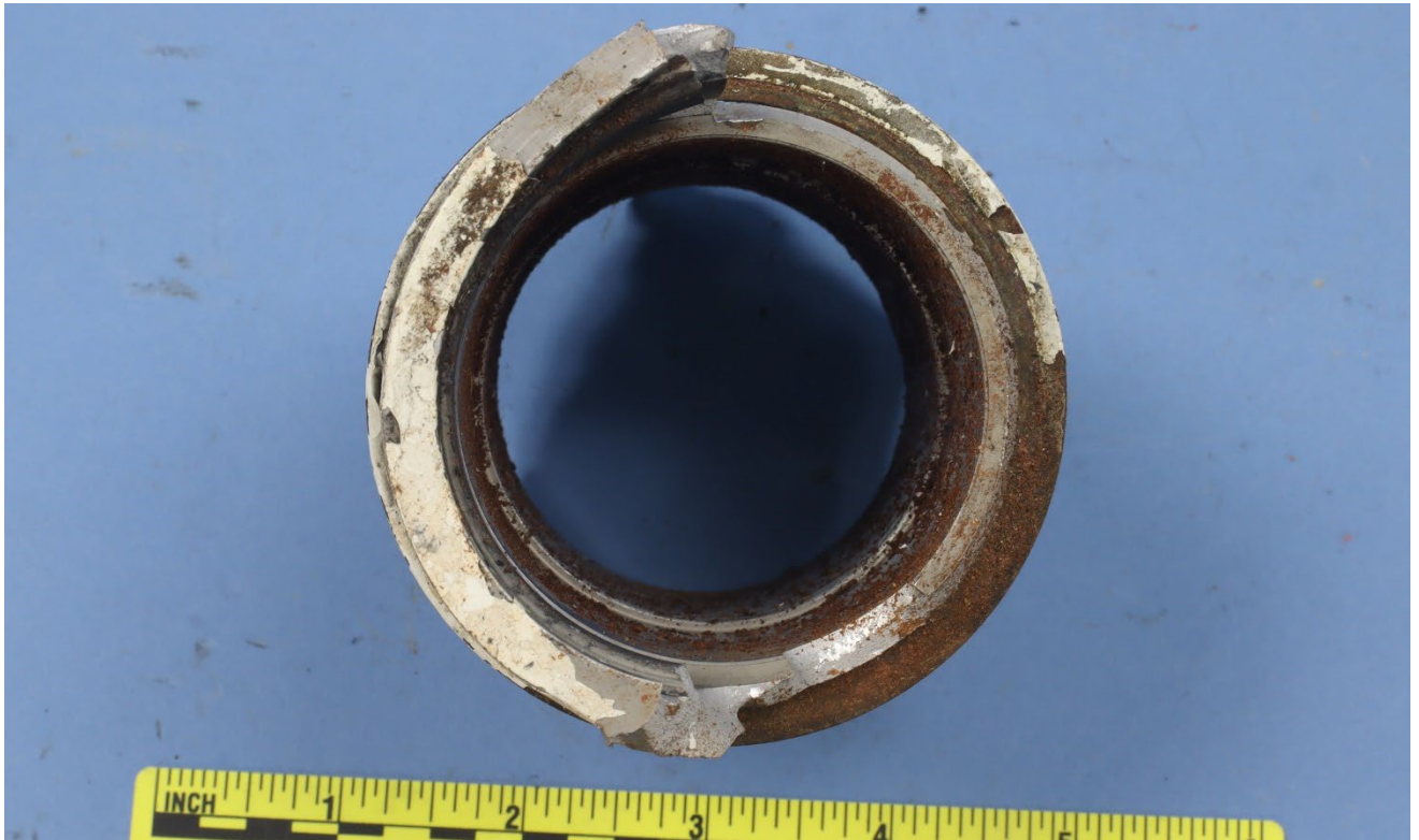
Figure 4 – View of the fractured area along and around the slotted portion of the trunnion.
