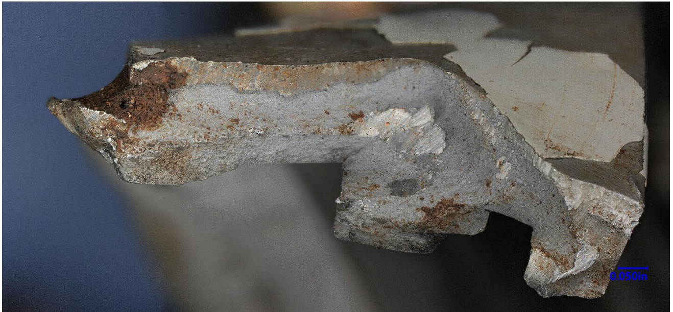
Figure 7 – Montage of the opposite edge of the slotted-side trunnion fracture.
