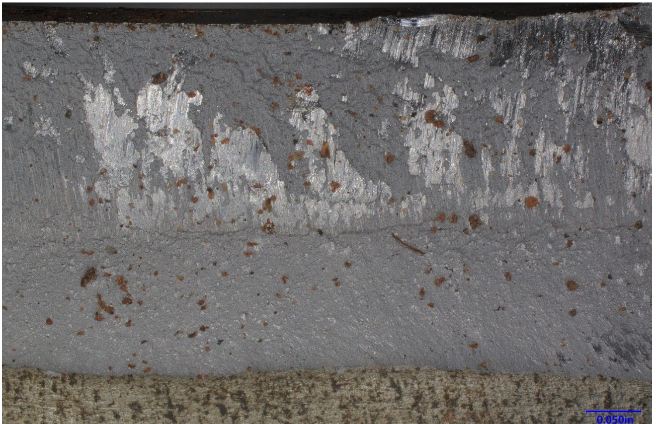
Figure 5 – Typical area of the trunnion circumferential barrel fracture.
