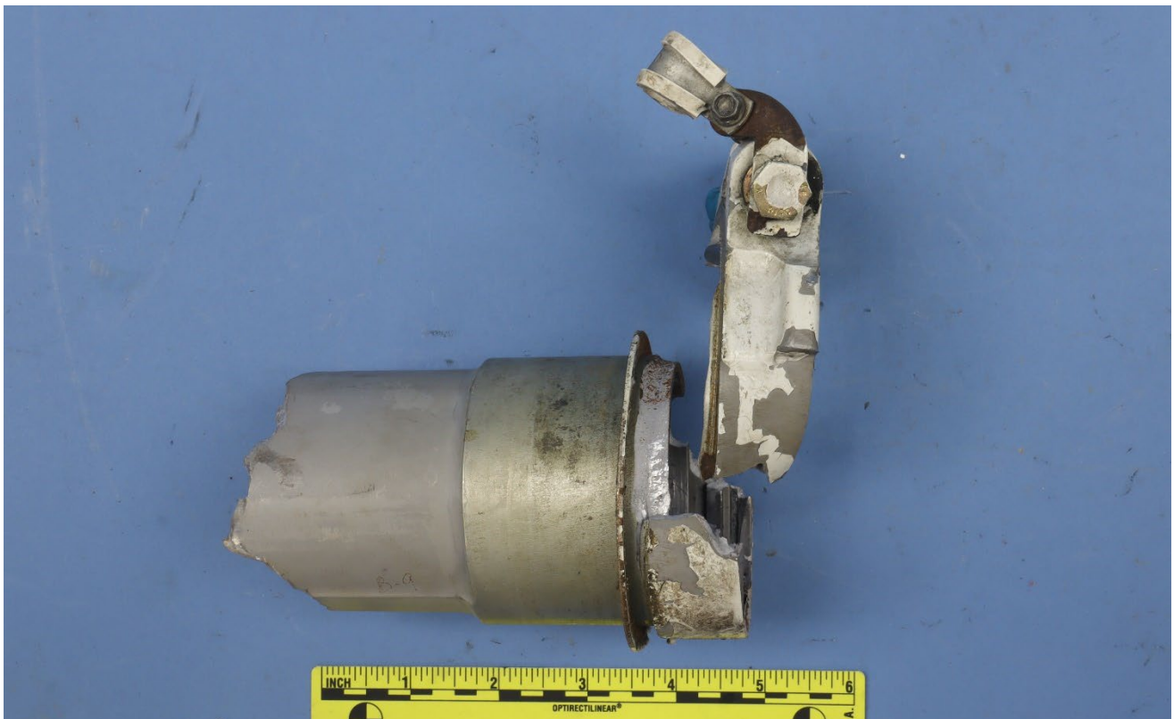
Figure 2 – Side view of the trunnion remnants, aligned to show the orientation of the mating fracture surfaces on the slotted bore.
