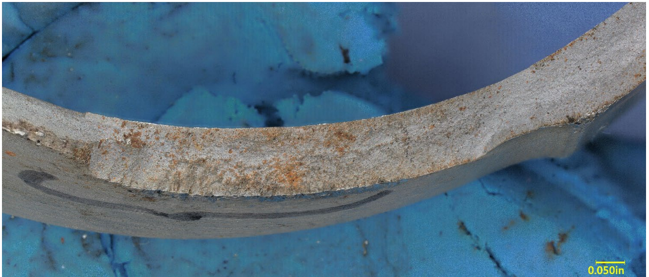
Figure 8 – View of a section of the non-slotted fractured surface of the trunnion cylinder, showing repeating parallel features near the outside edge.
