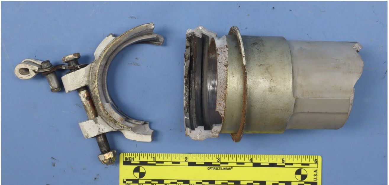
Figure 1 – View of the fractured remnants of the trunnion, as received.
