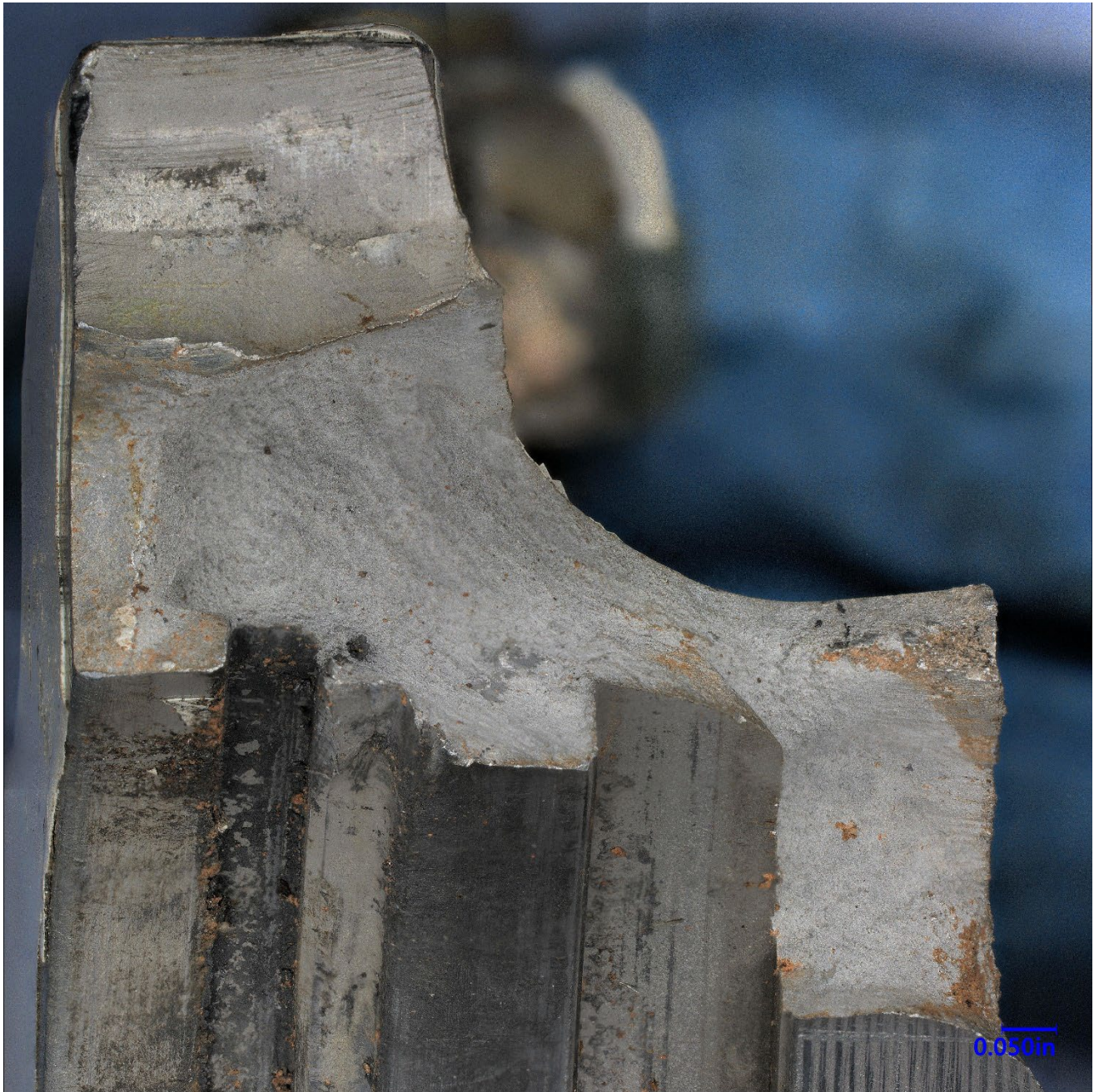
Figure 6 – Montage of the one of the edges of the trunnion fracture surface along the slotted bore, viewed from the interior.
