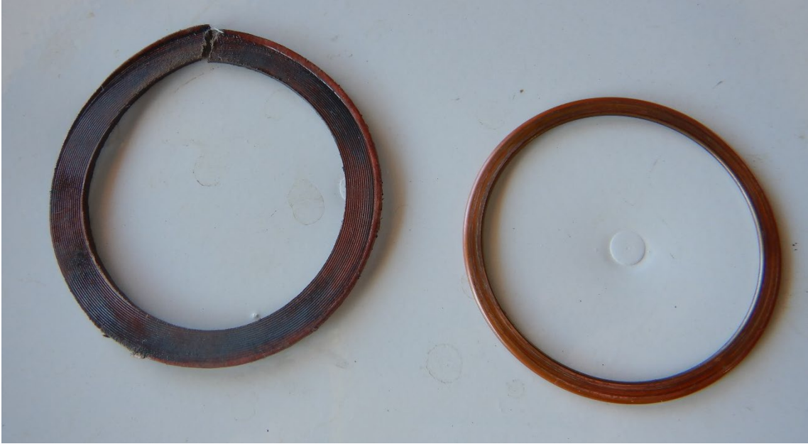
Figure 9 - View of fiber and copper gaskets
