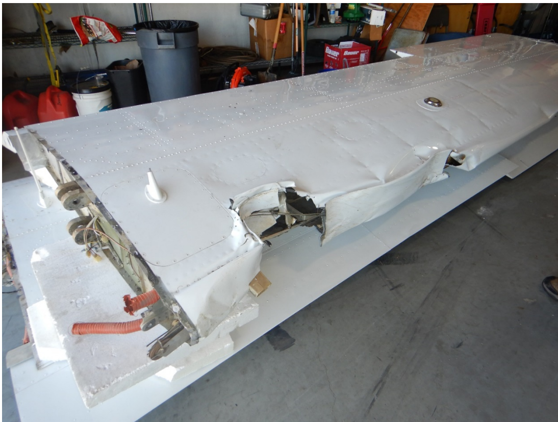
Figure 3- Leading edge damage of left wing (stored above right wing in hangar)
