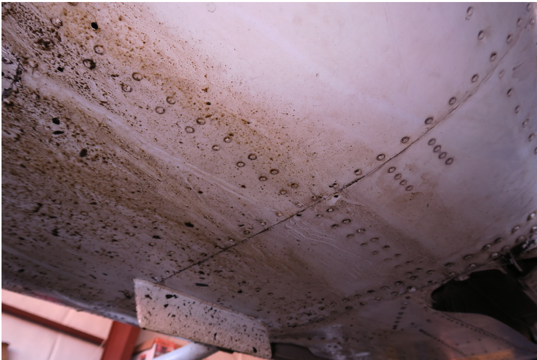
Figure 5- Oil on underside of fuselage
