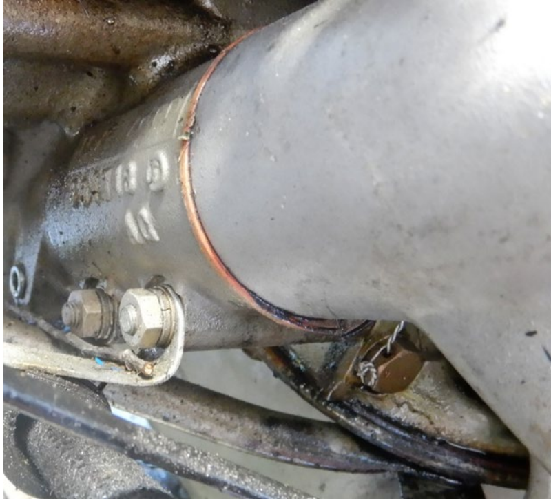
Figure 7 – Close-up view of lower (fiber) gasket on oil filter adapter
