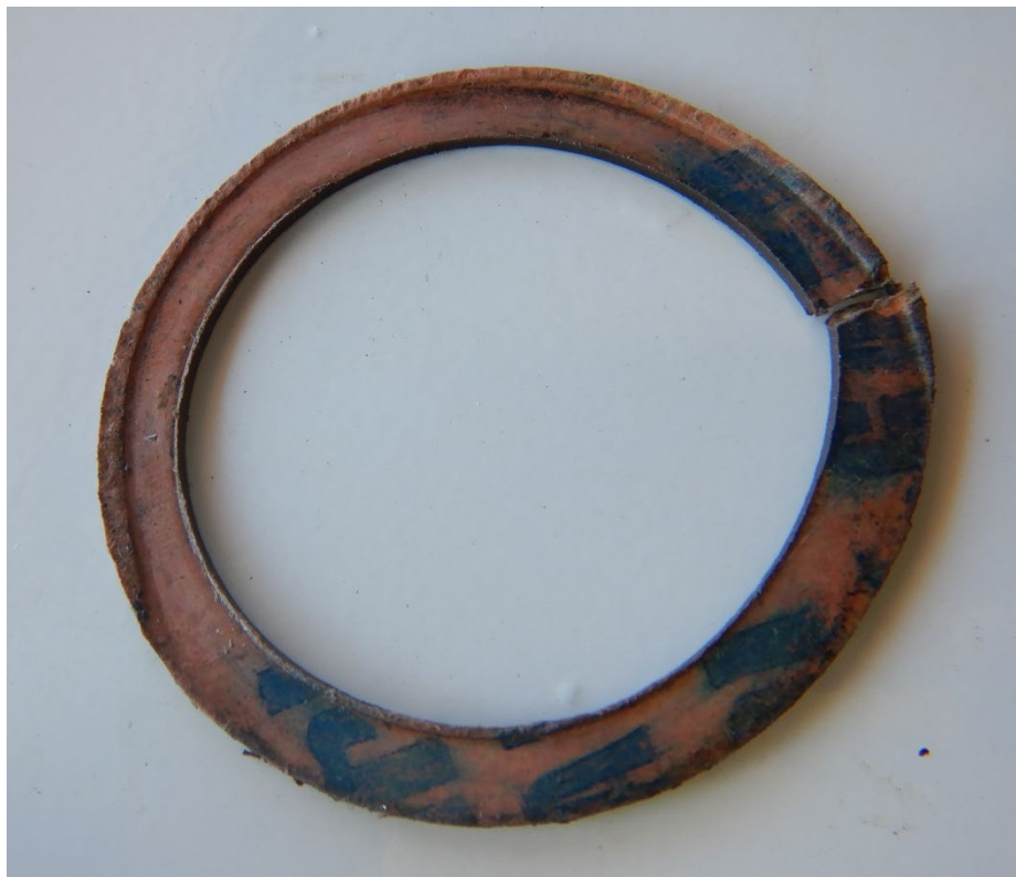
Figure 8 - Close-up view of torn fiber gasket
