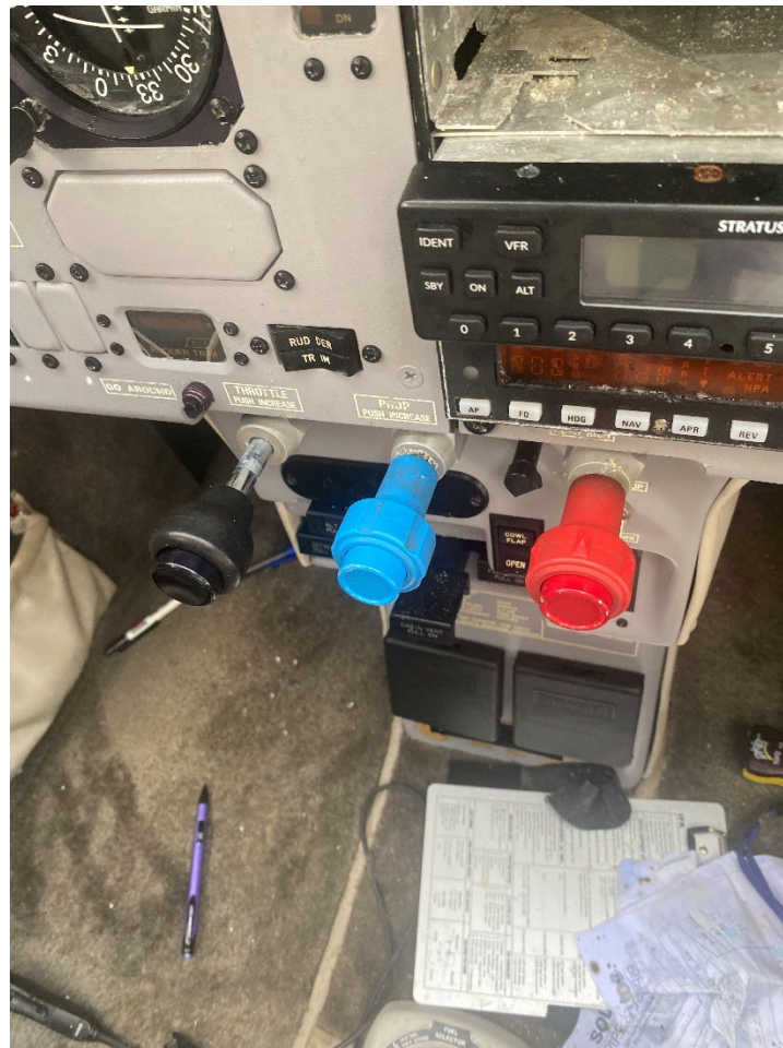
Figure 2: View of the positions of the throttle and mixture Controls for pressure testing the engine compartment fuel System Components.
