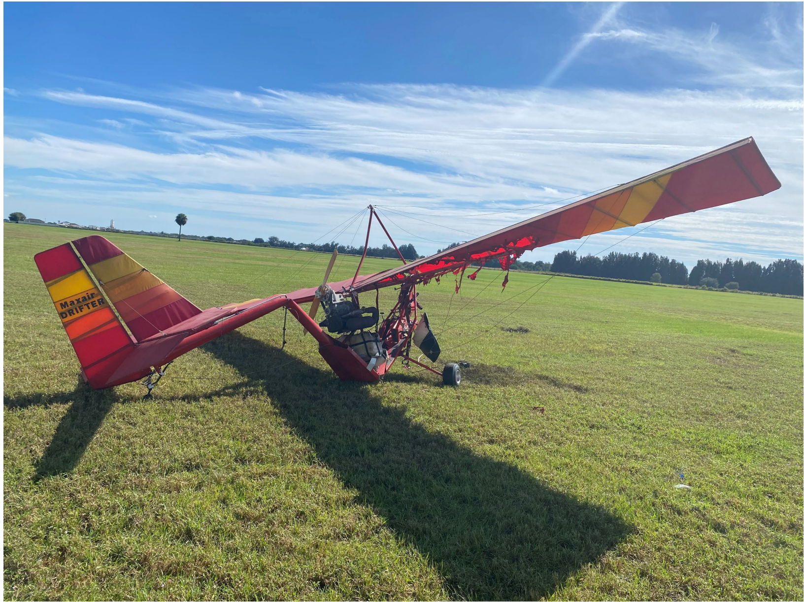
Photo 2 – View of the boom and wing damage (Photo Courtesy of FAA)
