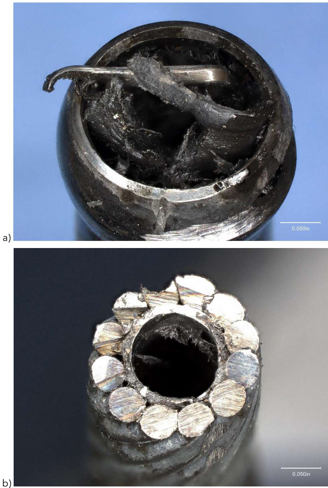
Figure 9. a) Image at end of guide rod sleeve showing remnant wire fragment and black plastic material and b) image at end of cable housing showing lack of inner lining.
