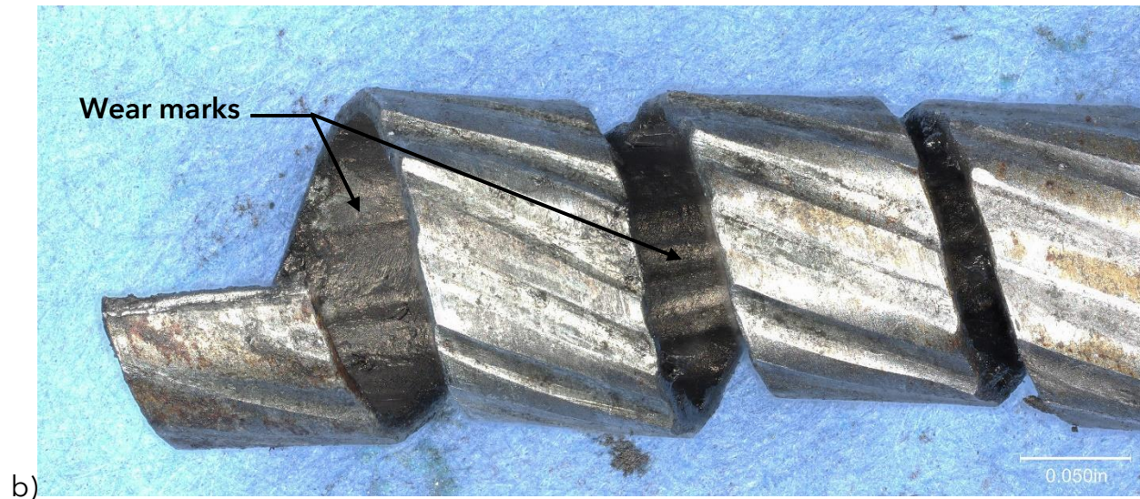
Figure 10. a) Image of disassembled cable housing (outer wires not shown). Deformation and fracture of the helical winding was caused during disassembly; b) image of the helical winding at the end of the cable housing with the windings spread apart to show the wear marks on the inner diameter surface.
