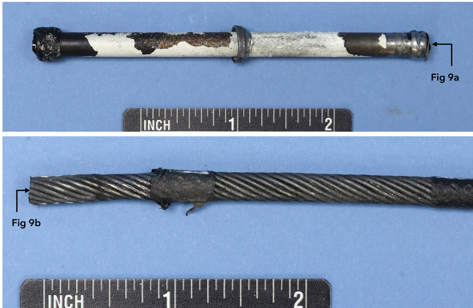
Figure 8. Top image: Guide rod sleeve after sectioning the ferrule. Lower image: Cable housing after removing the ferrule.
