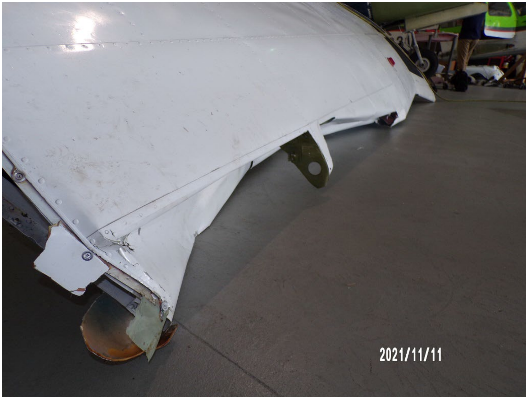
Photo 2 – Right Wing Damage (Photo Courtesy of Insurance Adjuster)
