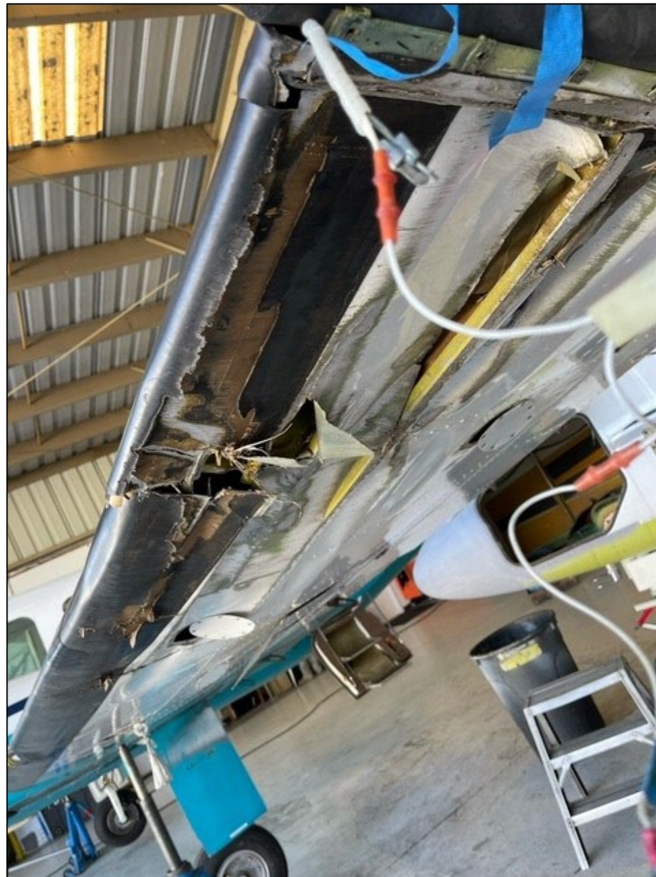
Photo 2 – View of the left-wing damage (Photo Courtesy of FAA)
