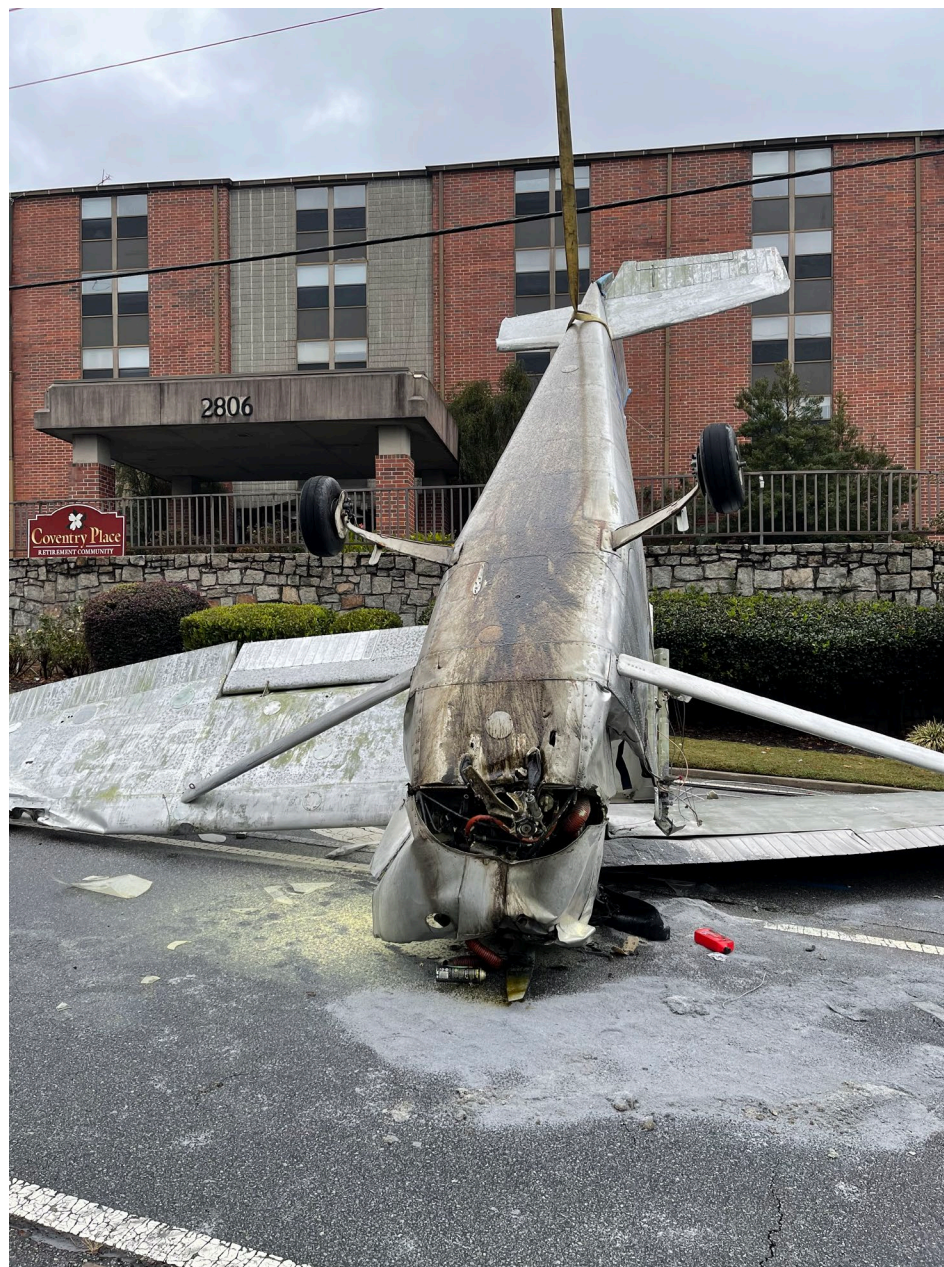
Photo 1 – FAA Digital Photograph. View of the Airplane at the Accident Site. Note the oil Covering the Entire Length of the Exterior of the Bottom Fuselage Skin, and the Damaged Left Horizontal Stabilizer and Elevator.
