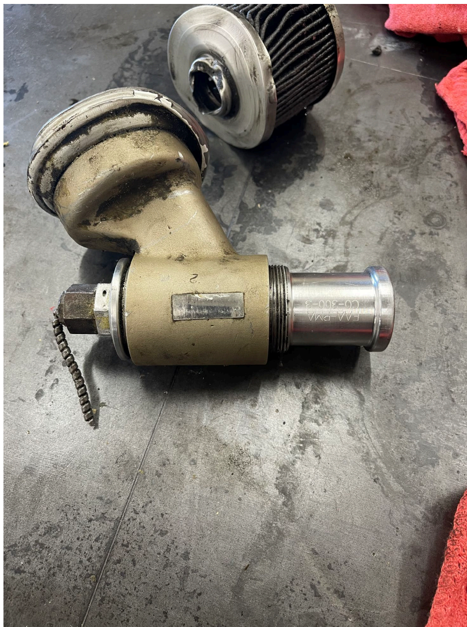
Photo 4 - FAA Digital Photograph. View of the Oil Filter Adapter and Installed Base of Oil filter, and also Oil Filter Element Separated For the Investigation.
