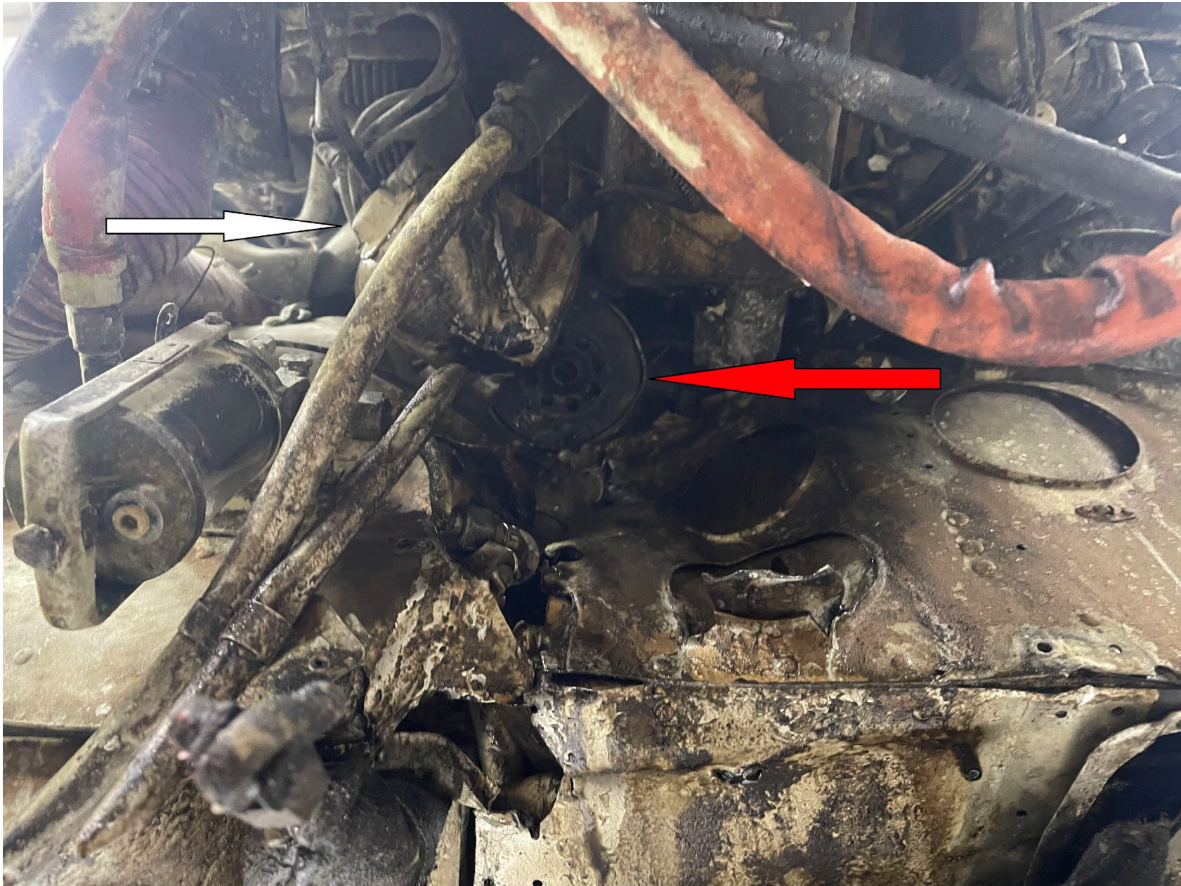
Photo 3 – Annotated FAA Digital Photograph. White Arrow Depicts upper Portion of the Separated Oil Filter and Red Arrow Points to Base of the Oil Filter Attached to the Oil Filter Adapter. Note the Impact Damaged Oil Filter.
