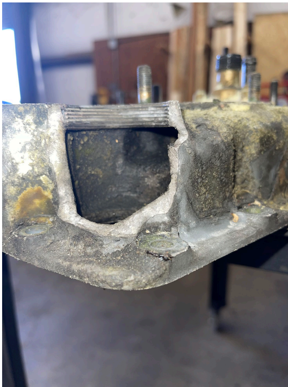
Photo 5 - FAA Digital Photograph. View of the Fractured Lower Portion of the Accessory Case that Accepted the Threaded Portion of the Oil Filter Adapter.
