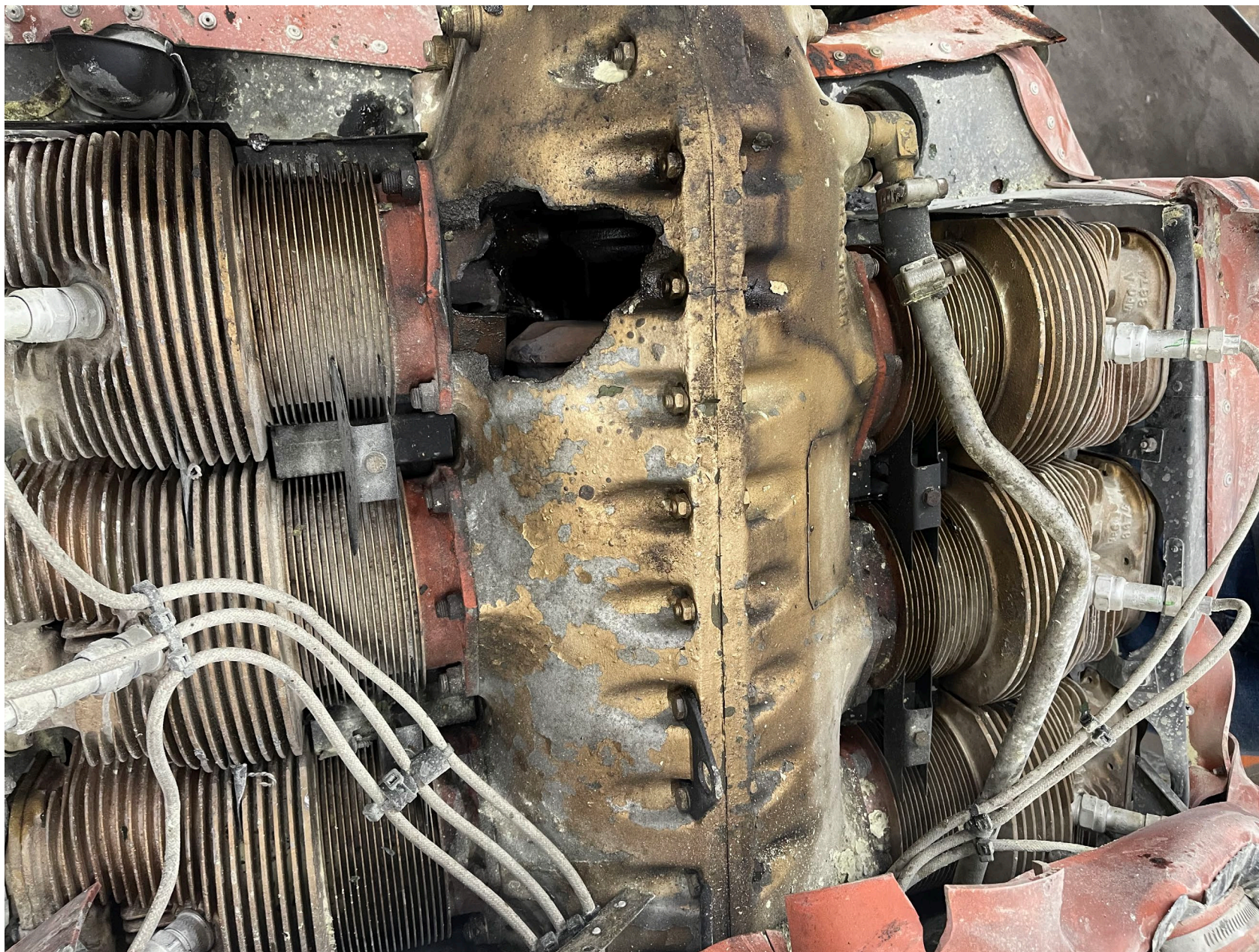
Photo 2 - FAA Digital Photograph. View of the Hole in the Engine Crankcase Above the No. 6 Cylinder.
