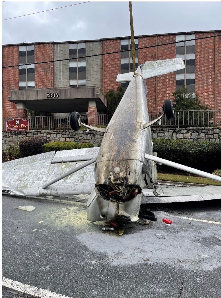
Figure 1: FAA Digital Photograph. View of the Airplane at The accident site. Note the oil covering the bottom of the Fuselage.
