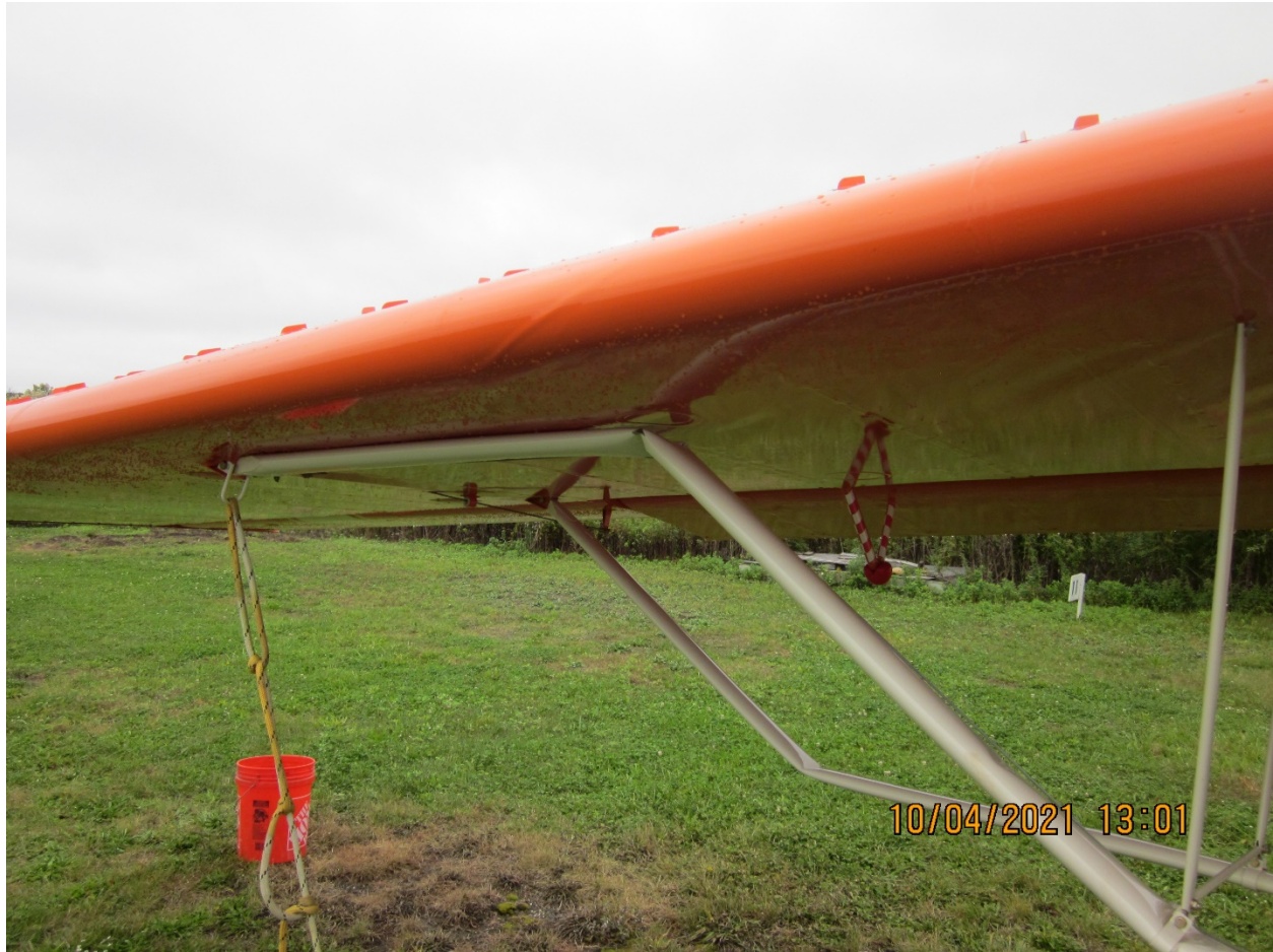
Photograph 2 2 – Accident airplane – right wing and strut damage.
