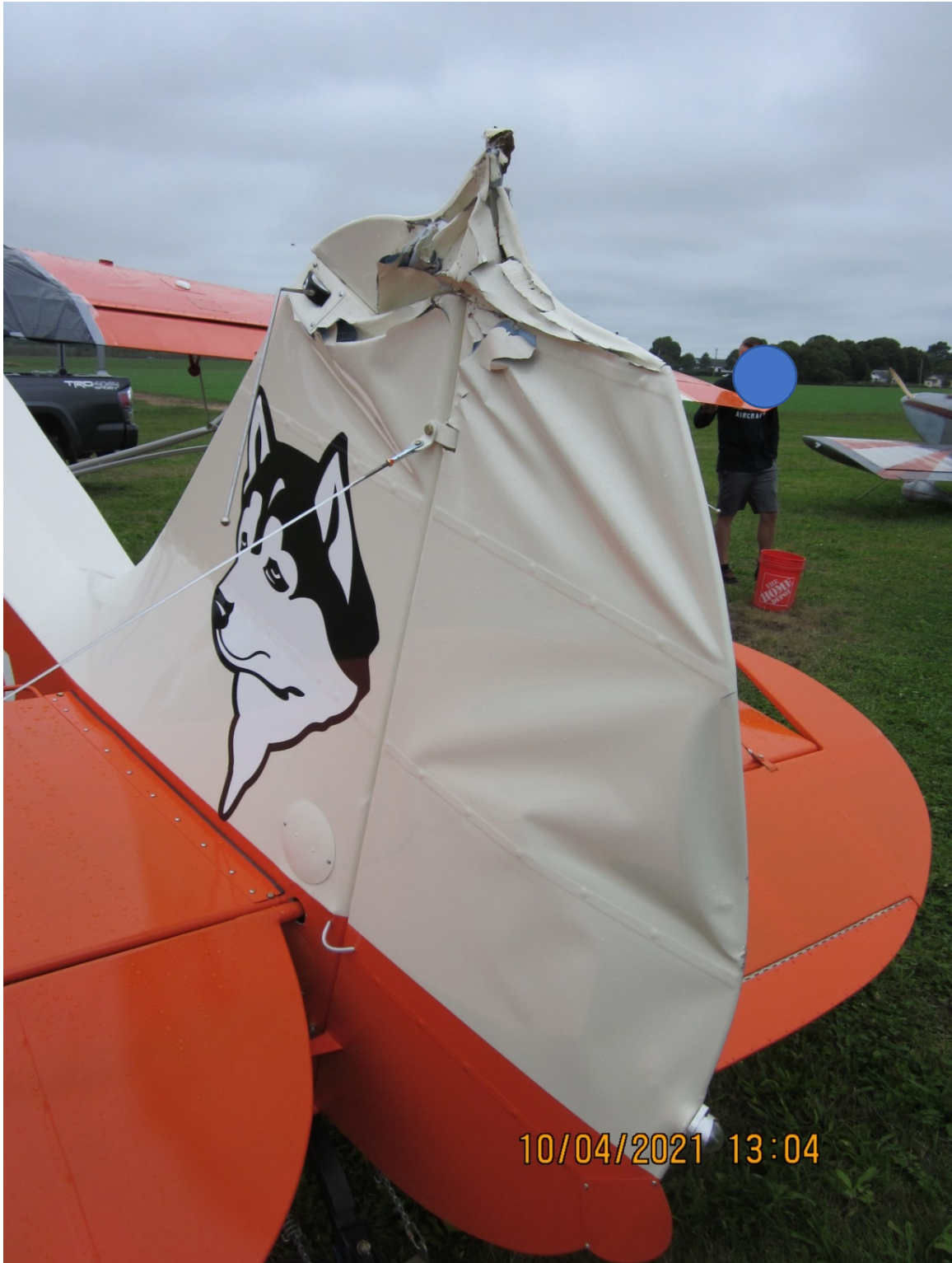
Photograph 3 3 – Accident airplane – Rudder damage.
