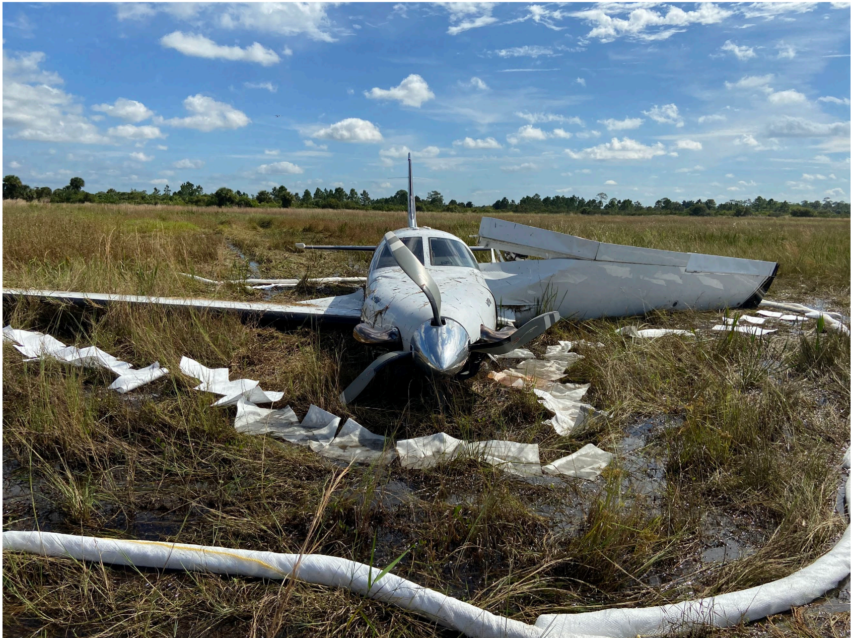
Photo 1 – FAA Digital Photograph. View Taken Forward of the Airplane at the Accident Site Looking Aft. Note the left wing leading edge Rotated down About 90 Degrees.
