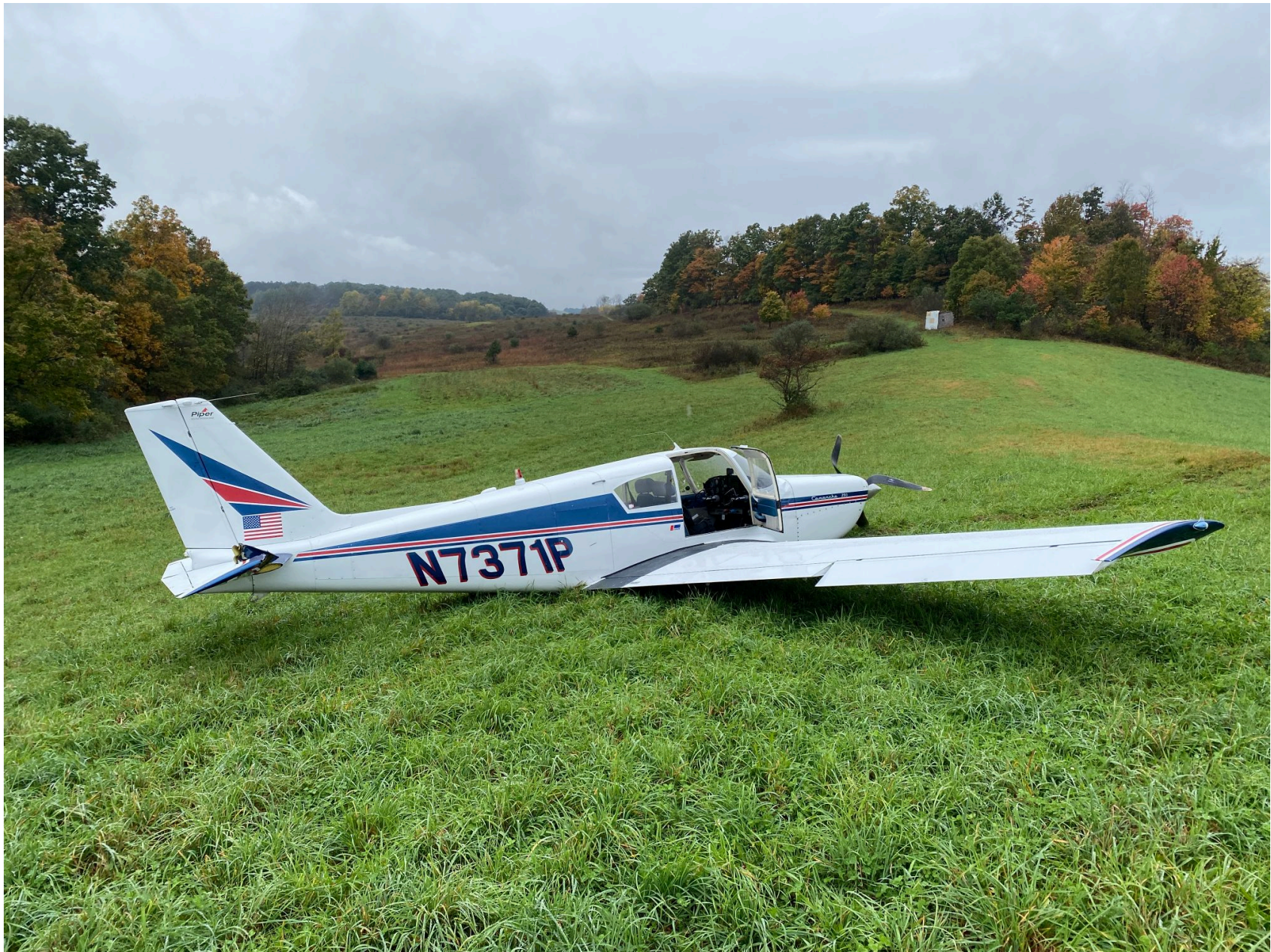
Photo 2 – View of right side of airplane showing horizontal stabilizer damage.
