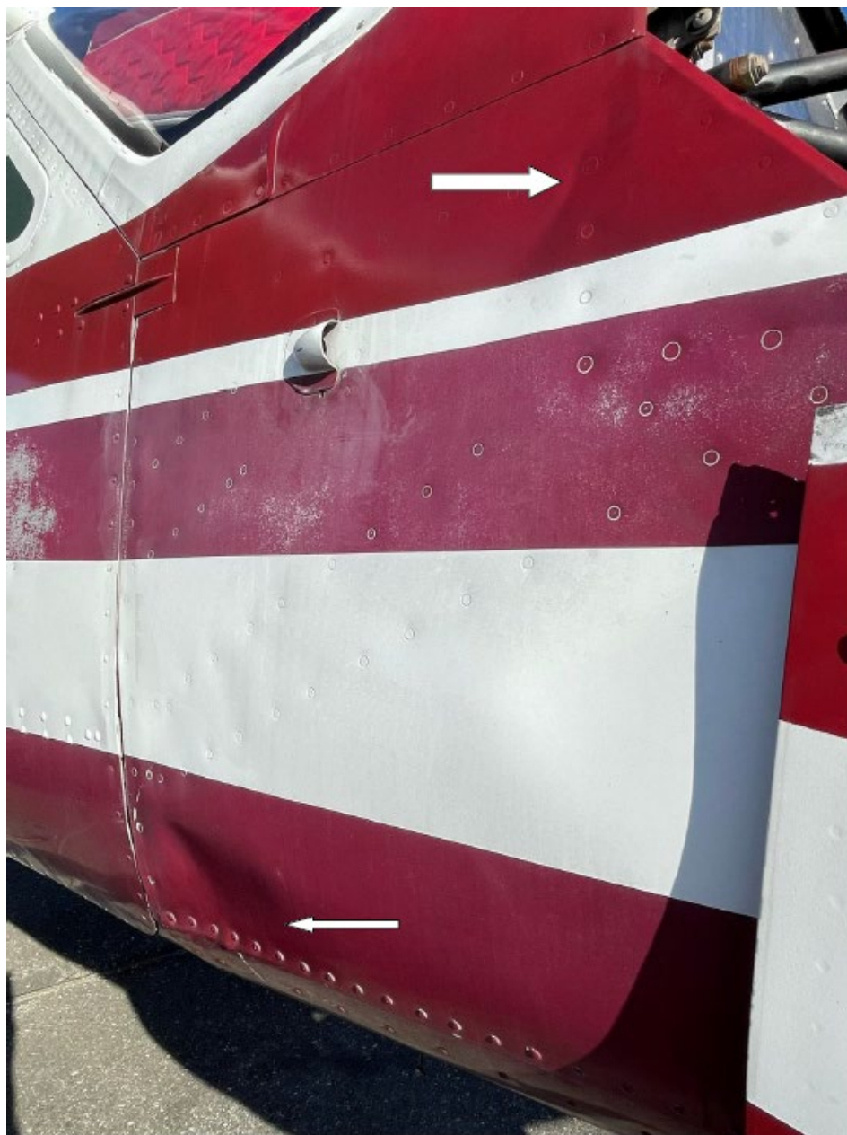
Photo 3 - Insurance Adjuster Digital Photograph. View of The Right Side of the Fuselage Between the Firewall and Front Portion of the Door. White Arrows denote Locations of Compression Wrinkles.
