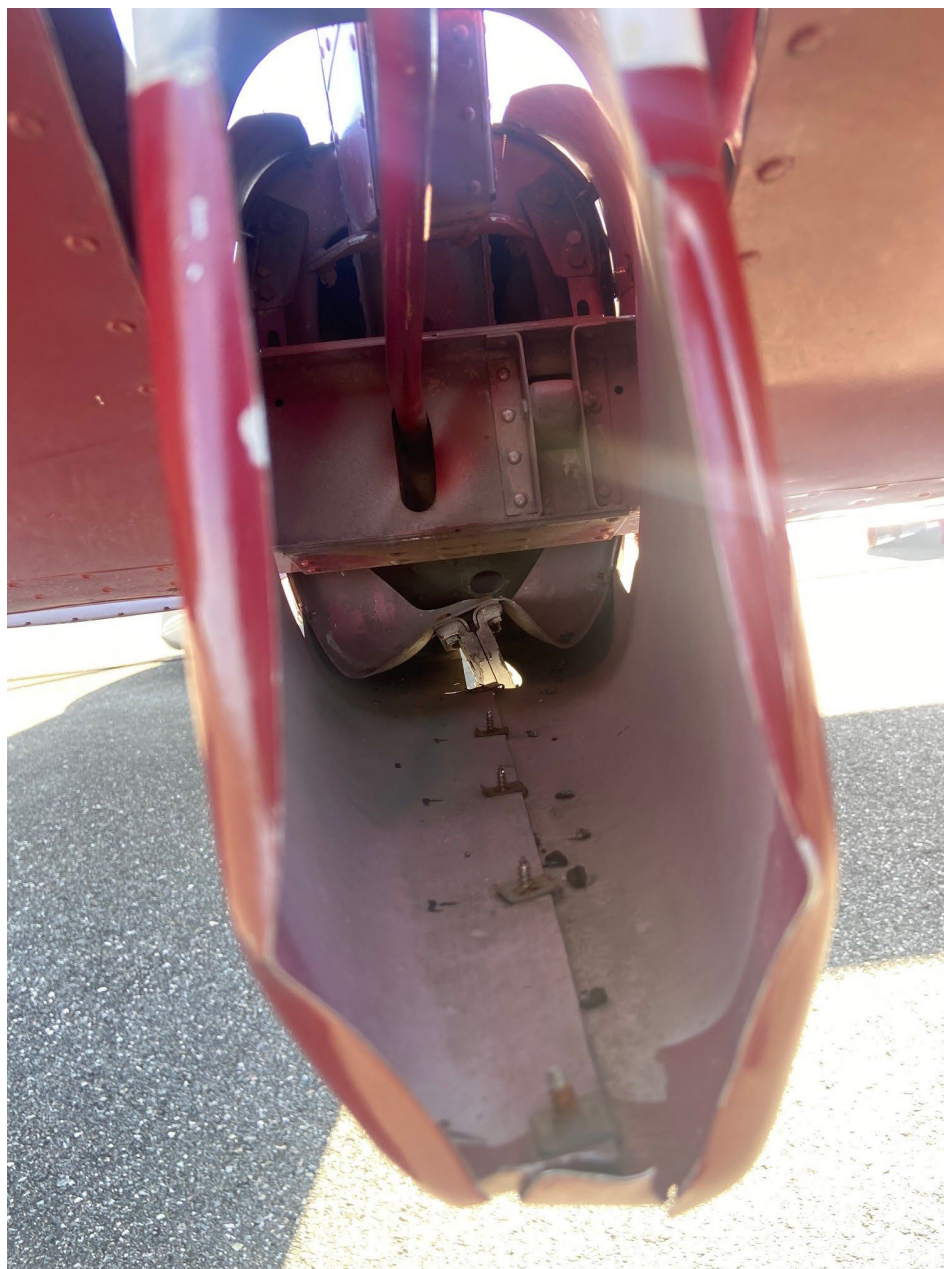
Photo 5 – Digital Photograph From Flight Instructor. View From Aft Looking Forward Showing Damage to Lower portion of Bulkhead Assembly Part Number 1712105-1 at Fuselage Station 281.48
