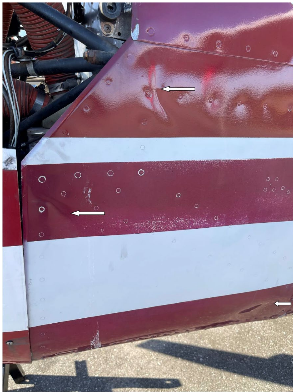
Photo 2 - Insurance Adjuster Digital Photograph. View of The Left Side of the Fuselage Between the Firewall and Front Portion of the Door. White Arrows denote Locations of Compression Wrinkles.
