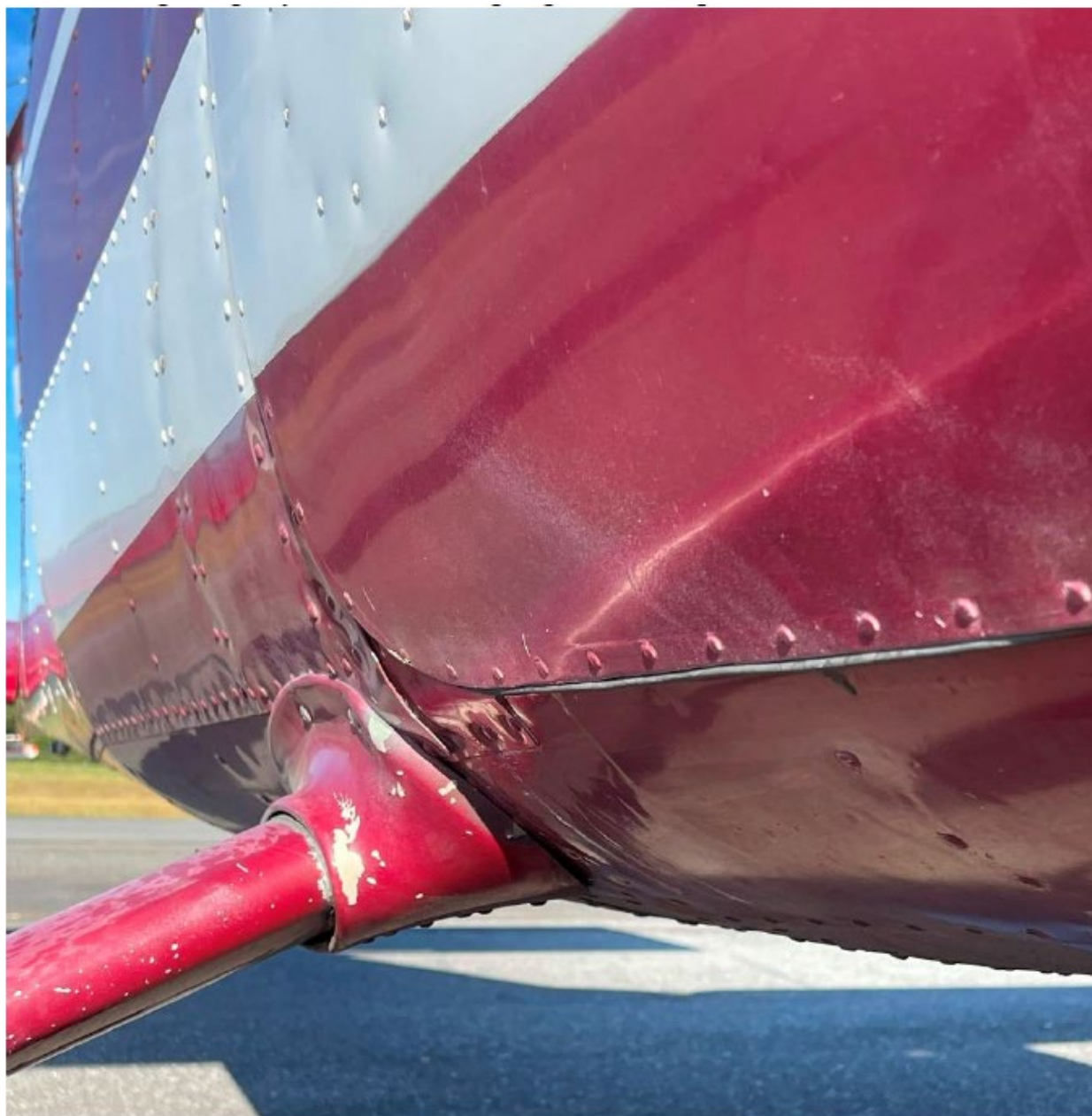
Photo 4 - Insurance Adjuster Digital Photograph. View of The Right Side of the Fuselage At the Main Landing Gear Attach. Note the Slight Deformation.
