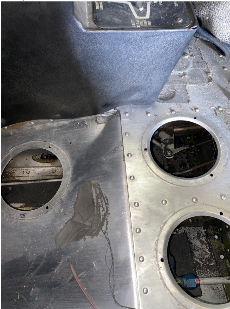
Photograph 1 – Accident airplane – Left pilot seat floor buckling.
