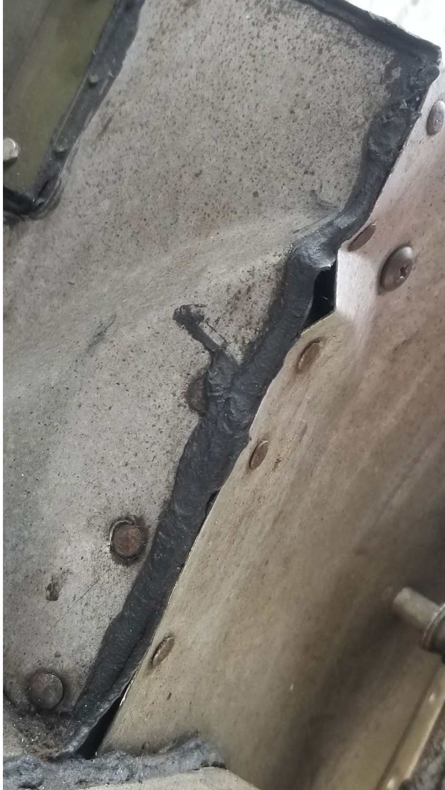
Photograph 3 – Accident airplane – Bulkhead damage
