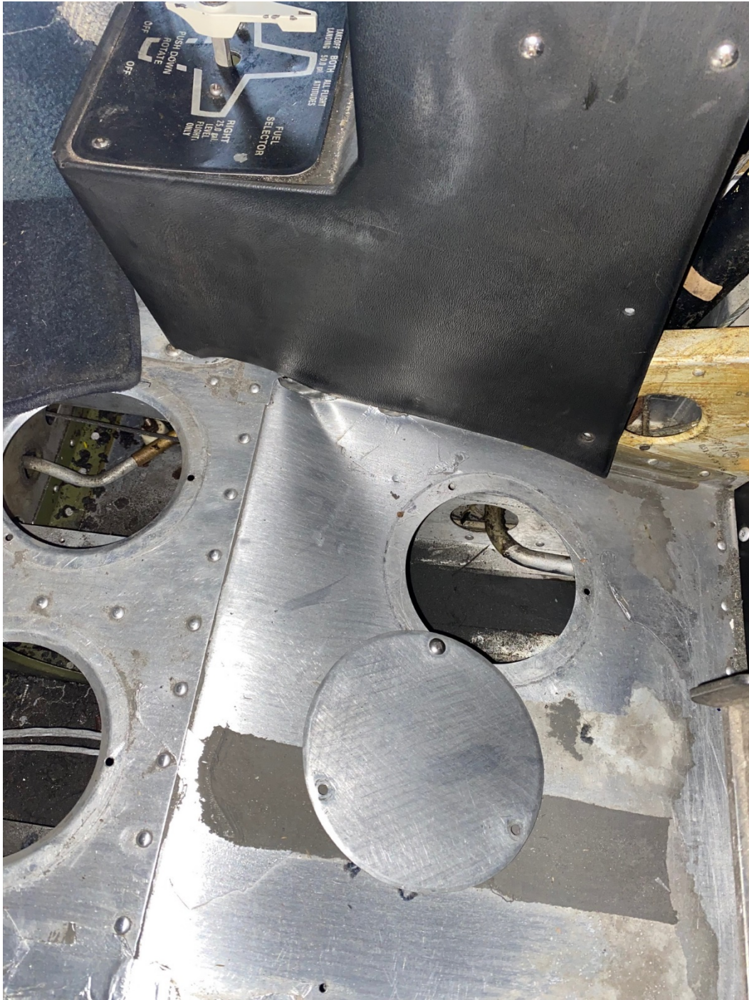
Photograph 2 – Accident airplane – Right pilot seat floor buckling.
