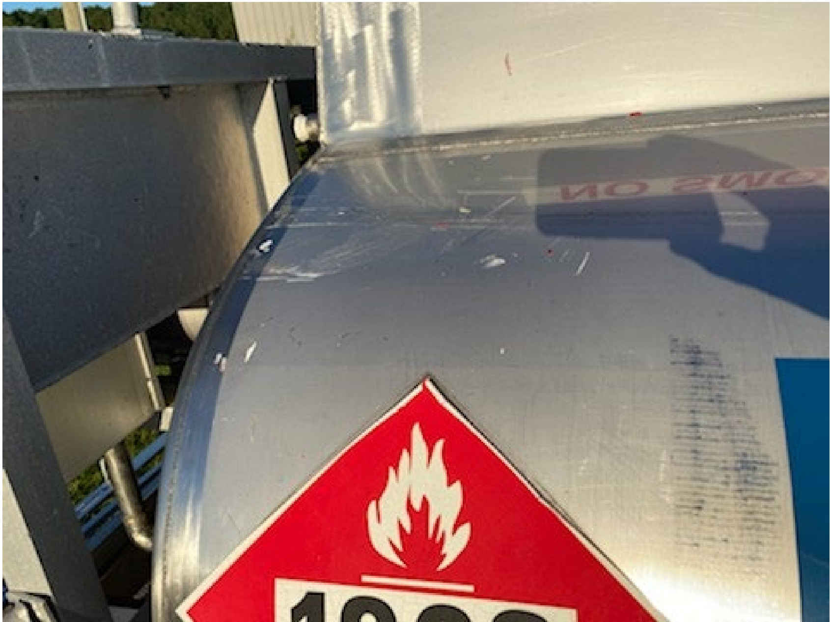
Photo 3 – Scratches and Rub Marks on Fuel Truck – Courtesy of FAA
