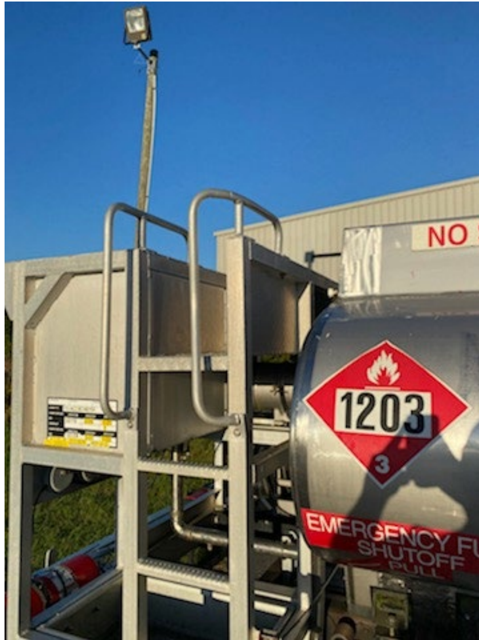
Photo 4 – Ladder Grab on Fuel Truck – Courtesy of FAA
