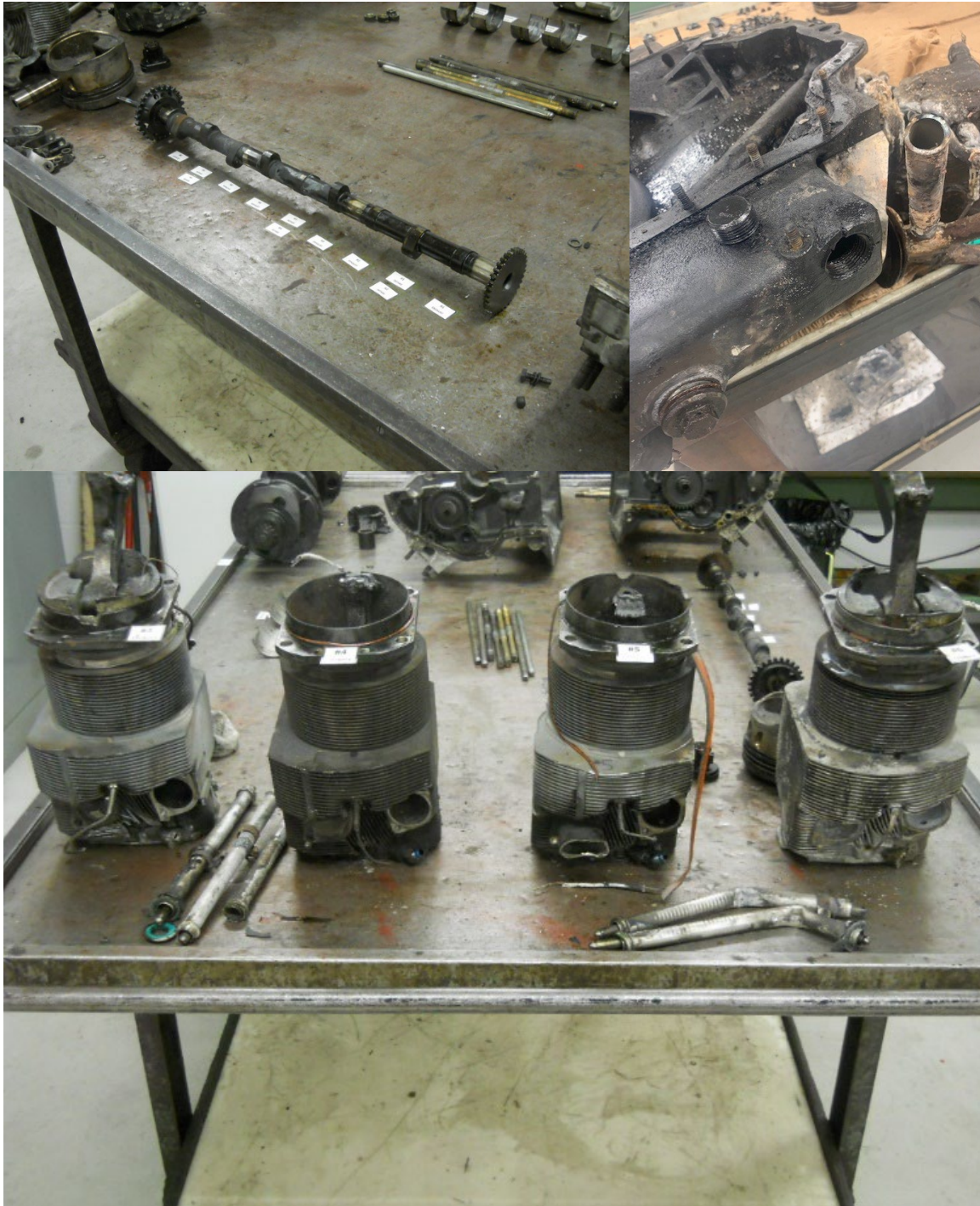
The Nos. 3 through 6 connecting rods separated from the crankshaft but remained attached to their respective piston. The No. 6 connecting rod had protruded out of the crankcase between the tappet bores. Some of the connecting rod pieces found in the oil sump were able to be identified by the
