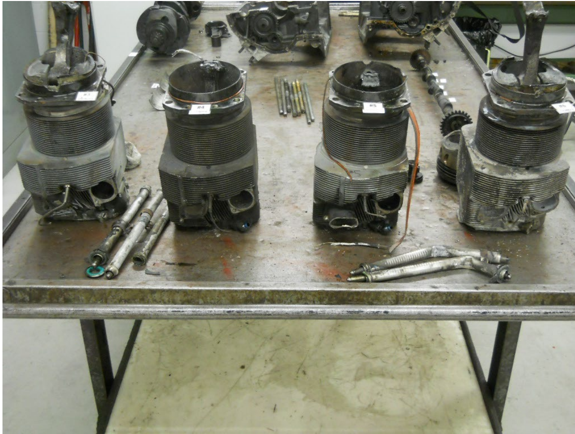
Photograph 6 - Fractured Connecting Rods
