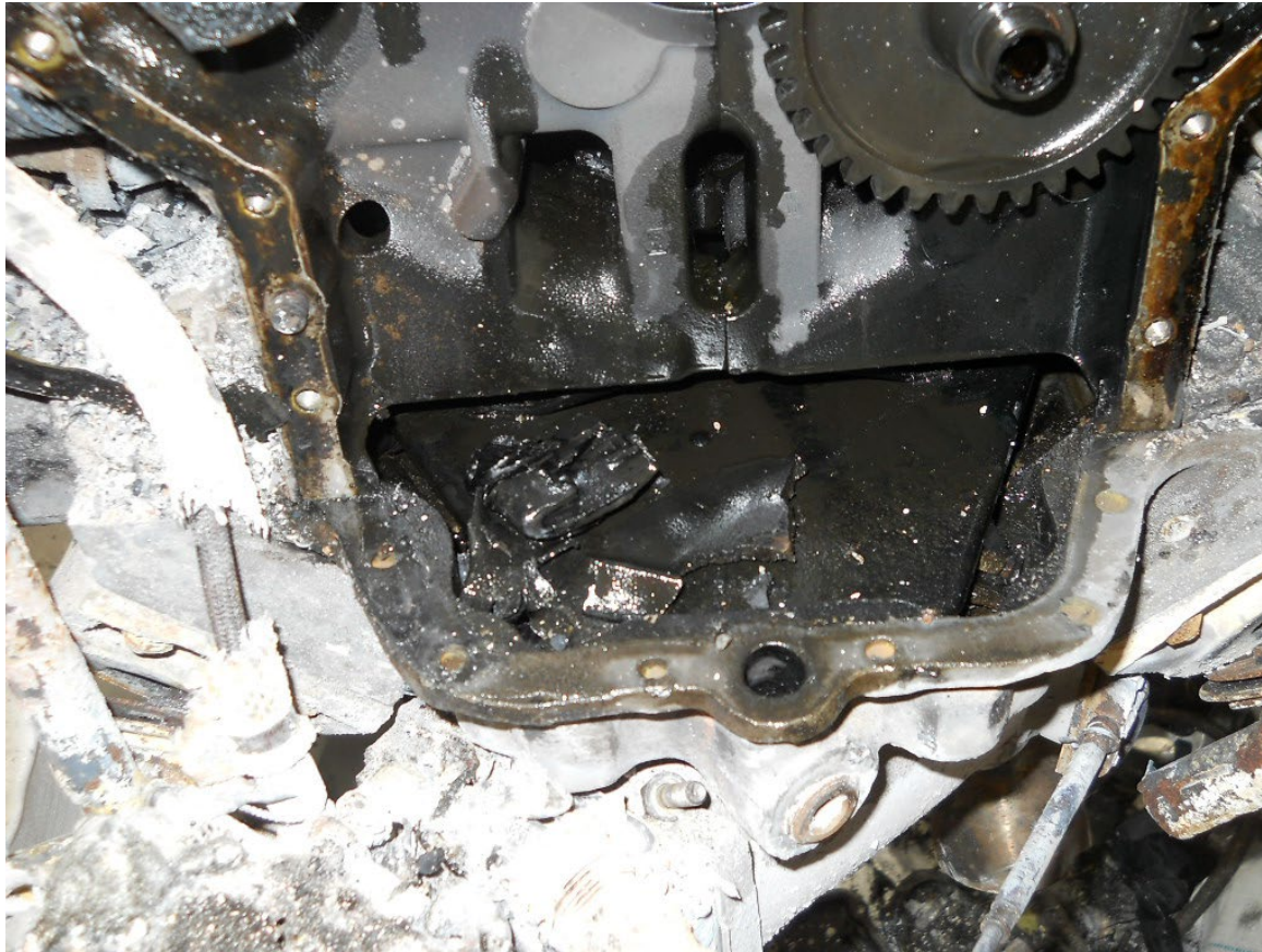
Photograph 3 - Metal Fragments in Oil Sump
