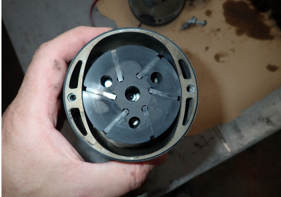
Figure 8. View of the vacuum pump.
