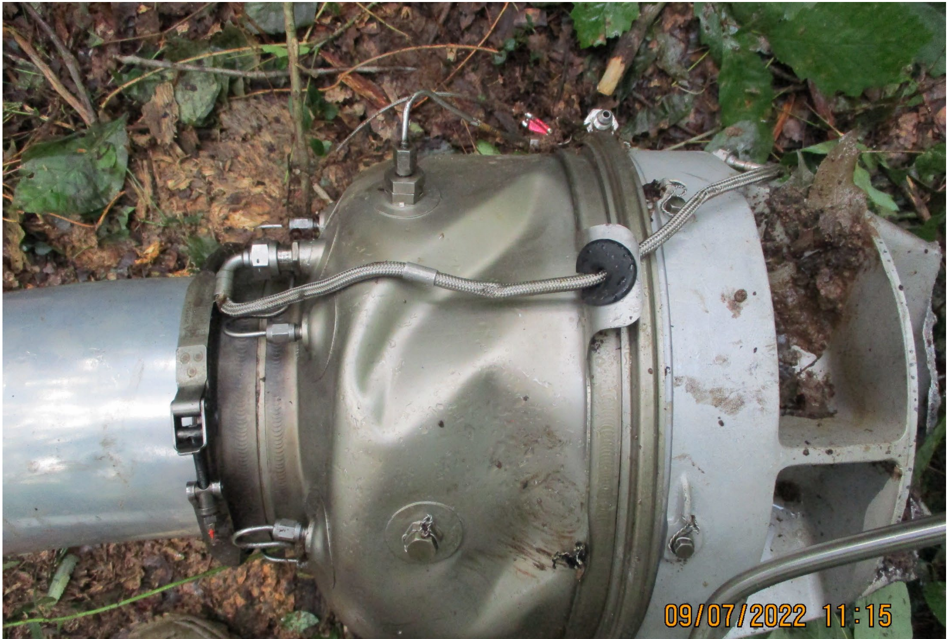
Photo 5 – engine with rotation buckling
