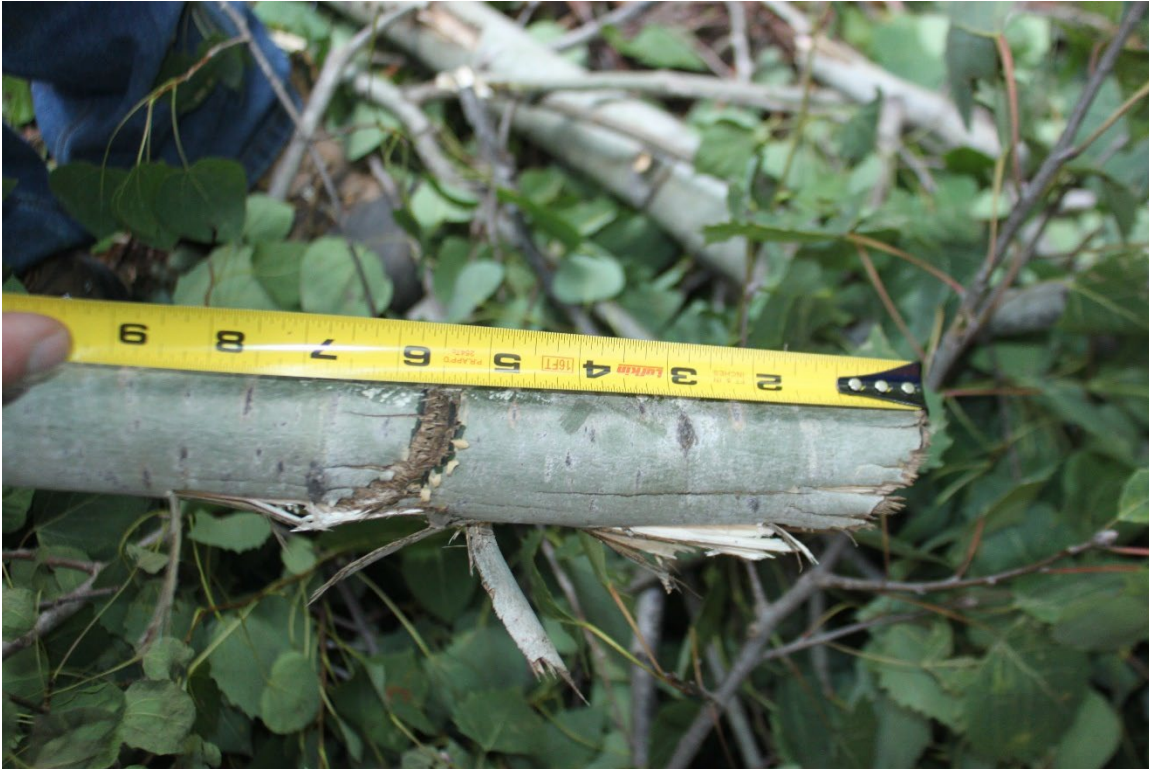
Figure 3: View of the 1.625 inches diameter tree trunk with parallel slash marks and black color consistent with propeller blade contact.
