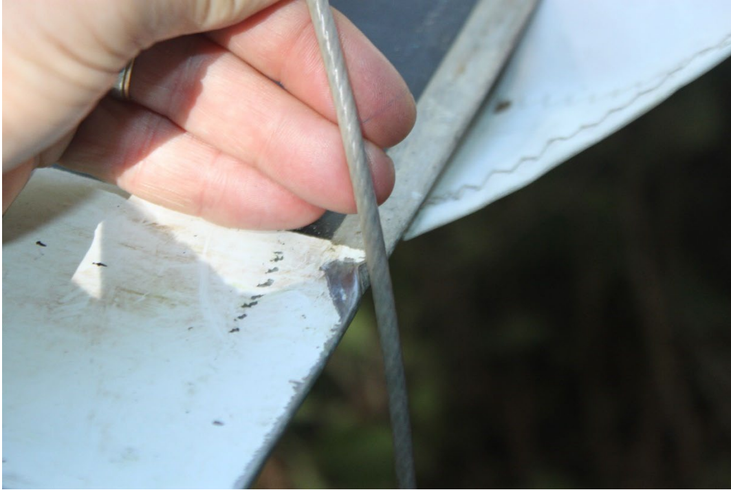
Figure 5: View Showing the Flying Wire or Control Cable from the right lower control bar attach point to the center forward attach in Proximity to the Damage on One Propeller Blade Leading Edge.
