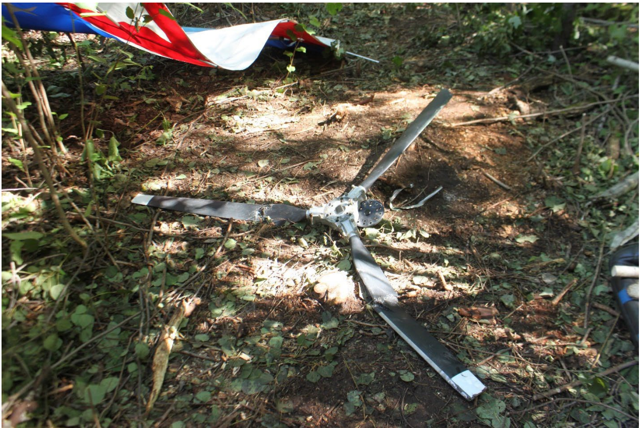
Figure 8: View of the Reconstructed Propeller.
