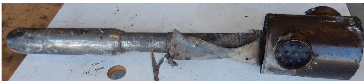
Photograph 6 –Engine left heat exchanger and tailpipe
