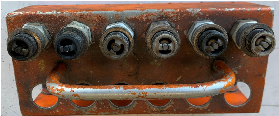
Photograph 4 –Champion REM 40 E top spark plugs removed from the accident engine.
