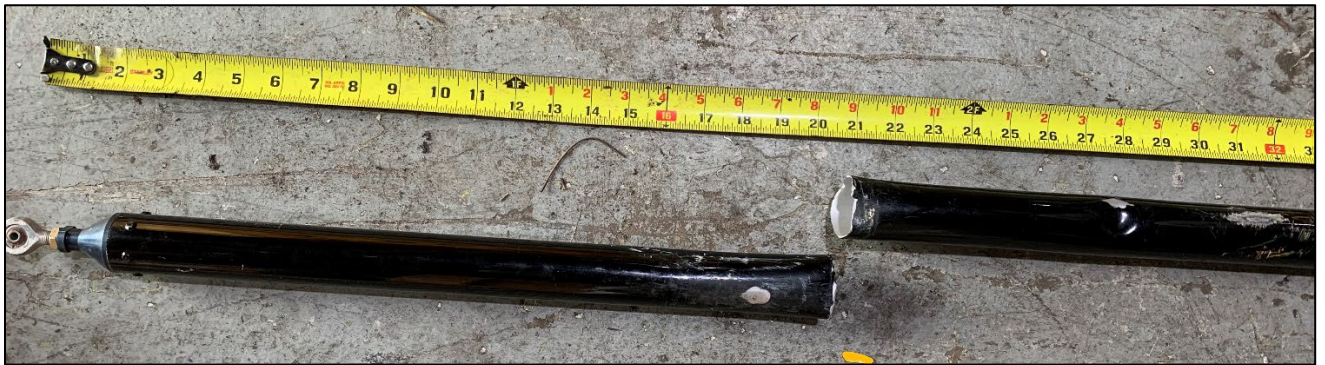
Photo 12 - View of aft elevator torque tube fracture and abrasion
