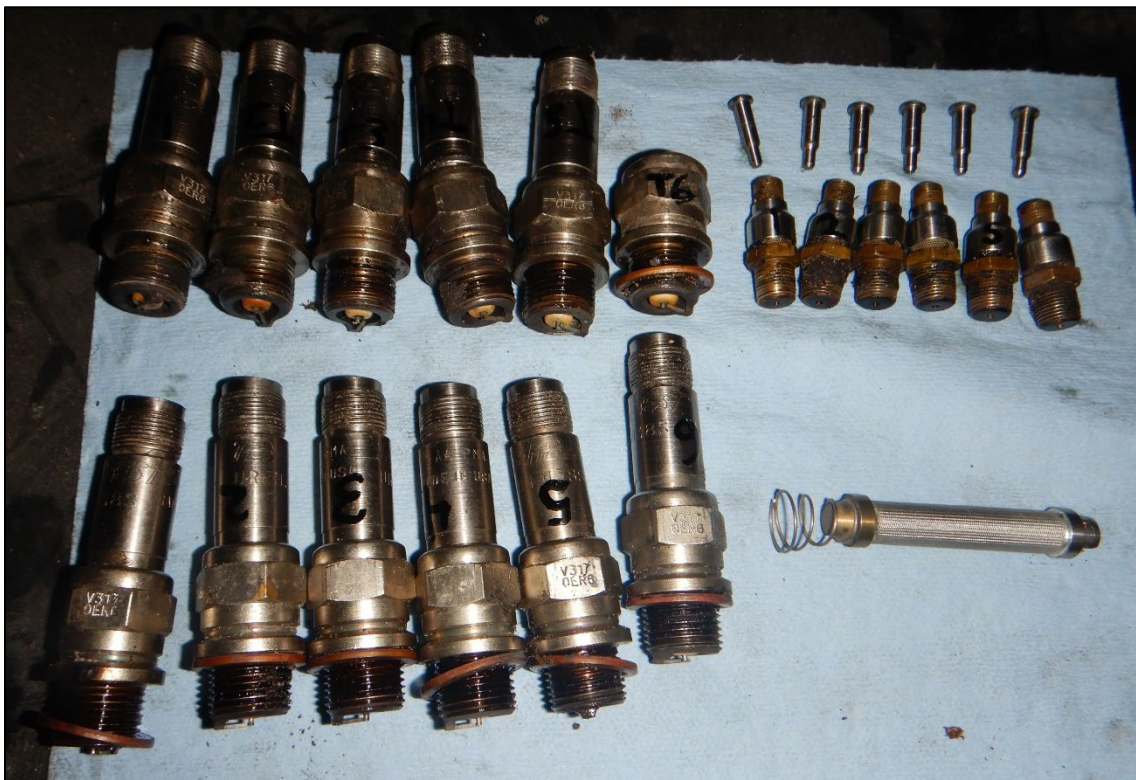
Photo 18 - Spark plugs, fuel servo inlet screen and fuel injector nozzles
