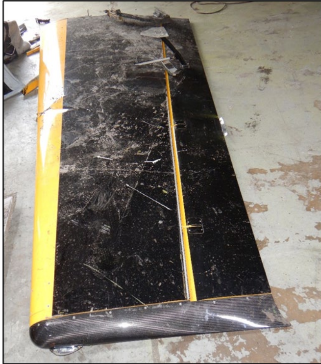
Photo 6 - Inverted right wing with aileron spade blade
