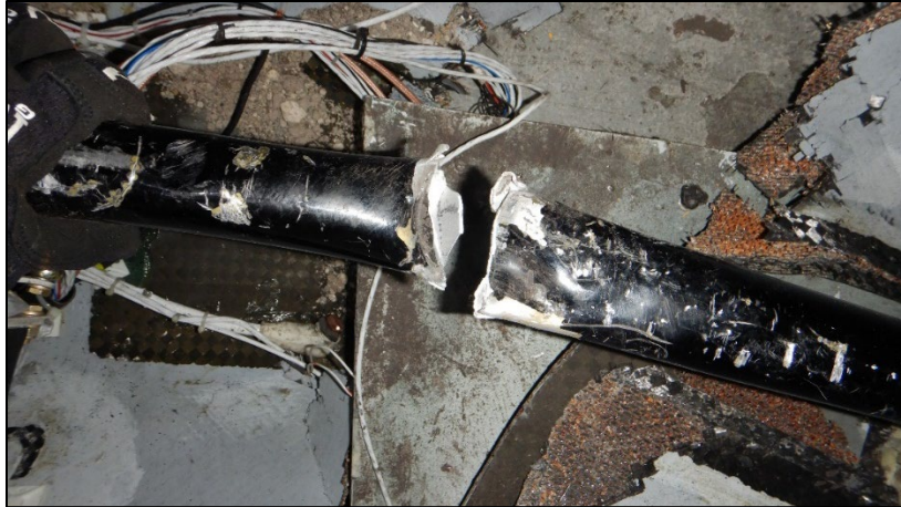
Photo 8 - Close-up photo of forward elevator torque tube fracture
