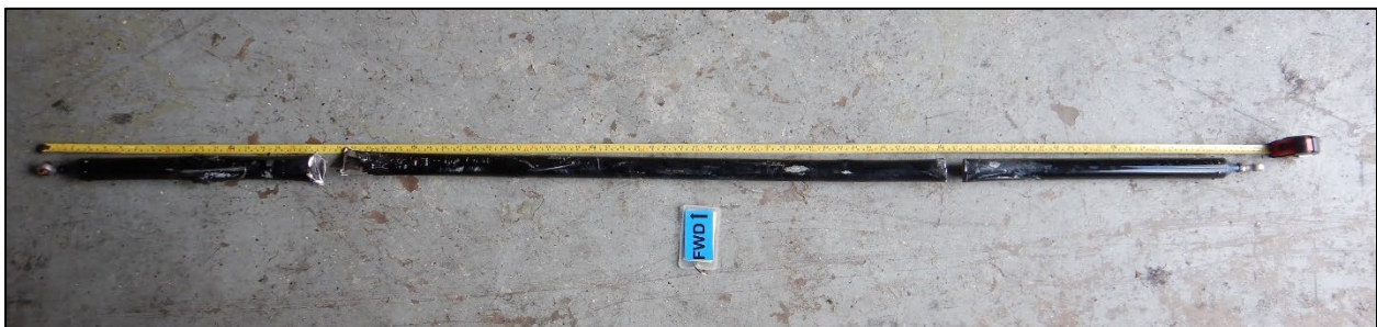
Photo 10 - Elevator control tube with fractures after removal
