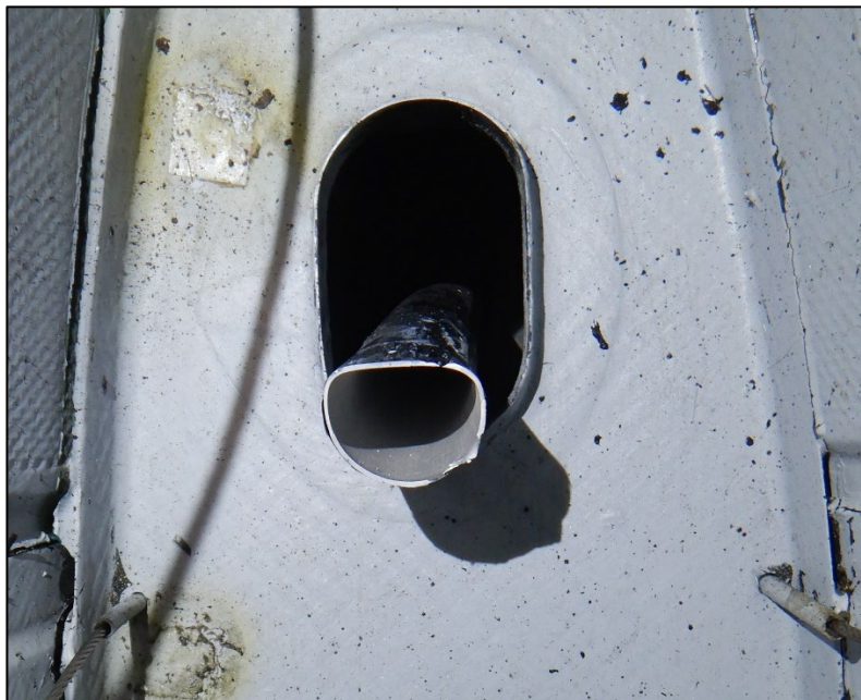
Photo 9 - Photo of aft elevator torque tube fracture at rear bulkhead
