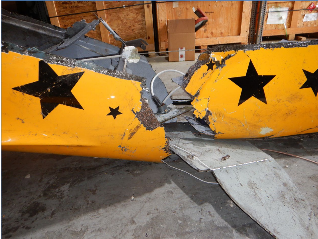
Photo 4 - Fuselage fracture aft of rear bulkhead
