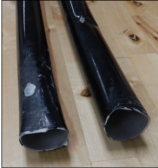
Photo 11 - Aft fracture surfaces of elevator torque tube and abrasion damage
