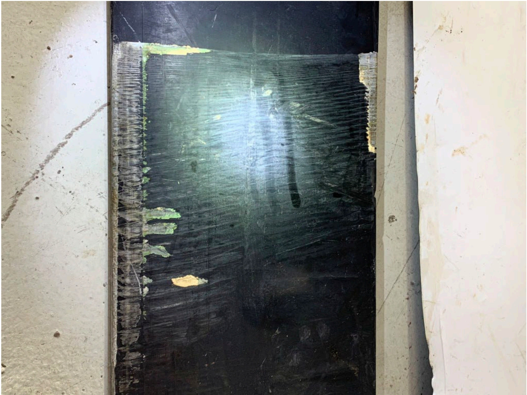
Photo 10 – Impact Marks/Striations to Bottom of White Main Rotor Blade
