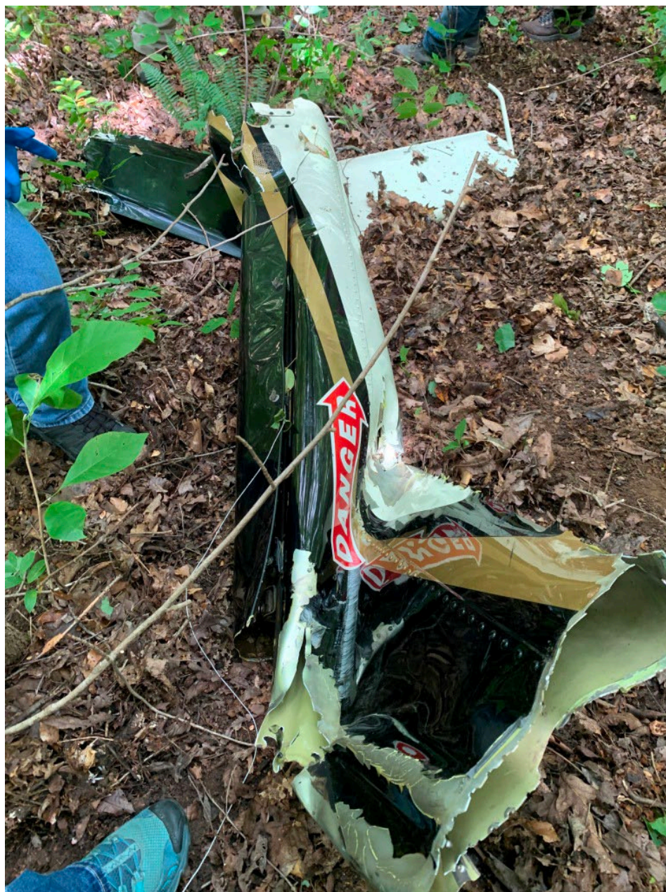
Photo 4 – Fractured Section of Tail Boom
