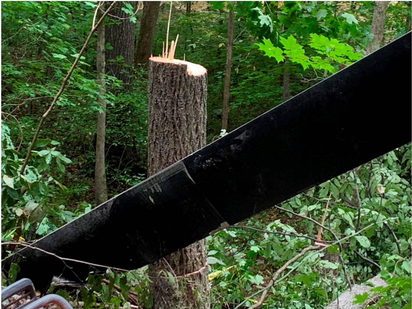
Photo 5 – Impact Striation Marks on White Main Rotor Blade
