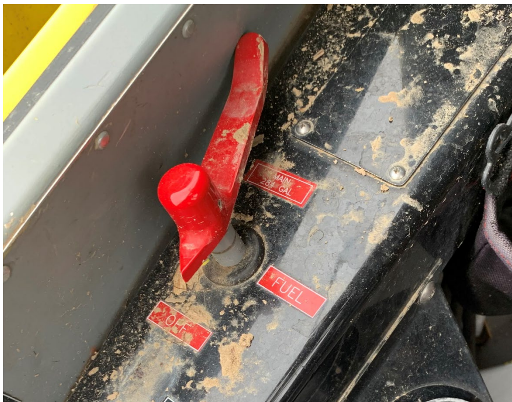
Figure 11. View of fuel selector as found.
