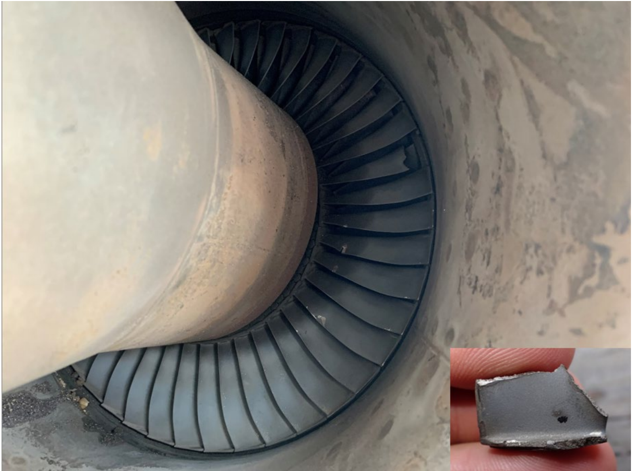
Figure 14. View of power turbine disk. Note broken blade & piece found outside the engine.
