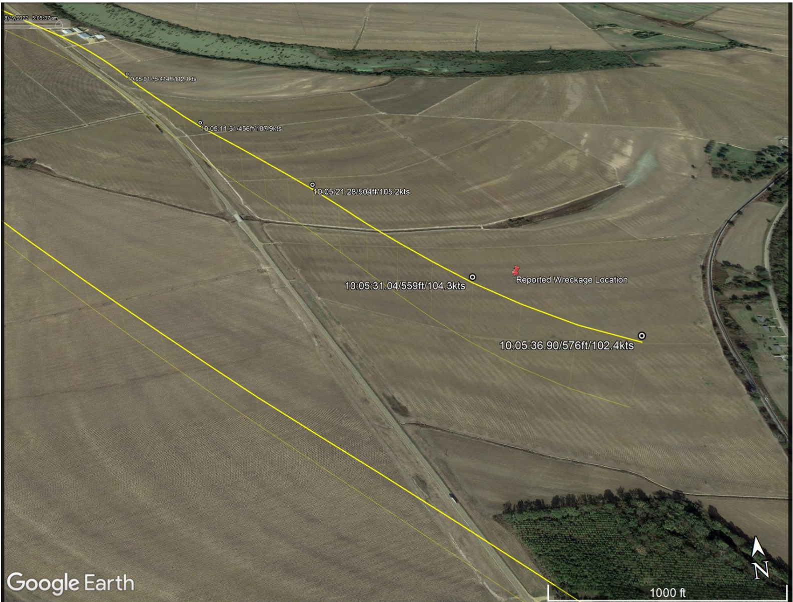
Figure 9. Google Earth overlay of the recording session from the Satloc M3 Bantam showing the final portion of the event flight.
