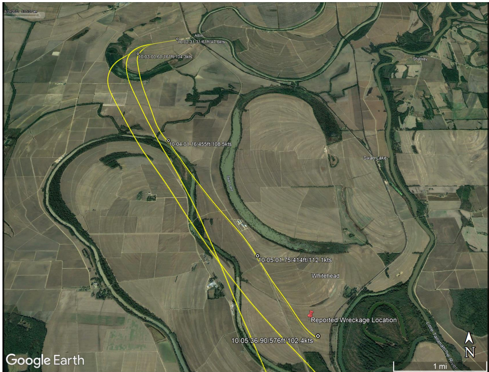
Figure 8. Google Earth overlay of the recording session from the Satloc M3 Bantam showing the event flight portion.
