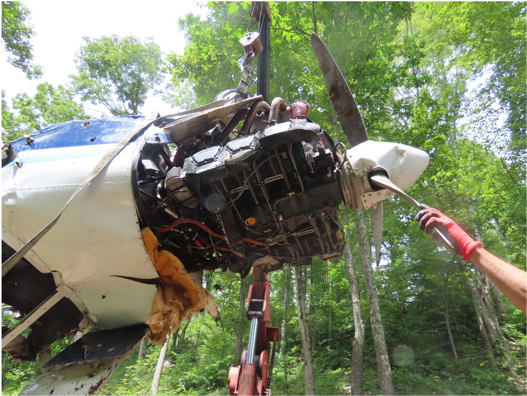
Photo 5 – View of Engine with Propeller Attached (Lycoming)
