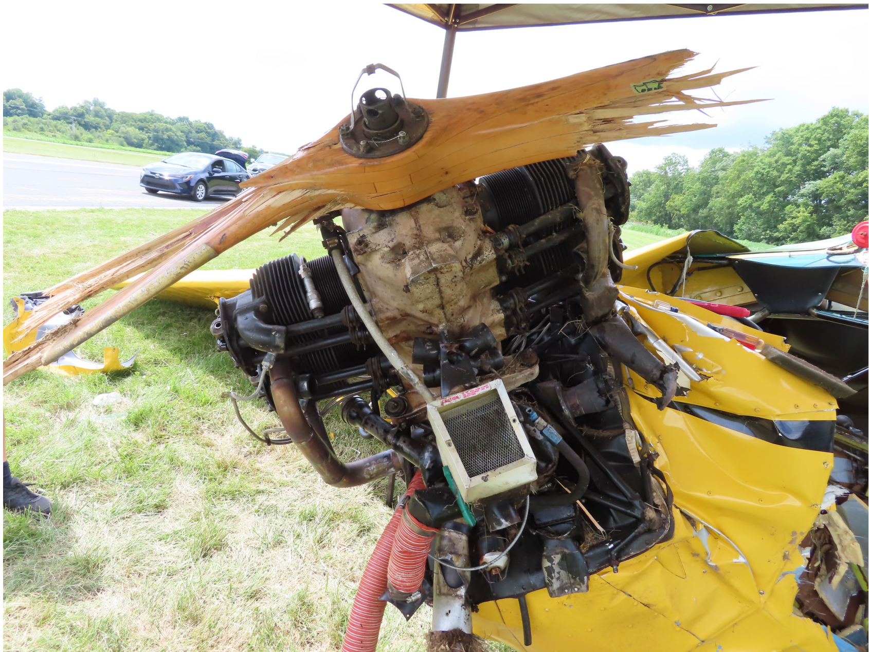
Photo 5 – Closeup of engine. Note shattered propellor and dirt on engine
