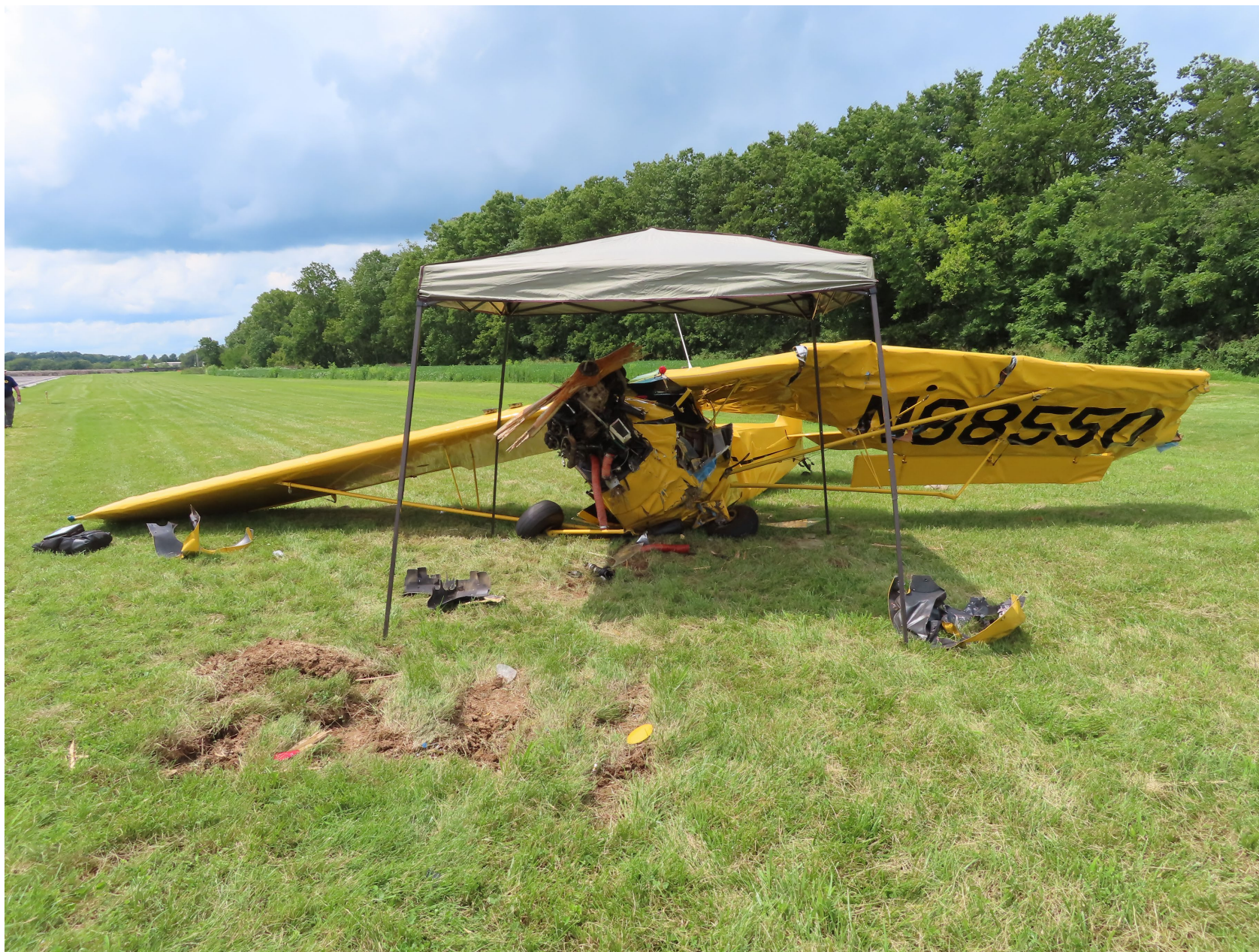
Photo 2 – Front view of aircraft. Note ground scarring
