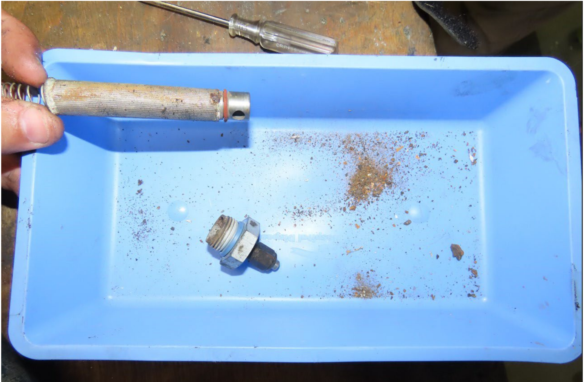
Photo 9 – View of the fuel servo screen showing contamination.
