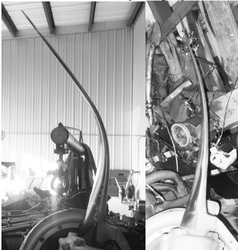
Photo #4 – Blades LA and LC after feathering showing simple aft bends with no twist
