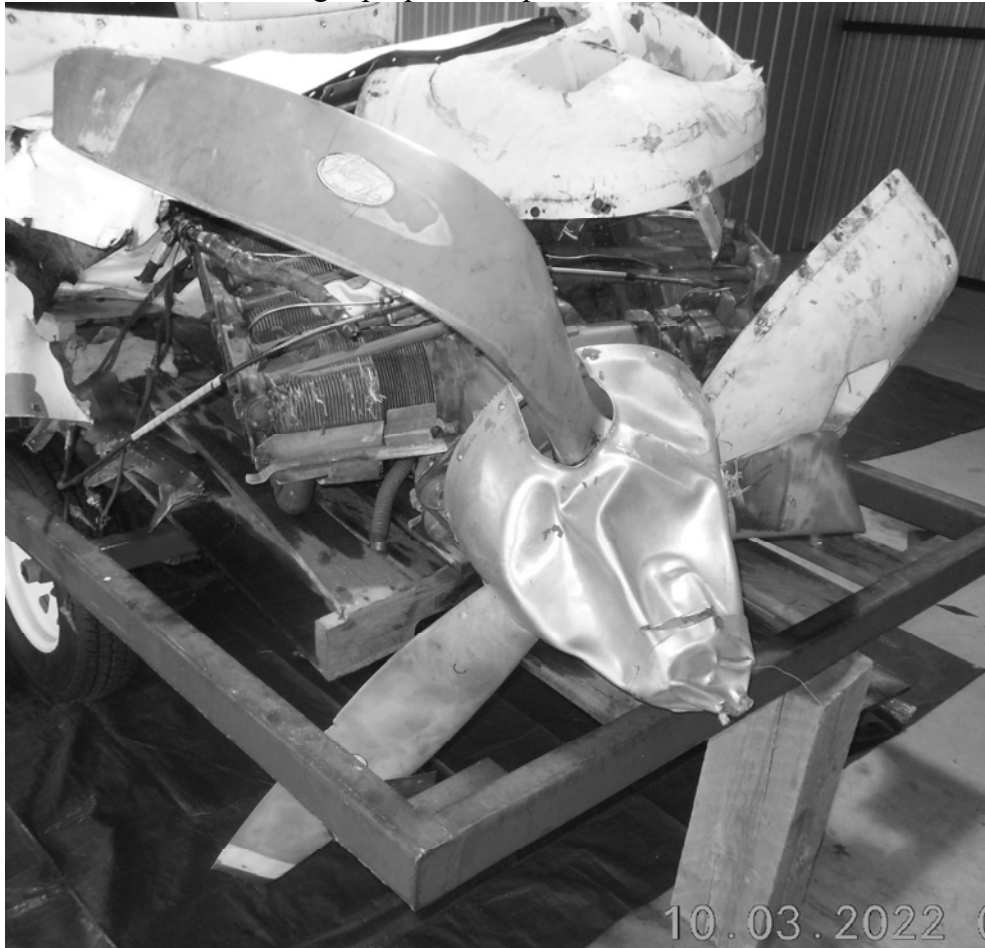
Photo #7 – Right propeller as-presented for examination
