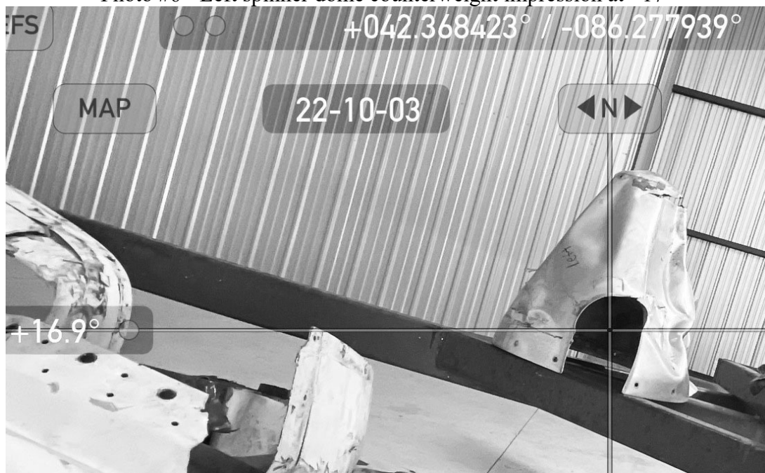
Photo #6 - Left spinner dome counterweight impression at ~17°
