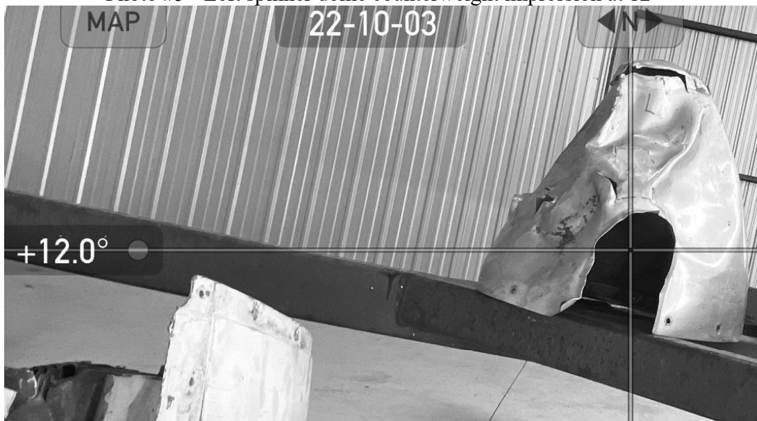
Photo #5 - Left spinner dome counterweight impression at 12°
