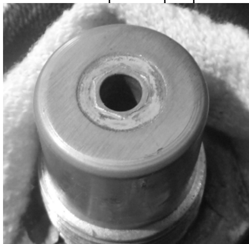
Photo #2 – Low pitch stop impact mark
