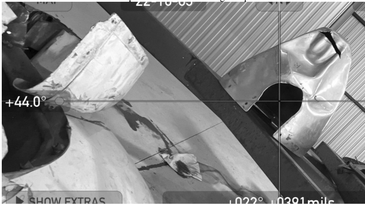
Photo #14 - Left spinner dome counterweight impression at ~44°
