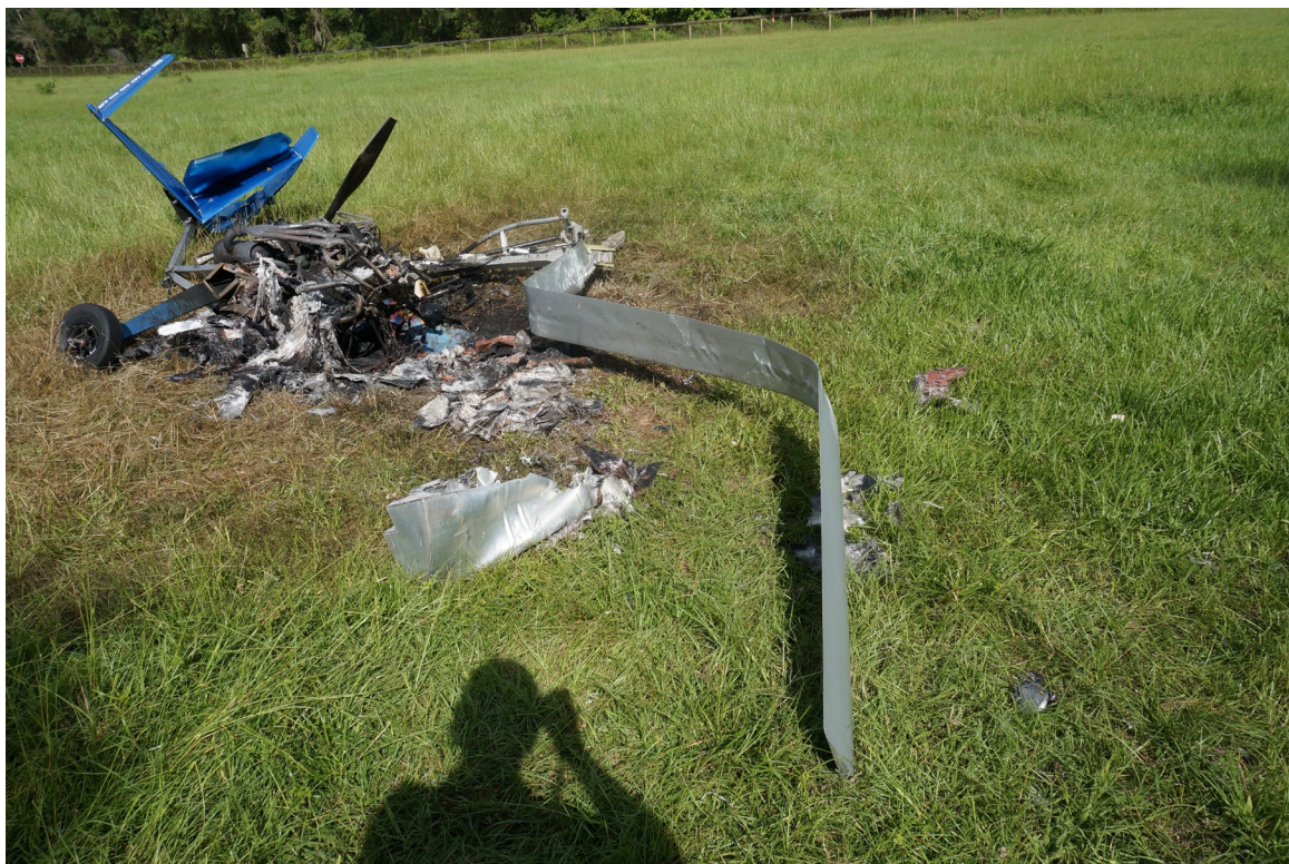
Photograph 2 - Attached Rotor Blade
