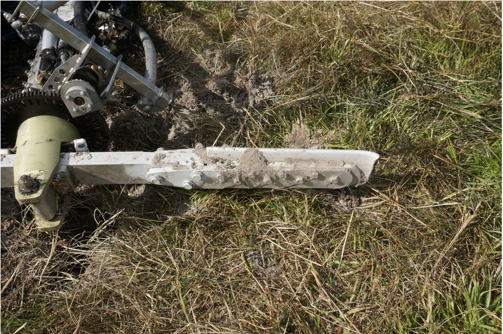
Photograph 4 - Blade Grip from Missing Rotor Blade
