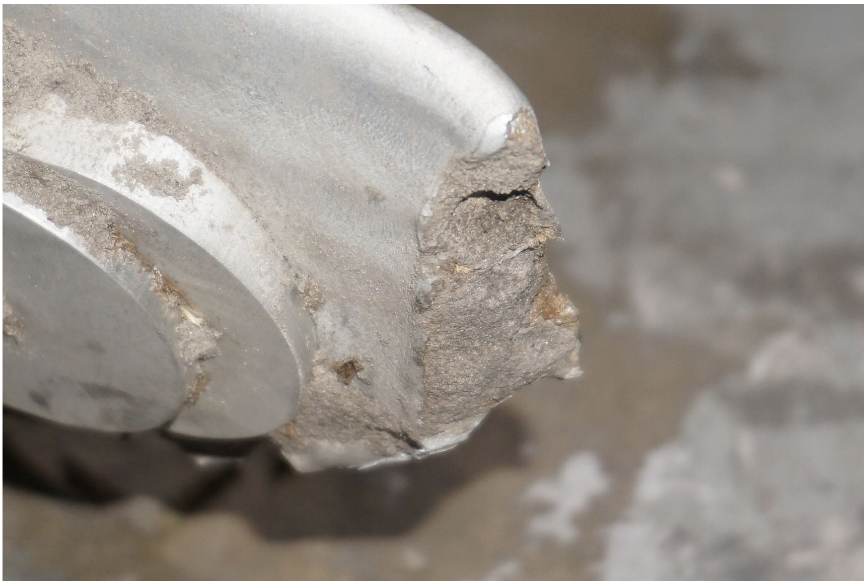
Photograph 5 - Fracture Surface Outboard of Blade Grip from Missing Rotor Blade
