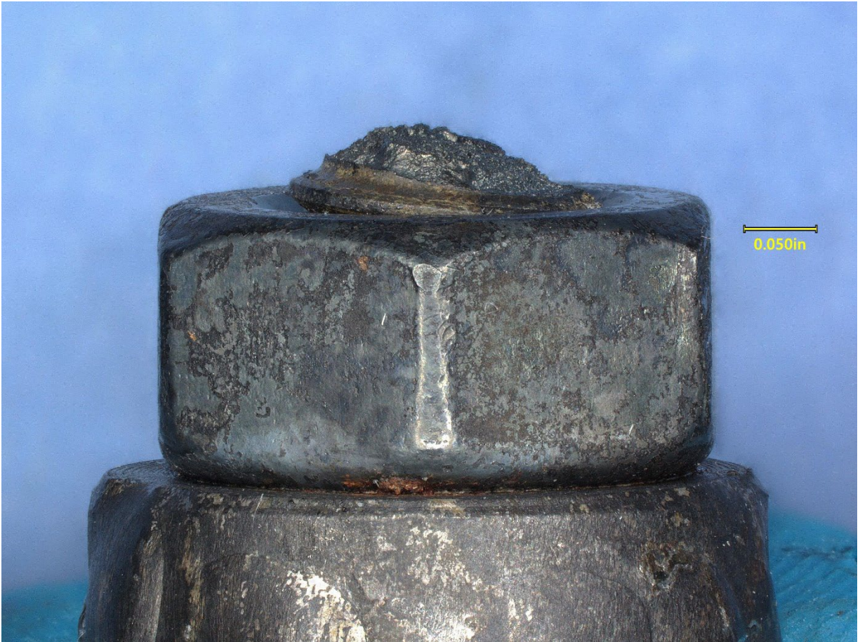
Figure 6. Rudder push pull rod end exhibiting bending of the threaded shank.
