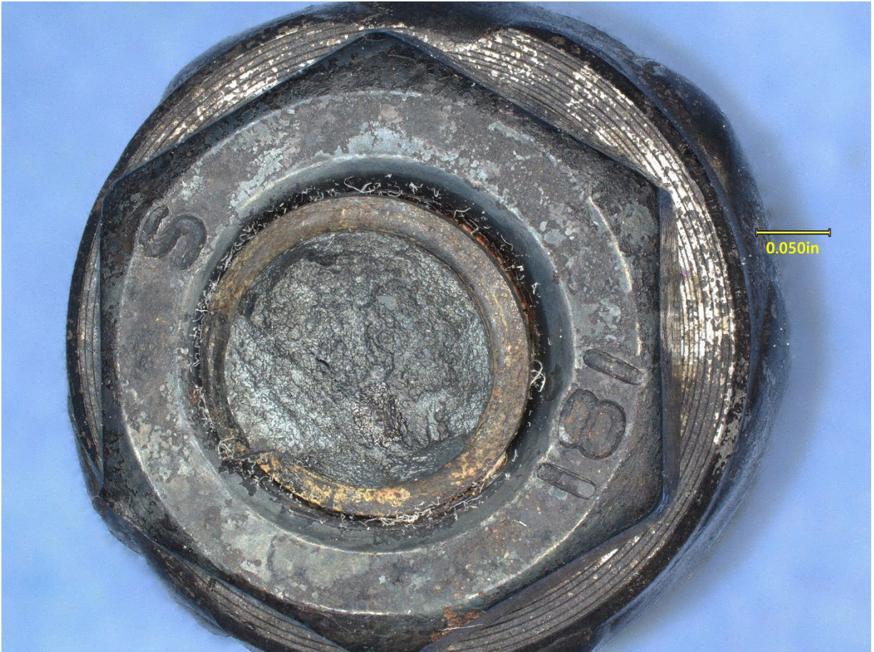
Figure 7. Slant fractures on outer periphery of the threaded shank.
