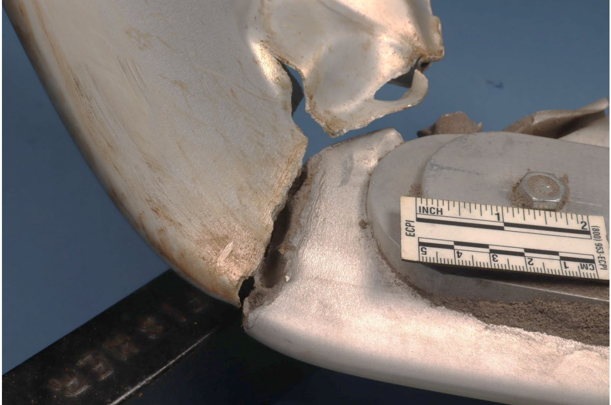
Figure 3. Close up of Rotor blade separation point.
